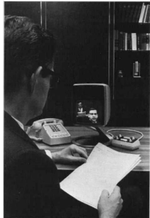
1968 The Bell System's Picturephone "see-while-you-talk" set has been redesigned to incorporate additional features as a result of the extensive trials. The improved "Mod II" set shown here is itself now the subject of further trials as the evolution of Picturephone service continues.
