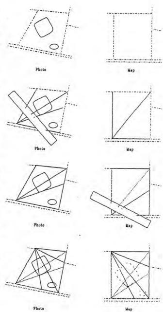
N.B. To ensure accuracy the paper strip should be laid across the lines on the photograph some distance from the control point to be used. Great care should be taken not to confuse lines - use plenty of paper strips and/or coloured pencils to ensure the right marks are transferred for each part of the construction.
