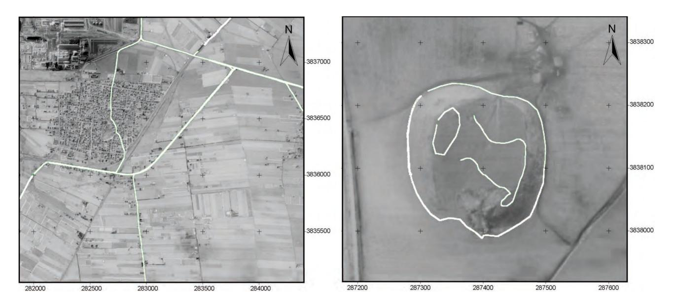
Fig 15. 2 Comparison of GPS tracks (in white) on hard and soft detail, overlaid onto Ikonos imagery
