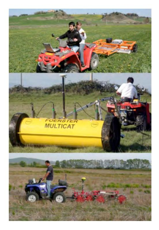
Fig 11. 10 Large-scale geophysical survey instruments in use
