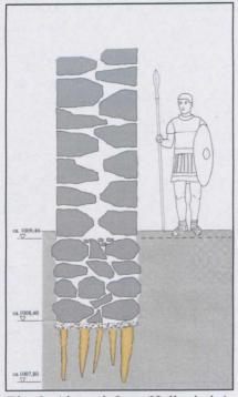
Fig. 9: Aizanoi: Late Hellenistic/ early Roman wood-pile-wall (reconstruction)
