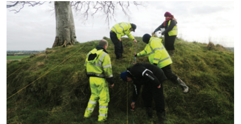
Fig. 4: 'Electrode crew' Kilberry Amenity and Heritage Group carrying out an Electrical Resistivity Tomography survey on Rathcoon Mound.
