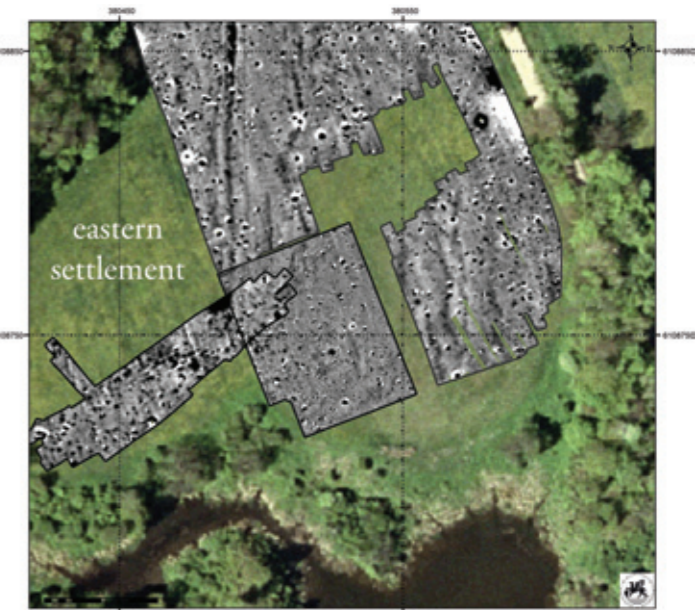
Fig. 2: Opstainis-Vilkyškiai. Geomagnetic survey; details of eastern settlement with probable semi-pit houses, storage pits; wells (5-/16-channel-magnetometer; -6/+6 nT). Graphics: S. Messal.
