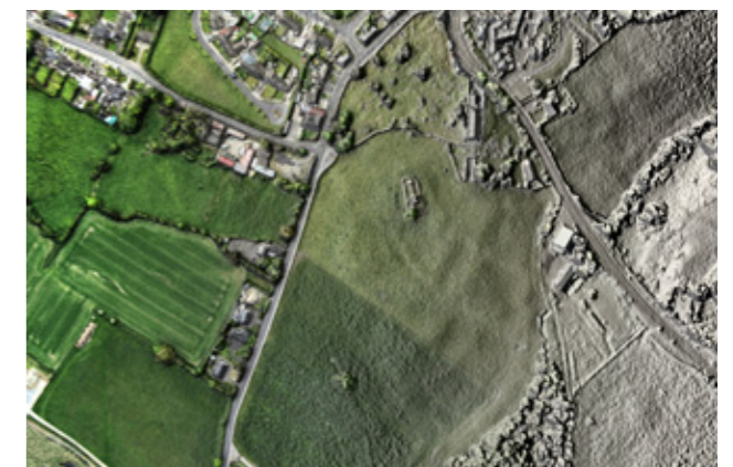
Resulting orthoimage and digital surface model produced by Simon Dowling's KAP survey (Images courtesy of Simon Dowling).
