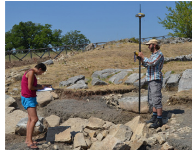
Fig. 2: Fieldschool 2012, Differential GPS survey of architectural features at the Samnite sanctuary of S. Giovanni in Galdo, Molise.
