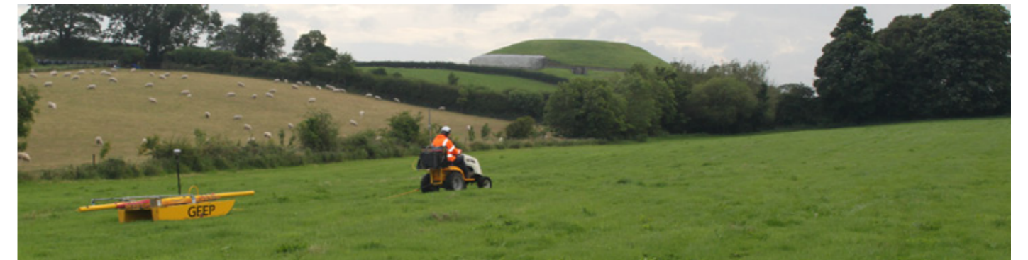
Fig. 5: Geophysical Exploration Equipment Platform (GEEP) system in operation at Newgrange, Brú na Bóinne WHS. The sled is configured with 4x caesium vapour sensors spaced 1m apart and a centrally mounted DualEM 4215 6-receiver coil EM system.
