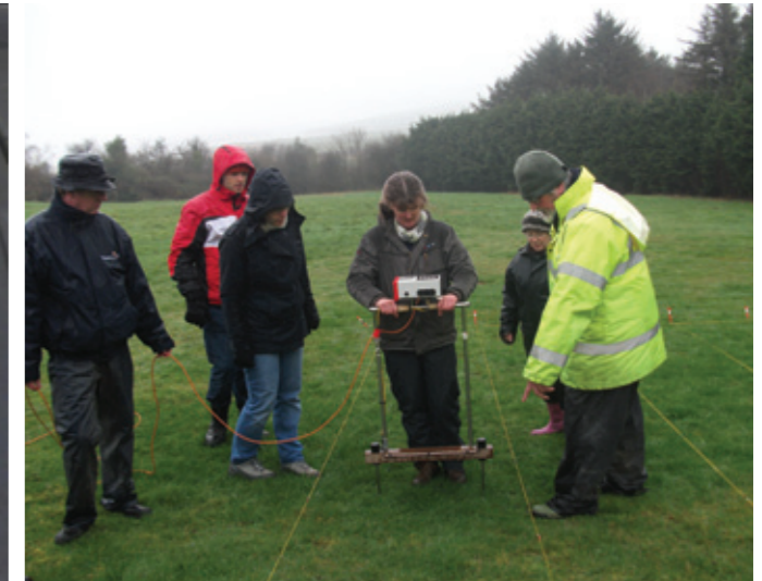
Left: TR/CIA Mark 1 Earth Resistance Meter. Right: Training session at Kilmokea Enclosure, Great Island, County Wexford, Ireland with the TR/CIA Meter mounted on a 0.5m frame and configured as a twin-probe array. (Kevin Barton/JohnFlynn).
