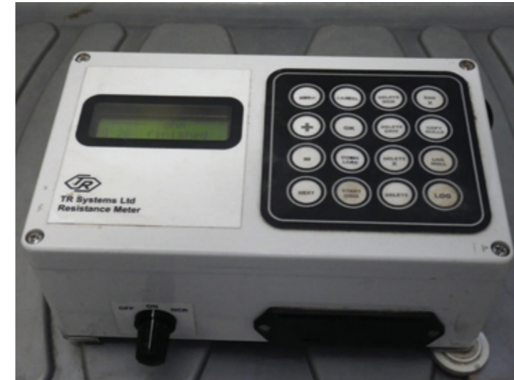
Left: TR/CIA Mark 1 Earth Resistance Meter. Right: Training session at Kilmokea Enclosure, Great Island, County Wexford, Ireland with the TR/CIA Meter mounted on a 0.5m frame and configured as a twin-probe array. (Kevin Barton/JohnFlynn).
