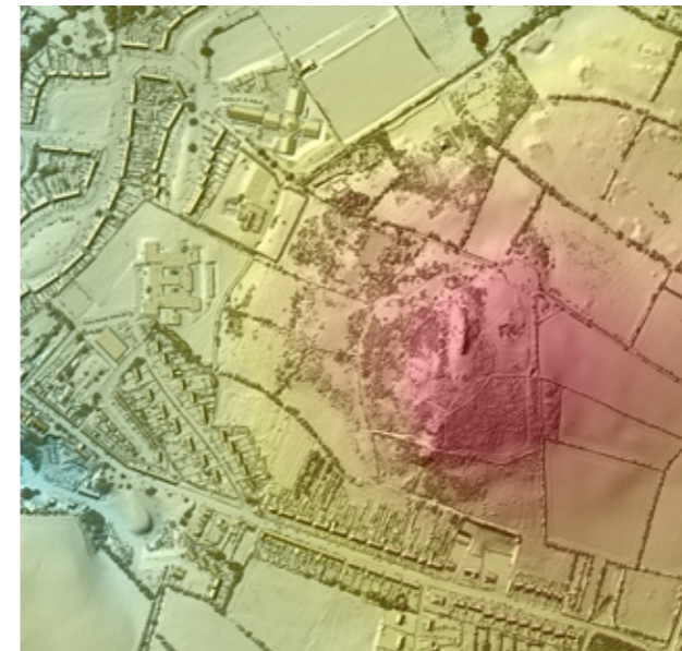
Shaded relief digital surface model of the summit of Vinegar Hill derived from National Road Authority (NRA) LiDAR survey.
