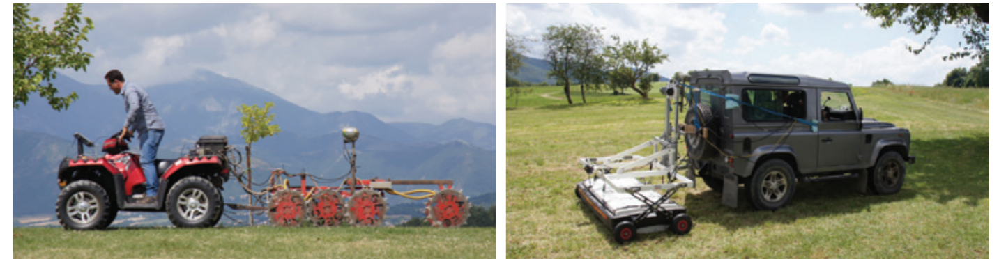
Fig. 3: Extensive geophysical mapping. ARP System (in collaboration with Geocarta, Paris and So.Ing, Livorno) and IDS Stream X (in collaboration with IDS Corporation, Pisa and Geostudi Astier, Livorno) in action on the field during the school.
