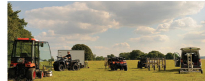
Fig. 2: Motorized LBI ArchPro fluxgate magnetometer systems and 16-channel 400 MHz MALÅ Imaging Radar Array (MIRA) in operation at Stonehenge (LBI ArchPro, Geert Verhoeven).
