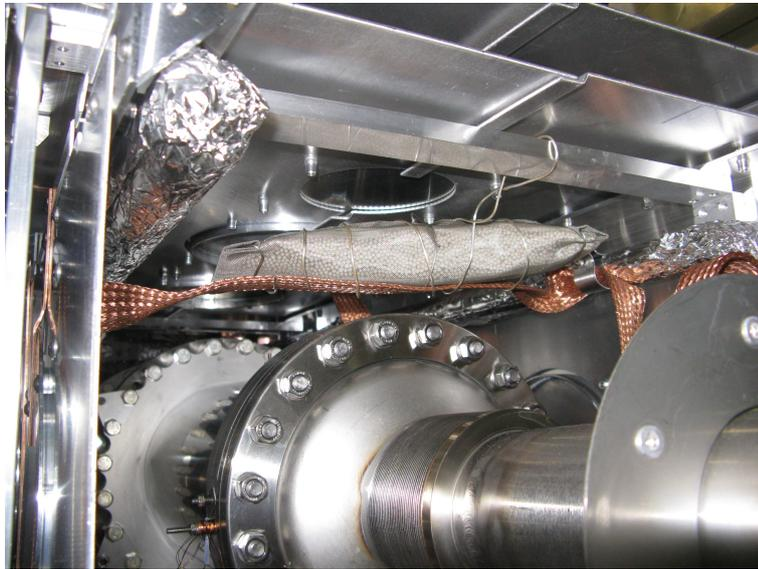
Figure 3.14: Photo of one of the molecular sieves mounted in the isolation vacuum. It is resting on one of the 40 K copper thermal shield cooling lines, suspended above the ion gauge chamber. A mounted silicon diode sensor can be seen in the lower left corner of the picture, in addition to part of the 80 K shield surrounding the 40 K thermal shields.
