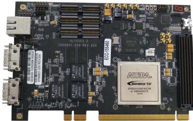
Figure 2. Stratix IV HTX3 Board
