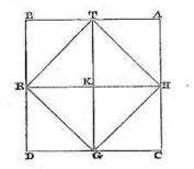
Quadrangles are of five kinds: firstly, with right angles and equal sides; secondly, with right angles and unequal sides; thirdly, the rhombus, with equal sides and unequal angles; fourthly, the rhomboid, the length of which differs from its breadth, and the angles of which are unequal, only that the two long and the two short sides are respectively of equal length; fifthly, quadrangles with unequal sides and angles.
