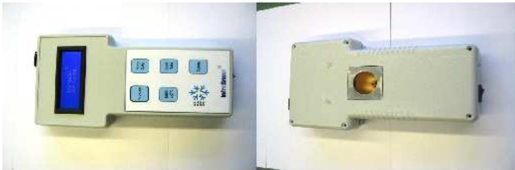
**Figure 4.2:** Top and bottom view of the operational InfraSnow device. For measurements the InfraSnow is placed on the snow surface. The maximum lateral extensions are 23 cm x 13 cm. The top view reveals the user interface of LCD display and push buttons. On the bottom side the golden integrating sphere, illustrated in Figure 4.1, can be seen through the opening inside an aluminum frame.
