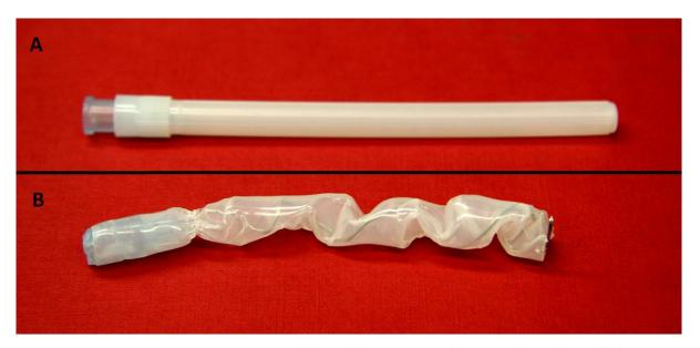
Figure 109: Effect of pressure on a needle including its cover. The picture shows the needle before (A) and after (B) the exposure to 90 MPa along the longitudinal axis.
