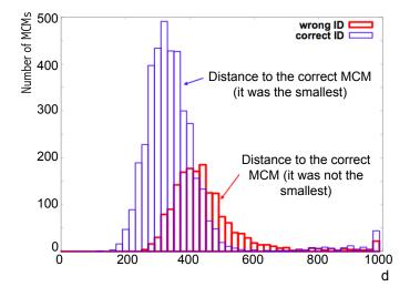
Figure 3.16: Distribution of the squared distance *d*. Blue histogram: correctly identified MCMs (the reference pattern with smaller distance from our measurement belongs to the same MCM). Red histogram: distance of our measurement from the correct reference pattern, although it is not the smallest (the MCM is wrongly identified). The pedestal correction is not applied in this measurement. Reference from [51].
