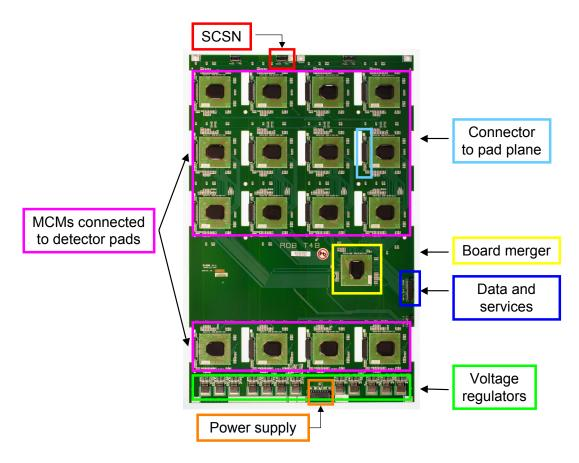
Figure 3.5: A TRD ROB integrating 17 MCMs. The functionalities of the different MCMs are indicated, as well as the main elements implemented on the board.
