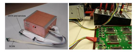
Figure 3.7: Box containing the single-MCM external PCB (left) and connection of the power supply lines to the ROB (right).
