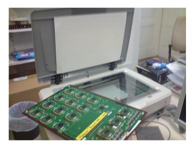
**Figure 3.17:** EPSON GT 200000 scanner used to take picture of the ROB for the identification of the MCMs.
