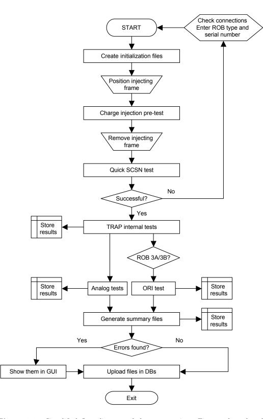
Figure 3.9: Simplified flow diagram of the test routine. Figure adapted and updated from [121].
