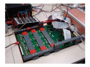
Figure 3.11: Frame used to inject signals at the PASA input positioned on a ROB.
