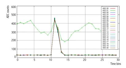
Figure 3.13: Output of the analog test for an MCM with baseline shift in 1 channel.
