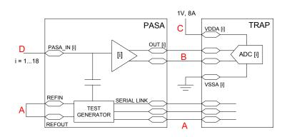
Figure 3.10: Schematic view of the PASA/TRAP interface and critical points. A: reference voltage of the PASA internal test-pattern generator and its serial link to the TRAP chip. B: interface between PASA and TRAP. C: ADCs' reference voltage. D: PASA input connected to the detector.
