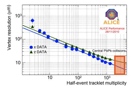
Figure 2.7: Primary vertex resolution in PbPb collisions at  $\sqrt{s} = 2.76$  ATeV as a function of half of the ITS tracklet-multiplicity in the event. The resolution along the x and z coordinates is obtained dividing the tracks of the event in two random samples and reconstructing two vertices for the two samples. The difference between these two vertices is the measure of the resolution as a function of the half tracklet-multiplicity. Fit according to Eq. 2.4. More details in the text.
