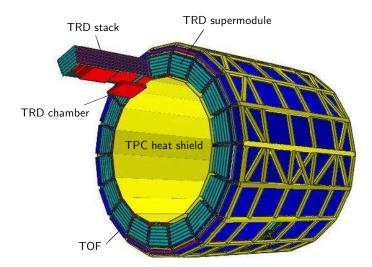
Figure 3.1: Schematic representation of the TRD system layout. Shown are 18 supermodules, containing 30 read-out chambers each (red) and arranged in 6 radial layers. Figure from [15].
