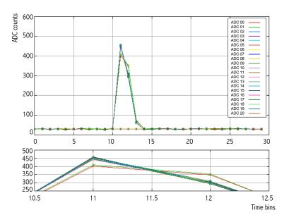
Figure 3.14: Output of the analog test for an MCM with phase shift in 2 channels.
