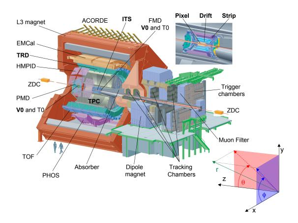
Figure 2.2: Schematic representation of the ALICE detector. Top-right insertion: enlargement of the Inner Tracking System (ITS) showing its sub-systems. Bottomright insertion: ALICE carthesian and spherical coordinate systems. The z > 0region is the so called detector A-side and the z < 0 region is the C-side.
