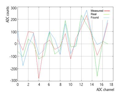
Figure 3.15: Baseline pattern for one TRAP ADC: the average baseline value is plotted as a function of the channel number. Reference from [51].
