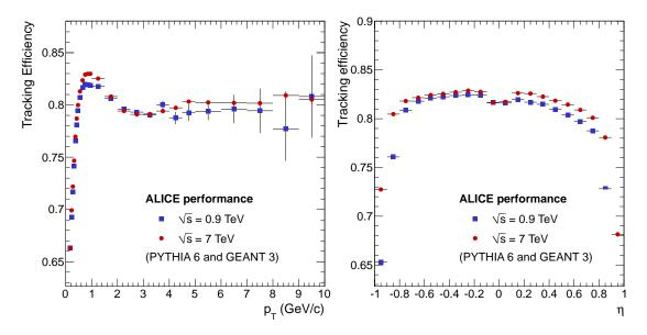
Figure 5.20: Tracking efficiency as a function of track  $p_{\rm T}$  (left,  $|\eta| < 0.8$ ) and  $\eta$  (right,  $p_{\rm T} > 0.5 \,{\rm GeV}/c$ ). The decrease in the range 1–3  ${\rm GeV}/c$  is due to straight (high- $p_T$ ) tracks falling in the dead areas between TPC sectors. The dip at  $\eta = 0$  in the pseudo-rapidity projection is due to the central TPC cathode. PYTHIA and GEANT simulation.
