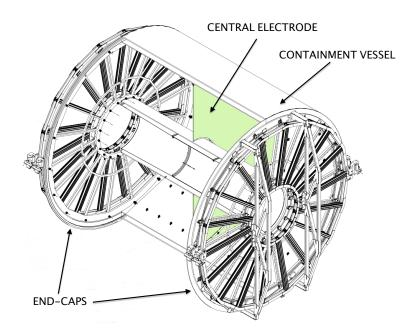
**Figure 2.3:** 3D view of the TPC field cage. The containment vessel and the central electrode are indicated in the figure, as well as the end-caps sustaining the read-out chambers (not shown). Figure adapted from [15].
