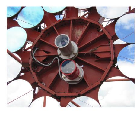
Figure 4.2.: The picture shows the LidCCD in the central part of the CT2 dish and the SingleCCD in the bottom right part.
