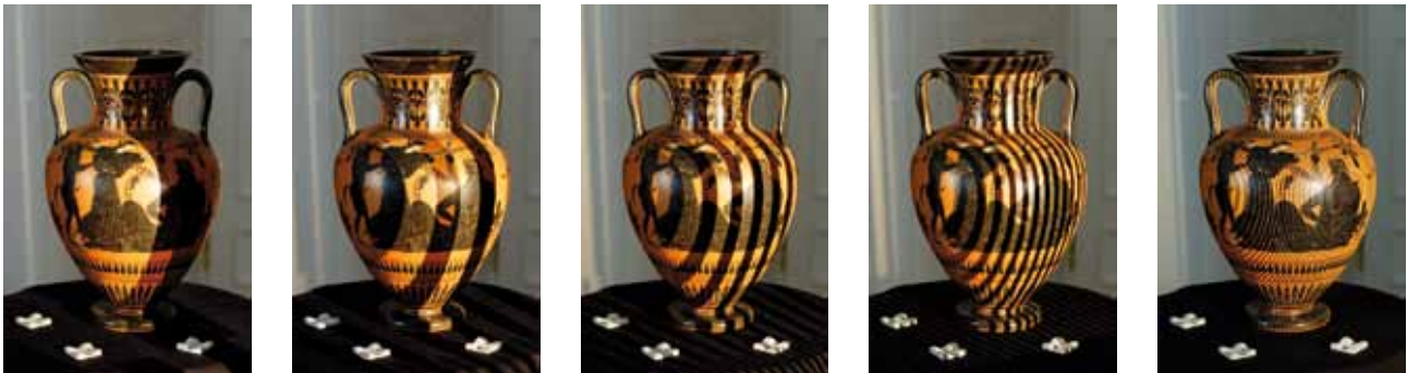
Figure 3: Setup of the 3D scanner and the turntable for the acquisition of KHM ANSA IV 3601. The image on the top shows a Breuckmann smartSCAN-3D-HE using the optics with a FOV of 470 mm. The lower images show the structured light patterns projected on the object during the acquisition.
