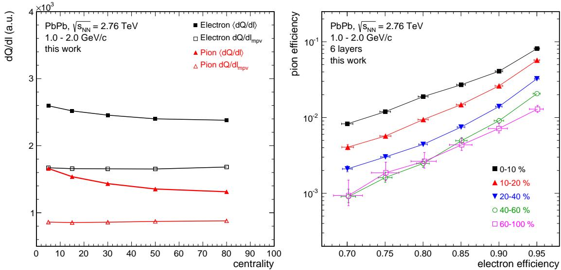
Figure 6.22: (left) Centrality dependence of mean  $\langle dQ/dl \rangle$  and most probable  $dQ/dl_{mpv}$  charge deposit. (right) Pion efficiency as a function of the electron efficiency in different centrality bins.
