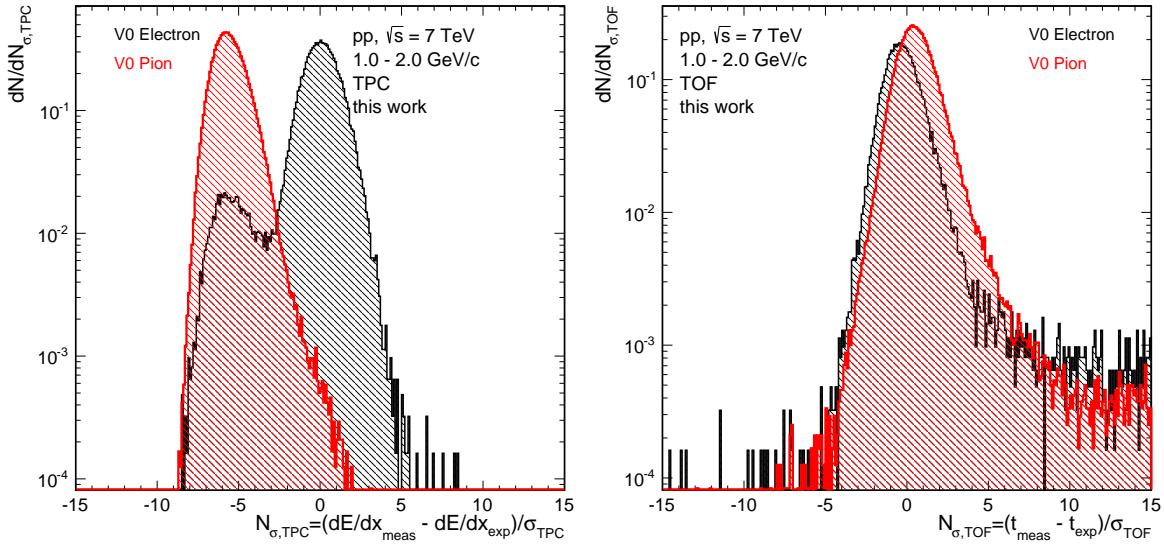
Figure 6.13: (left)  $N_{\sigma, \text{TPC}}^e$  and (right)  $N_{\sigma, \text{TOF}}^e$  for V0 identified electrons and pions at  $1 - 2 \text{ GeV}/c$ .
