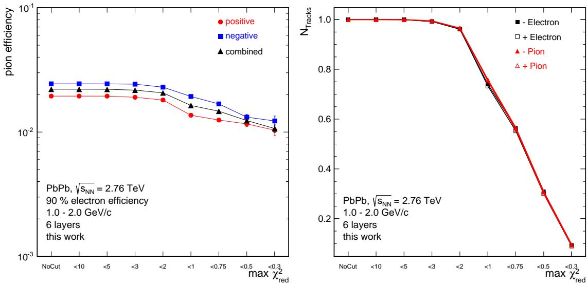
Figure 6.19: (left) Pion efficiency as a function of the  $\chi^2_{\text{red}}$ -cut for positively and negatively charged tracks and combined. (right) Corresponding number of tracks surviving the  $\chi^2_{\text{red}}$ -cut.
