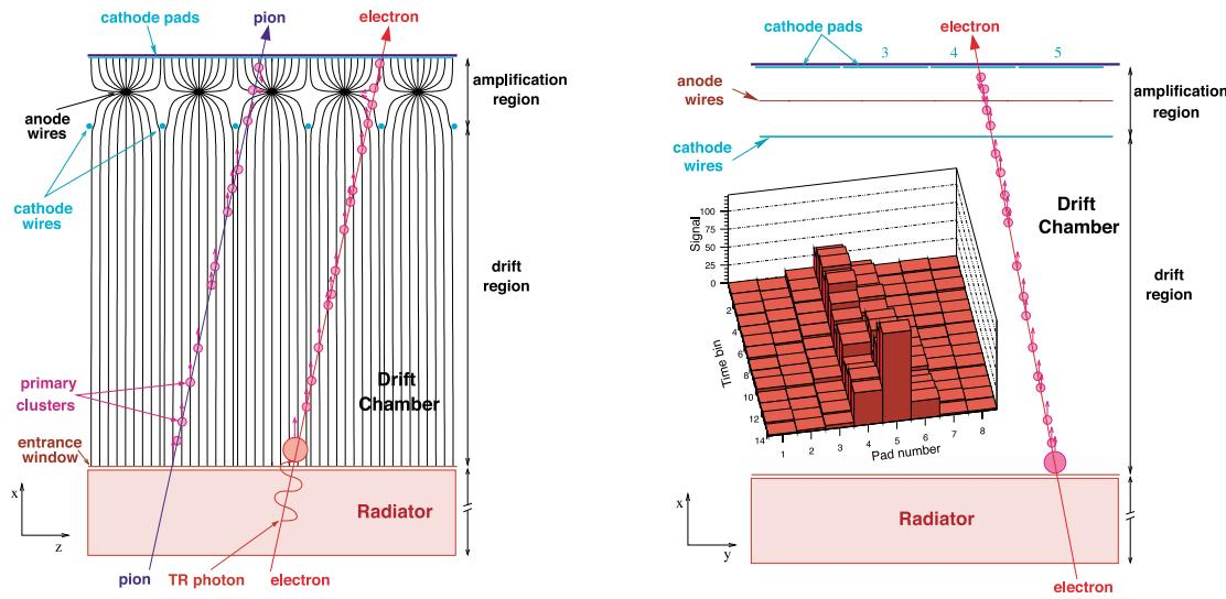
*Figure 6.3:* Cross section of a TRD readout chamber and schematic illustration of the principle of operation. (left) Projection in  $xz$  plane. Schematic signals produced by the energy loss of a pion and an electron. (right) Projection in the  $xy$  plane. The insert shows the distribution of the pulse height (signal) over pads and time bins [268].
