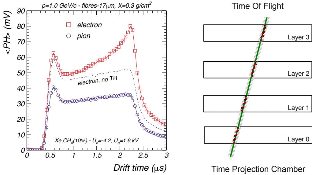
Figure 6.4: (left) Average pulse height as function of the drift time for pions and electrons with a momentum of  $1\text{ GeV}/c$  [268]. (right) Illustration of the TRD track reconstruction.
