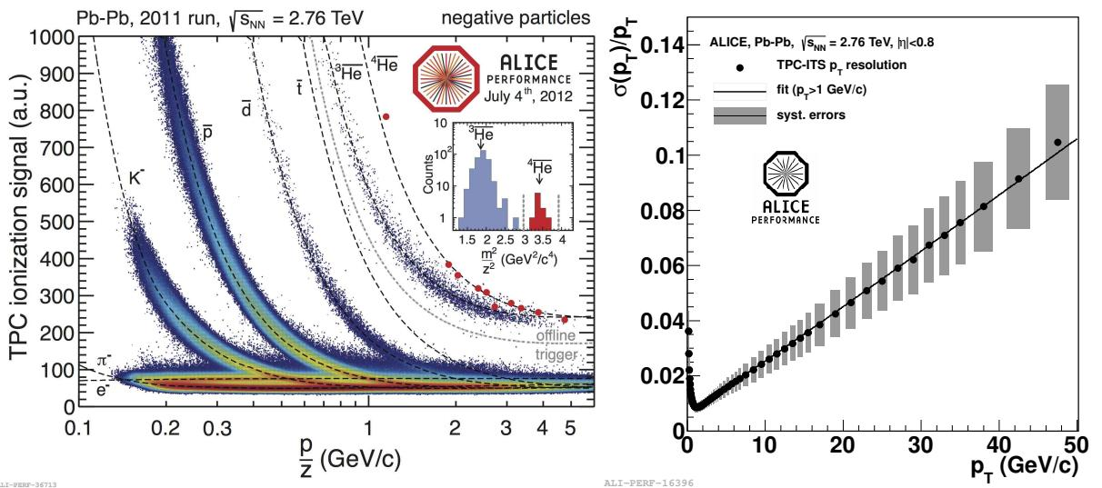
Figure 5.3: (left) TPC signal as a function of the momentum over charge ratio  $p/Z$  [234]. (right) Relative  $p_T$  resolution for TPC-ITS combined tracks as a function of  $p_T$  [239].
