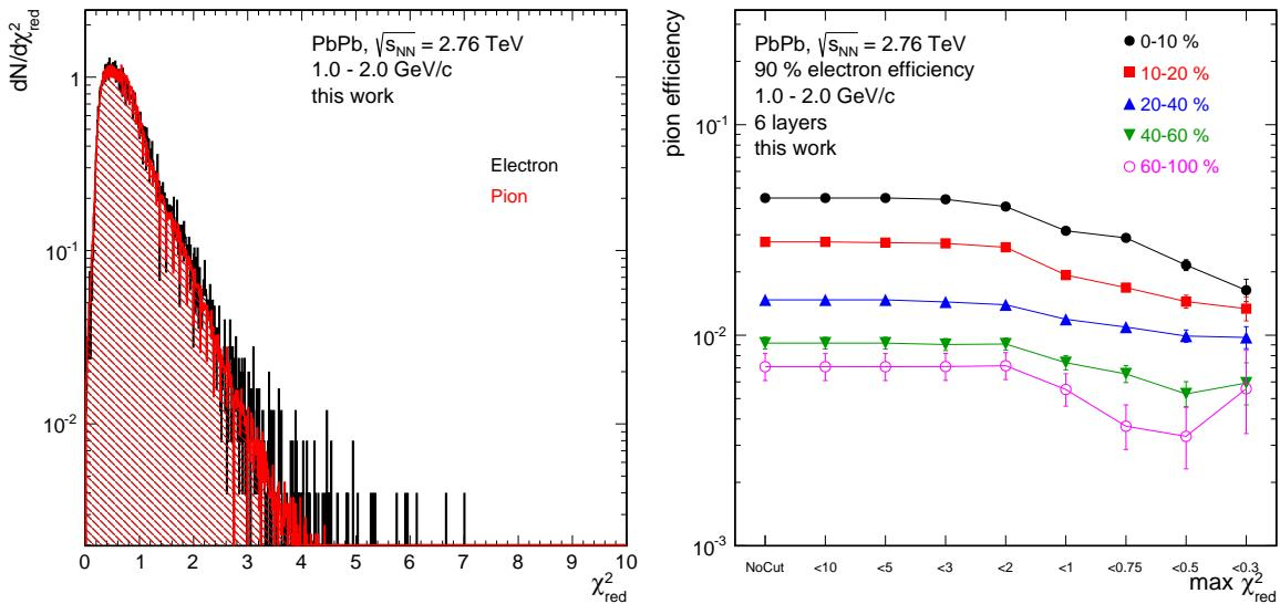
Figure 6.18: (left)  $\chi^2_{\text{red}}$  distribution for pions and electrons. (right) Pion Efficiency as a function of a cut on  $\chi^2_{\text{red}}$  for various centralities.
