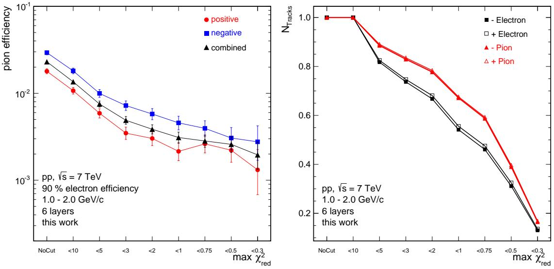
Figure 6.17: (left) Pion Efficiency as a function of a cut on  $\chi^2_{\text{red}}$ . (right) Corresponding number of tracks surviving the  $\chi^2_{\text{red}}$ -cut.
