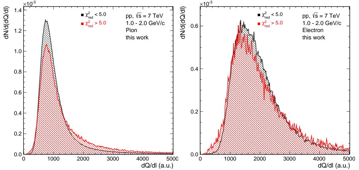
Figure 6.16:  $dQ/dl$  distribution for pions (left) and electrons (right) for tracks above and below a  $\chi^2_{\text{red}}$ -cut at  $\chi^2_{\text{red}} = 5$ .
