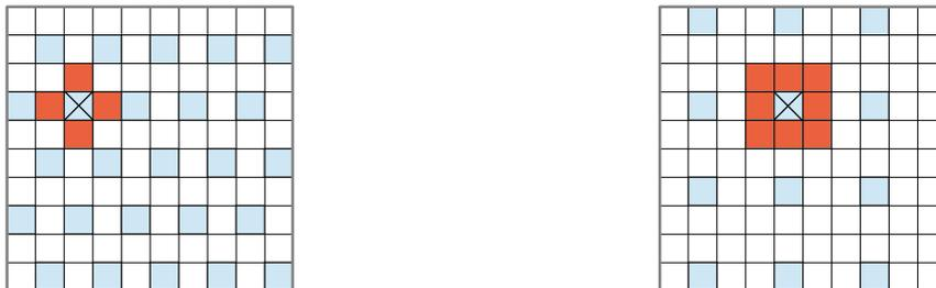
Figure 6.3: Schematic illustration of the distribution of pixels operated in Timepix mode (blue squares) and energy mode (white squares) over the detector area. The graph on the left shows the distribution for measurements in which one out of four pixels was operated in Timepix mode, while in the graph on the right one out of nine pixels is operated in Timepix mode. The red squares indicate the pixels used for derivation of the pseudo energy value of the pixel marked with a black cross.
