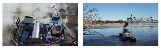
Figure 35. Setup for water analysis and air collection (left) and PTFE chamber on Lake Dune in 2013 (right). Images: Torsten Krause CC BY-SA 4.0.
