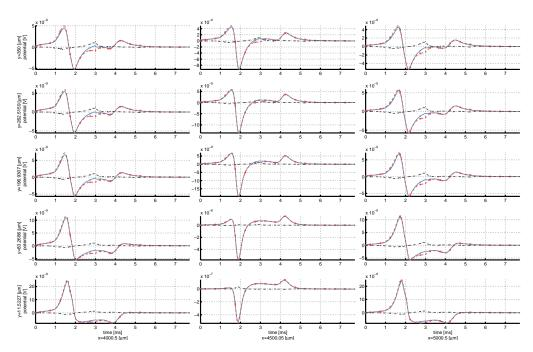
Figure 6.15: Comparison with LSA at various farfield positions. The same potential time courses as in fig. 6.14 (solid lines) are compared with the LSA potential (dashed lines). Additionally, the difference between both curves is shown (dash-dotted lines). The agreement between both models generally is very good and shows notable deviations only between peaks N1 and P3.
