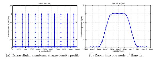
Figure 6.8: **Equilibrium charge density profile**. The scaled charge densities  $\sum_i z_i n_i$  at equilibrium follow a distinct, comb-shaped distribution along the membrane (*left*). On the right, a zoom into one node of Ranvier reveals the jump in equilibrium concentrations due to different membrane permittivities at myelin and nodes of Ranvier.
