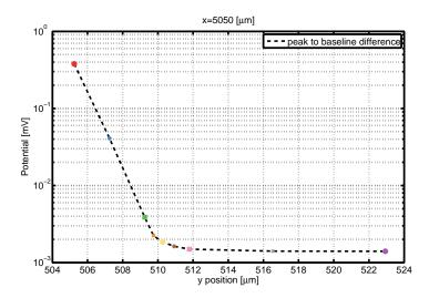
Figure 5.14: **Decay of peak-to-baseline in EAP over Debye layer**. For the EAPs in fig. 5.12, the difference between peak and baseline potential (value at  $t = 2 \,\mathrm{ms}$ ) is plotted on a log-scale, showing an abrupt switch in the fall-off rate.
