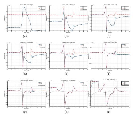
Figure 5.21: **Comparison of ED and VC results**. Both numerical simulations (ED, solid lines; VC, dashed lines) were generated on an identical computational grid and compared at the same positions as before in fig. 5.17, showing essentially same differences (dash-dotted lines).
