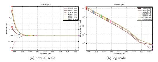
Figure 5.15: Charge density profile over Debye layer at various time points. As in fig. 5.13, the left panel is in normal scale, the right panel are the log-scaled absolute values. The kinks between  $y=518\,\mathrm{nm}$  and  $y=520\,\mathrm{nm}$  are a consequence of the charge density switching signs, as it is already close to zero. In both panels, the plotted markers correspond to the positions of the time courses in fig. 5.12.
