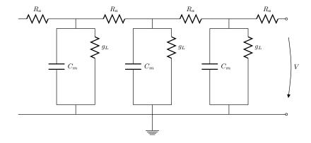
Figure 2.6: Equivalent circuit for a spatially extended neuronal membrane. Multiple (in this case passive) membrane patches are connected through axial resistances  $R_a$ , which in general are position-dependent.
