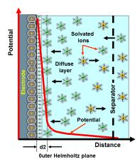
Figure 2.3: Schematic picture of a membrane and electrolyte. By Elcap (Own work) [CC0], via Wikimedia Commons
