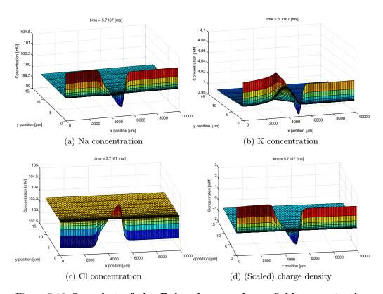
Figure 5.16: Snapshot of the Debye layer and nearfield concentration profiles. The concentration profiles of all three ion species and the charge density are plotted up to a distance of about 10 µm from the membrane. The strong concentration gradients close to the membrane demonstrate the influence of the Debye layer. The charge density can be seen to be dominated by the sodium concentration.
