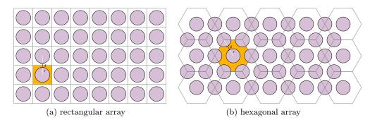
Figure 7.2: Illustration of axonal packing in different geometric arrangements. A regular rectangular packing (*left*) leads to a non-optimal packing ratio. The optimal packing can be achieved in a hexagonal array (*right*).
