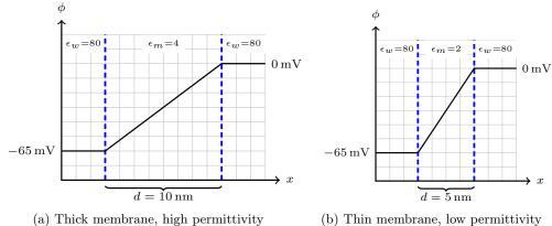
Figure 6.3: Relation of linear potential decay and membrane thickness/permittivity. Doubling membrane thickness and permittivity (left) results in the same membrane potential difference when the potential is linear across the membrane.
