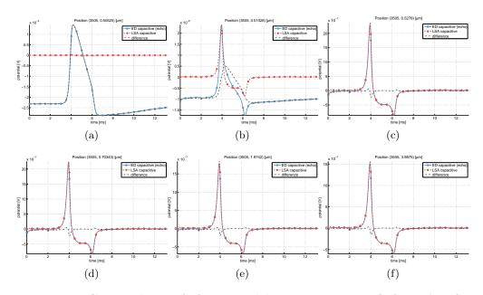
Figure 5.18: Comparison of the capacitive component of the EAP for ED and LSA. This shows only the capacitive component of the full EAP in fig. 5.17 for LSA (dashed lines) and ED (solid lines) model, as generated by the echo simulation.
