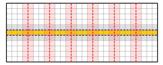
Figure 5.1: Partition of the unmyelinated axon computational domain for the parallel case. The computational domain with its three subdomains is shown as before; additionally, processor boundaries (vertical dashed lines) and overlap elements (shaded) are shown, in this case exemplary for p=7 processors. Note that this method gives optimal control over the load balancing and ensures that membrane interfaces never coincide with processor boundaries.
