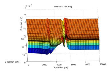
Figure 5.9: Snapshot of the nearfield extracellular potential profile. The plot shows the potential values for a stripe of the extracellular domain  $\Omega_{\rm ES}$  just above the extracellular Debye layer (i.e., above the gray area from fig. 3.1), at a fixed time. It shows a more complex structure compared to the Debye layer.
