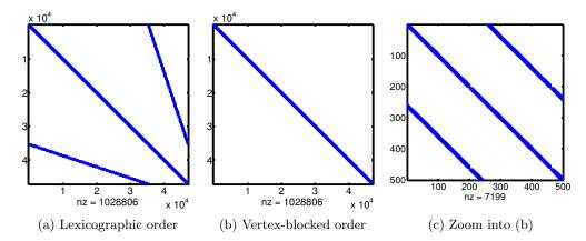
Figure 4.1: Comparison of matrix structure depending on DOF ordering. The left panel shows a lexicographic ordering of unknowns with an unfavorable sparsity pattern. Using a vertex-blocked ordering (center) yields an advantageous diagonal pattern, which reveals to consist of multiple block-diagonal matrices when zooming in (right).
