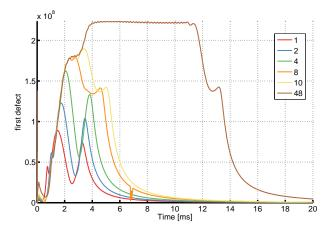
Figure 6.7: **Initial defect for different domain sizes**. The initial defect at the beginning of each time step is growing with processor count (and thus with domain size), since the AP wave spends a larger fraction of time within a longer axon.
