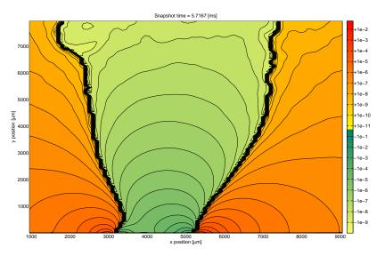
Figure 5.10: Snapshot of the whole extracellular potential. A contour plot of the log-scaled extracellular potential at a fixed time point. The domain was cut at the left, right, and upper boundary to exclude artifacts introduced by the boundary where the potential is almost zero and switches signs due to small numerical errors.
