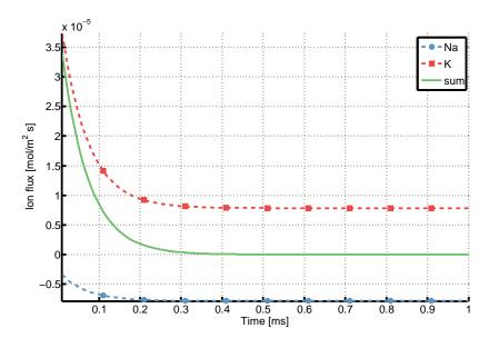
Figure 5.3: **Equilibration of membrane fluxes**. Na (lower line), K (upper line), and summed membrane fluxes (middle line) are shown for the equilibration phase. The sum of fluxes vanishes at equilibrium.
