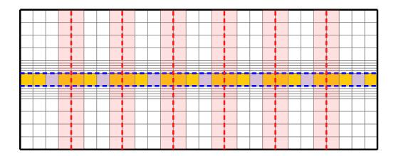
Figure 6.6: Partition of the computational domain for the parallel case. As in the unmyelinated case, the domain is divided by cuts in vertical direction. In the myelinated case, additional care has to be taken in order to not place the highly dynamic nodes of Ranvier close to a processor boundary, as suggested in the sketch.
