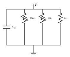
Figure 2.5: Equivalent circuit for the Hodgkin-Huxley membrane patch model. It consists of a membrane capacitance  $C_m$  in parallel with three branches, each consisting of a series of conductance and battery, representing the ionic current and reversal potentials, respectively. Note that the voltage-gated conductance are dynamic, while the leak conductance does not change over time. Reversal potentials of sodium  $(E_{\text{Na}})$  and potassium  $(E_{\text{K}})$  have opposite sign.
