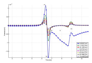
Figure 5.8: Extracellular potential at various distances from the membrane. The potential time courses for a fixed x-coordinate  $x = 5.05 \,\mathrm{mm}$  are shown for several different y positions. While the characteristic triphasic shape is maintained, the amplitude spans several orders of magnitude as the signal is strongly attenuated with distance.
