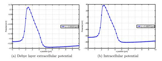
Figure 6.12: **Debye layer potential time course at node of Ranvier**. The Debye layer potential directly at the extracellular membrane interface (*left*) can be seen to directly correspond to the intracellular potential on the opposite membrane interface (*right*), the only difference being the amplitude, which was significantly reduced by the membrane.
