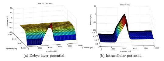
Figure 5.11: Snapshot of the Debye layer extracellular potential profile. In the left part, the potential values for a narrow stripe of the extracellular domain  $\Omega_{\rm ES}$  (corresponding to the gray area from fig. 3.1) just above the membrane are plotted at a fixed time. This turns out to be the intracellular action potential (right) propagating over the membrane, with a significantly reduced amplitude.
