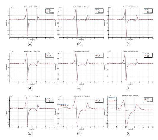
Figure 5.20: Comparison of numerical and LSA solution to the volume conductor equation. A wide range of extracellular points was used to assess the accuracy of the numerical solution (solid lines). The match is very good even at small membrane distances, indicating that the line source approximation (dashed lines) provides a suitable reduction of the full cylinder geometry. At larger distances, the influence of the upper Dirichlet boundary leads to notable deviations from LSA.
