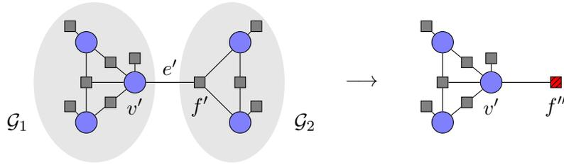
Figure 4.4: Bridge reduction: The right side of the original graph can be shrunk to a unary factor  $f''$  by  $|X_{v'}|$  small optimization problems. After solving the problem corresponding to the reduced graph, the full solution can be recovered.
