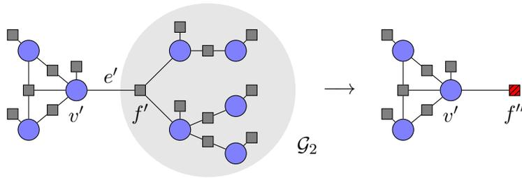
Figure 4.5: Tentacle reduction: In cases where  $\mathcal{G}_2$  is acyclic, i.e., is a tentacle, dynamic programming can be used to replace this subgraph by a single unary factor  $f''$ .
