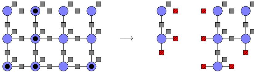
Figure 4.1: Partial optimality reduction: After applying a partial optimality algorithm, the nodes with known value (black dots) can be removed after modifying the factors connected to them appropriately (red).
