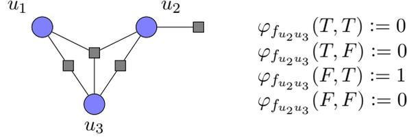
Figure 3.2: Transformation of an instance of the satisfiability problem into a discrete graphical model. The variables of SAT correspond to the variable nodes in the factor graph, the clauses to the factor nodes. The energy functions are 1 if and only if the corresponding clause is unsatisfied as is exemplarily shown for  $f_{u_2u_3}$ .
