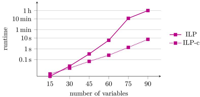
Figure 4.3: Average runtimes of ten binary instances per size. Each instance consists of three complete graphs of equal size. Standard ILP solvers are not able to capture this. Processing each connected component independently (ILP-c) leads to a significant speedup. Note that the time axis is logarithmic.
