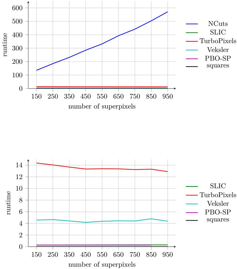
Figure 4.16: Runtimes of the superpixel algorithms: In the top plot it can be seen that NCuts is clearly the slowest method. The bottom plot is simply a zoomed in version of the top one to show the differences of the other methods.
