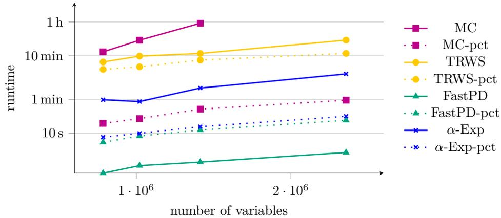
Figure 6.4: Runtimes for the brain dataset for different slice thicknesses which result in different numbers of variables. While for MC, the speedup caused by model-reduction is large, it is moderate or not present for approximative methods.
