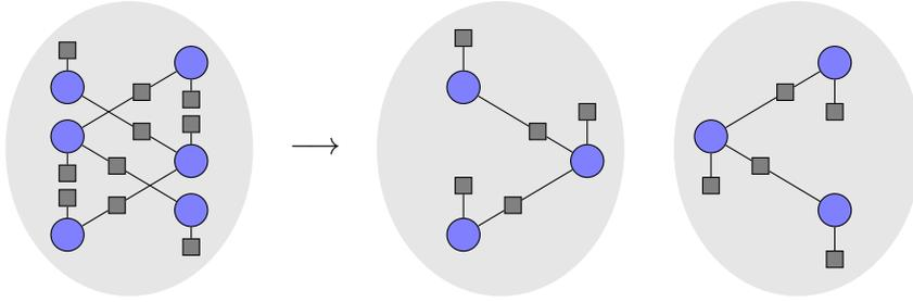
Figure 4.2: Connected component reduction: Obviously, each connected component of a factor graph can be treated separately.
