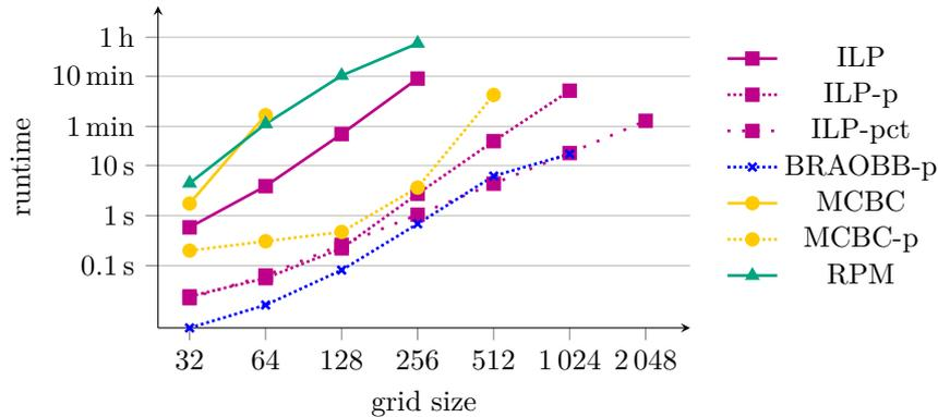
Figure 4.7: Average runtimes of those instances that could be solved in less than one hour (compare Fig. 4.8). For all methods reduction makes them applicable to larger instances. Overall, ILP-pct and BRAOBB-p perform best.
