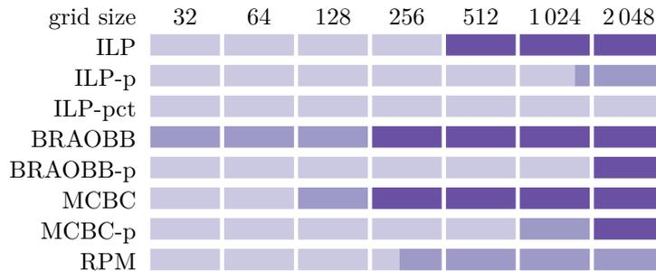
Figure 4.8: Fraction of the ten instances per grid size that could be solved within one hour (■), that could not be solved due to the time limit of one hour (■), and that could not be solved due to an out-of-memory error (■). Using the three proposed reduction techniques makes methods applicable to larger instances. Overall, ILP-pct scales best.
