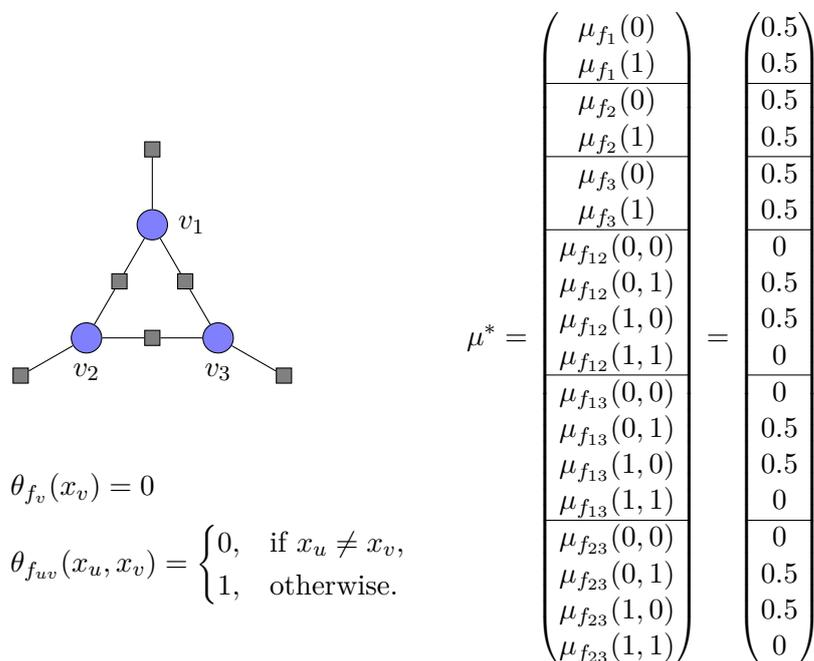
Figure 3.5: Fractional vertex of  $\mathbb{L}(\mathcal{M})$ : The fractional vertex  $\mu^*$  satisfies all constraints of the local polytope relaxation and is a vertex of  $\mathbb{L}(\mathcal{M})$ . For the energy function  $\theta$ , it is an optimal solution with a lower value than an optimal solution of the MAP problem.
