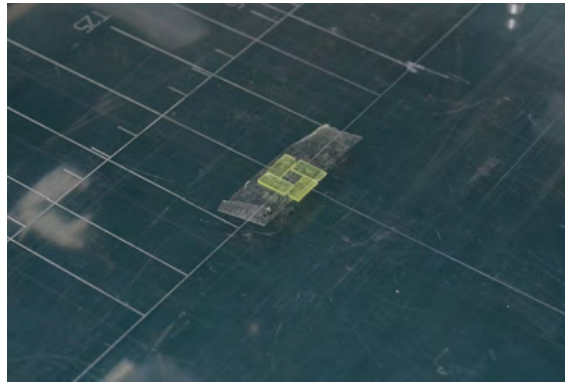
Figure 4.2: Fixation of FNTDs gk5003 ( \varphi = 0^\circ , left), gk5004 ( \varphi = +90^\circ , top), gk5005 ( \varphi = \pm 180^\circ , right) and gk5006 ( \varphi = -90^\circ , bottom)
