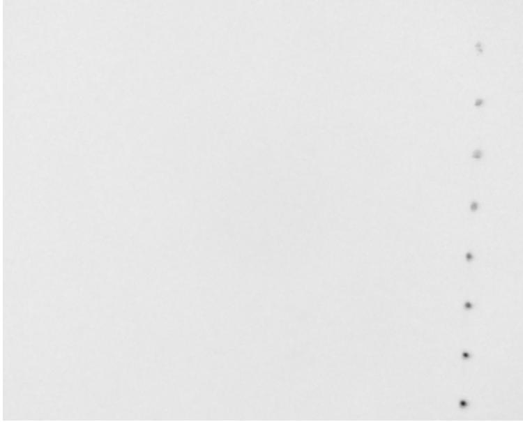
Figure 3.3.: Example image at 1.52 \text{ m s}^{-1} wind generator frequency from an IR sequence, which is inverted for better visibility. Darker colors correspond to higher temperature. The heated spot at the bottom has been drawn in the current frame. The flow is directed to the left. Dead pixels have been removed using a median filter.
