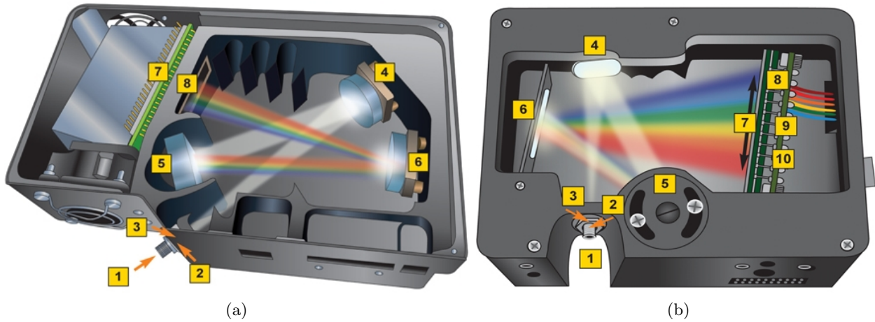
Figure 7.4: Sketch of the (a) QE and (b) USB spectrograph from Ocean Optics. (1) SMA 905 connector, (2) entrance slit, (3) longpass absorbing filter (optional), (4) collimating mirror, (5) grating, (6) focussing mirror, (7) collection lenses, (8) detector, (9) longpass order-sorting filter (optional), (10) UV2 and UV4 detector upgrades (optional). Images adapted from Ocean Optics, 2013 ( http://www.oceanoptics.com/ ).
