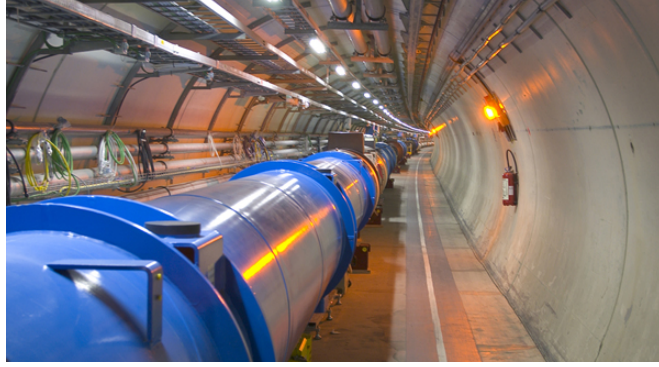
Figure 3.2.: Picture of the LHC with its superconducting magnets placed in the tunnel of the former LEP collider. Figure taken from Ref. [58]
