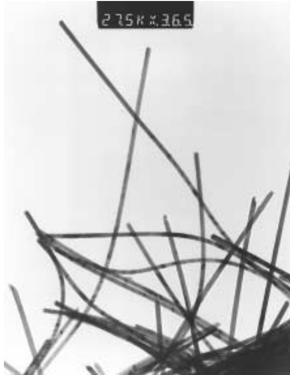
Figure 5.18: TEM image showing an array of copper nanowires of 45 nm diameter.
