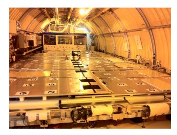
**Figure 2.4:** Lower outer veto in the laboratory of the far detector (from [51]). The chimney is seen in the middle of the outer veto modules, while the glovebox was not yet installed. In the back of the laboratory the entire DC electronics is stored, on the left hand side the HV splitter boxes are mounted to the side walls.
