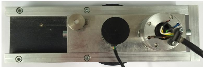
FIGURE B.4: Picture of the LED setup which provides switching between two LED lamps (without any daylight irradiation during the change of the LED lamp). It is designed to be mounted on a UV window of a UHV chamber for UV/vis irradiation experiments.
