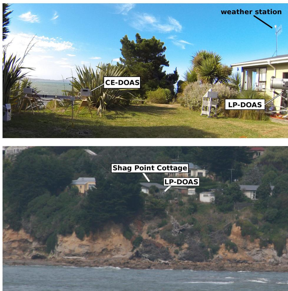
**Figure 13.2. | Shag Point Cottage with Instruments.** Top: Shown are the LP-DOAS, measuring along the light path indicated in Fig. 13.1, the CE-DOAS in (open) atmospheric measurement configuration (as on 03/07/2013) and on the roof of the cottage, the weather station Vaisala WXT520 and Kipp&Zonen CM11 is mounted. Bottom: The Cottage is located on a cliff about 15 m above the shoreline.
