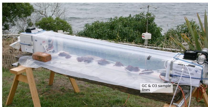
**Figure 13.17.** | **CE-DOAS with closed chamber.** In order to measure halocarbons and and ozone additional sample lines are connected to the chamber.
