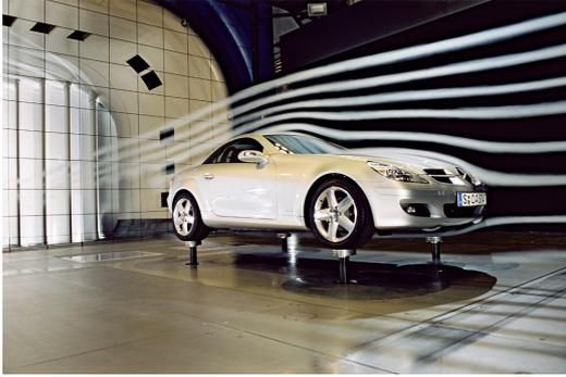
(a) Experimental path lines for a car in a wind channel [5]
