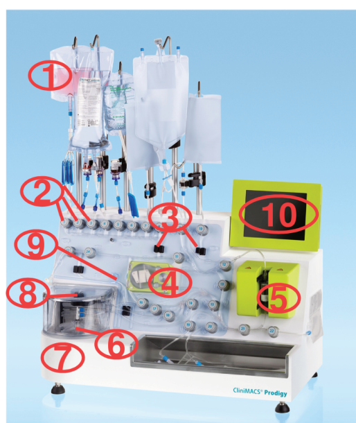
Figure 3.1 The CliniMACS Prodigy system incorporates several features for complex processing of cells for clinical use within a closed system. (1) Clinical bags are connected to a closed tubing set and allow sterile conditions during the process. (2) Several valves are used for controlled transfer of liquids and gas to the different components of the instrument. (3) Sensors for air bubbles allow discrimination between liquid and air in defined sections of the tubing, ensuring proper process control for handling of liquids and gases. (4) A pump transports liquids and gases in a defined speed. (5) Magnetic cell separation in clinical scale can be performed by a large MACS column and a special clinical scale magnet for MACS. (6) The CentriCult Unit allows centrifugation and cultivation of the cells. (7) Cultured cells can be observed by an installed microscope. (8) A camera for layer detection can be used during centrifugation and allows density gradient centrifugation including isolation of cells from a detected layer. (9) Defined gas supply is provided during cell culture applications. (10) Operation of the system and in-process control is done by a touch screen.
