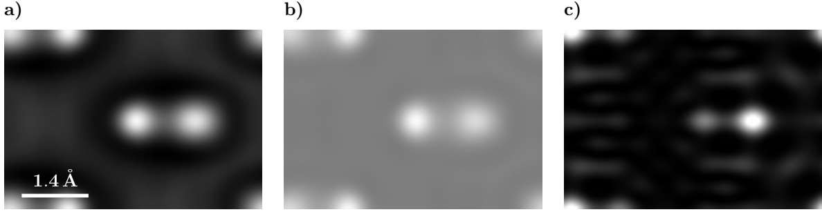
Figure 6.3: Simulation results for 46.8 nm silicon [110] at an acceleration voltage of 5 kV including backscattering effects. The images shown are calculated for an objective aperture of 100 mrad. a) Intensity of the wave-function |\psi|^2 in the detector plane. b) Corrections caused by the inclusion of backscattering. Shown are the differences with respect to the Matrix Forward algorithm described in section 5.2.1. The contrast of the difference image has been enhanced by a factor of 50. c) Intensity of the backscattered wave. This is the signal that would be found by a hypothetical second optical system and detector on top of the sample. The signal has been amplified by a factor of 2 \cdot 10^{13} .
