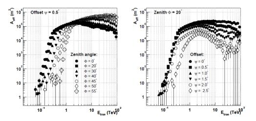
**Figure 4.14:** Effective area as function of the true energy for different Zenith angles and fixed off-axis angle (*left*) and for different off-axis angles and fixed Zenith angle (*right*). These are calculated for Hillas reconstruction and Standard cuts. Note that here the Zenith angle is referred to with  $\Phi$  and the offset with  $\Psi$  (from Funk 2005).
