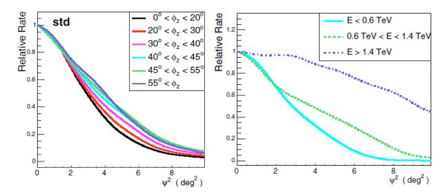
**Figure 4.11:** Radial acceptance from OFF source observations as function of the off-axis angle squared  $\Psi^2$  for different Zenith angles of the observation (*left*) and  $\gamma$ -ray energy (*right*), for the Hillas reconstruction using Standard cuts (from Berge et al. 2007). Note that in the text the off-axis angle is referred to with  $\theta$ .
