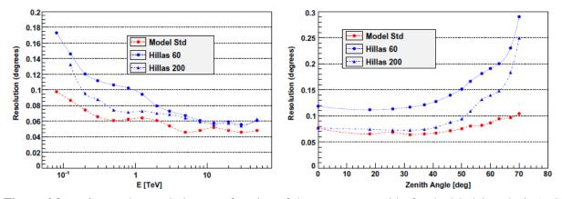
**Figure 4.9:** *Left*: angular resolution as a function of the energy, at zenith, for the Model analysis (red) compared to the values obtained for the Hillas analysis. *Right*: average angular resolution for a  $E^{-2}$  spectrum, as a function of zenith angle. From de Naurois & Rolland (2009).
