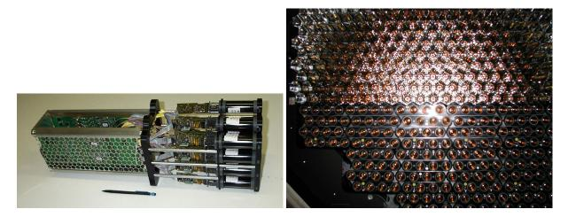
**Figure 3.7:** *Left*: a "drawer", consisting of 16 PMTs and all associated electronics. *Right*: front image of a HESS-I camera. In the upper half the hexagonal Winston cones are already in place, while in the lower half, one can see the bare PMTs. From https://www.mpi-hd.mpg.de/hfm/HESS/
