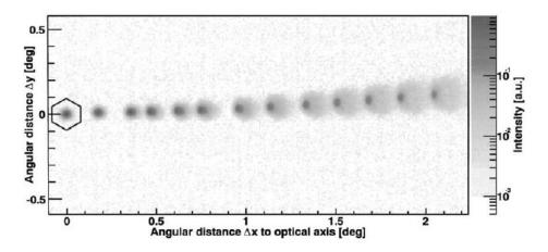
**Figure 3.6:** HESS-I PSF size of a star as function of the offset from the optical axis. The pixel size is indicated, as well (Cornils et al. 2003).
