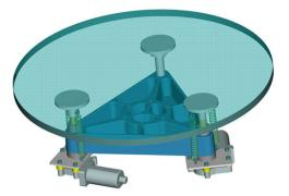
**Figure 3.4:** Drawing of a HESS-I mirror with its anchorage system. The same method is used for the HESS-II mirrors. From https://www.mpi-hd.mpg.de/hfm/HESS/.
