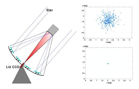
**Figure 3.5:** Mirror alignment technique. *Left*: a star is observed with a CCD camera positioned at the center of the dish, viewing the closed lid of the PMT camera. *Top-right*: star image before alignment. *Bottom-right*: star image after alignment (Cornils et al. 2003).
