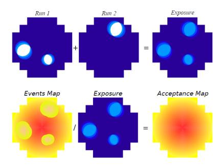
**Figure 4.12:** *Top*: run-wise exposure maps are summed together to create a cumulative averaged exposure map in the nominal system. *Bottom*: the nominal system acceptance map is derived dividing the event map by the exposure map (from De Naurois 2012).
