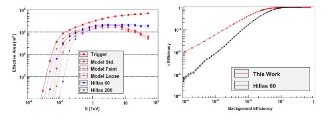
**Figure 4.7:** *Left*: Effective areas as function of energy, at zenith. In red, the values for the Model analysis for three different cuts, compared to the Hillas analysis, in blue. *Right*: Model  $\gamma$ -ray efficiency (red) as function of the background rejection for a selection based on *ShowerGoodness* only, after shape cuts, compared to the results of the standard Hillas reconstruction (black) using the MRSW and MRSL variables. From de Naurois & Rolland (2009).
