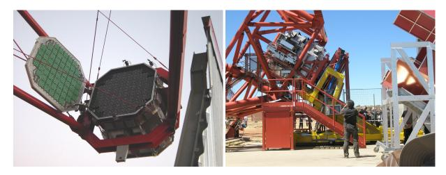
**Figure 3.8:** Left: HESS-I camera with open lid inside its support (from https://www.mpi-hd.mpg. de/hfm/HESS/). *Right*: CT 5 camera being unloaded from the quadrupod as demonstration during the inauguration in September 2012.
