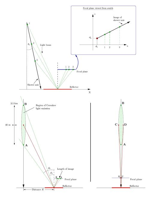
**Figure 4.1:** Mapping of an air shower onto the telescope camera. *Top*: the orientation of the image depends on the inclination of the shower axis with respect to the telescope optical axis. *Bottom*: the shape and size of the distribution depends on  $\Delta \phi = \phi_2 - \phi_1$ , *R* and the width of the shower (from Berge 2006).
