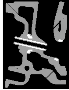
Figure 5.2: The figure shows the GMDs at iteration 1 (top), 15,000 (middle) and 35,000 (bottom) on the left side and the corresponding reconstruction of ML-EM-GATV on the right side. The reconstruction settings were: 40 projections, SNR = 2236. The GMDs show the true Gradient Magnitudes of the reference data (squares), the GMs of ML-EM-GATV (gray dots with a black border) and the currently penalized GMs (represented by a solid line) at different optimization steps. Note, we do not display a GM of intensity 0 for the sake of clarity.
