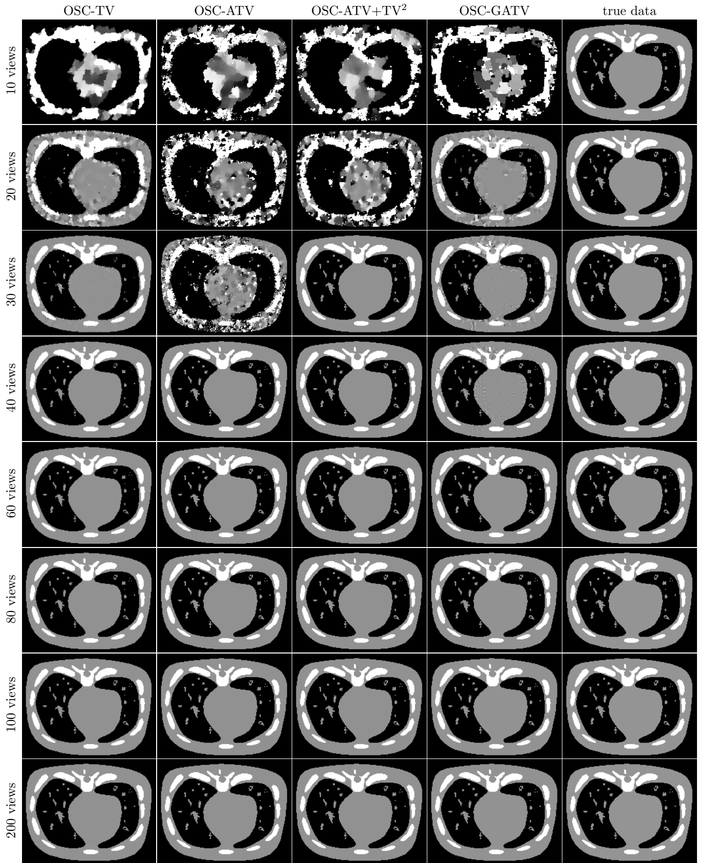
Figure 6.5: Reconstructions of the lung phantom from different numbers of noise-free projections, window-level: [0.0160, 0.0178] .
