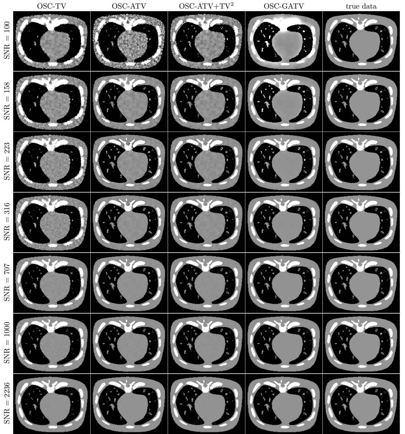
Figure 6.6: Reconstructions of the lung phantom from 40 projections, different noise levels and 10 different realizations of the random noise variable. The mean of the results is displayed, window-level: [0.0160,0.0178].
