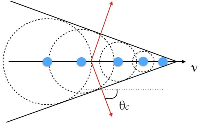
Figure 2.3: Schematic showing the production of Cherenkov radiation at an emission angle  $\theta_C$  to the trajectory of a particle moving at  $v$ . The emission from all parts of the particles trajectory forms a coherent wavefront under Huygen's construction, which moves outwards at  $c$ .
