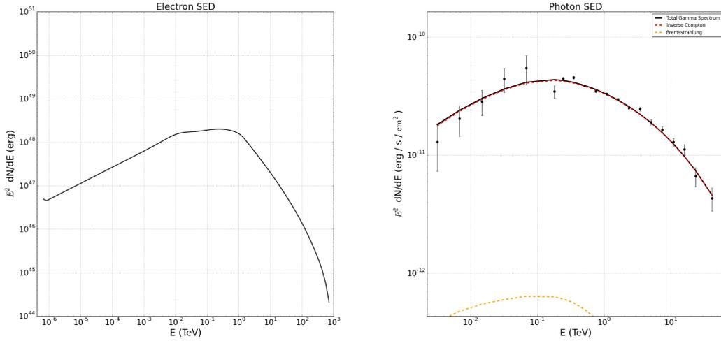
Figure 7.20: The evolved particle spectrum and resulting  $\gamma$ -ray spectrum from model 1 with enhanced kinematic evolutionary phases. In this case, the radius is constrained to reach 40 pc at  $t = T$ . The  $\gamma$ -ray spectrum is dominated by Inverse Compton emission, with a small Bremsstrahlung contribution. The data points seem to be better matched with a 40 pc radius than the 20 pc of figure 7.19.
