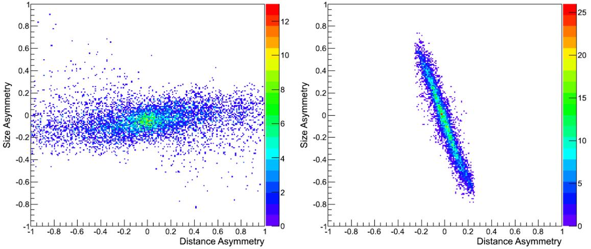
Figure 4.2: Two main components contribute to the Monte Carlo event distribution in a histogram of image size asymmetry against core distance asymmetry (at  $20^\circ$  zenith angle). A horizontal component is due to events with a core distance,  $d \lesssim 125$  m in both telescopes (left) and an anti-linear component arising from events with  $d \gtrsim 125$  m in both telescopes (right).
