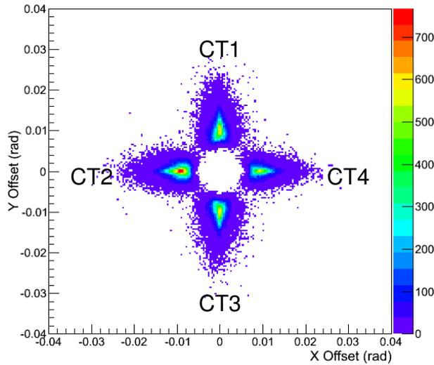
Figure A.4: Offset distributions between CT5 and each of CT1-4, obtained from gamma simulations at  $\theta_z = 20^\circ$ . The orientation of the distribution depends on the geometry of the array layout, with distributions from each pairwise comparison clearly isolated. Anticlockwise from the top, these correspond to offsets between CT5 and CT1, CT2, CT3, CT4 respectively.
