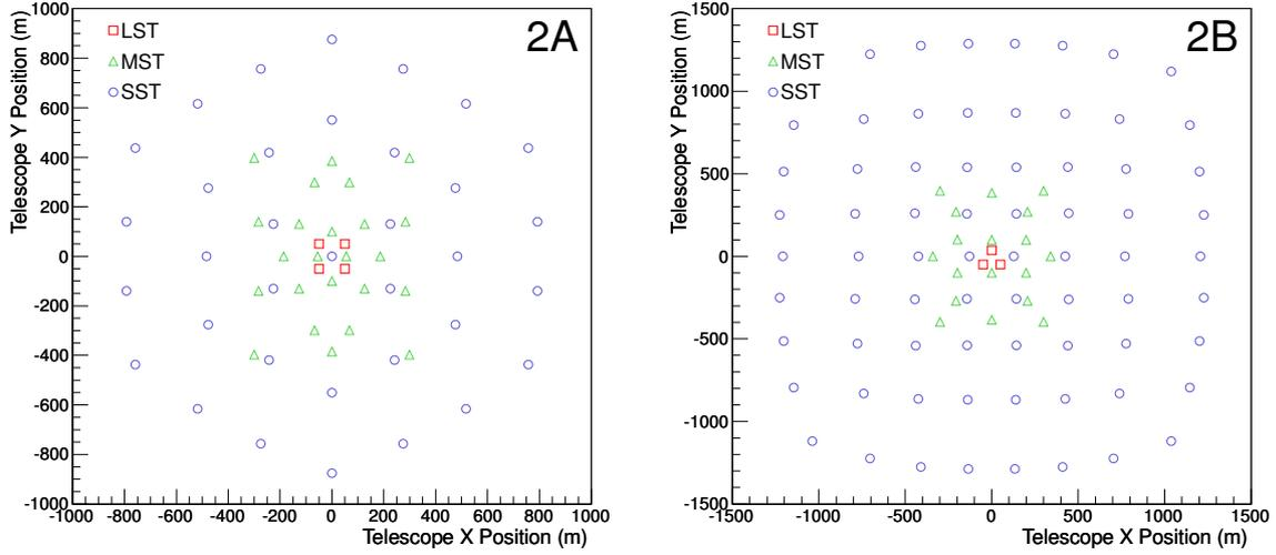
Figure 4.16: Array layouts used in the MC studies performed, with number of telescopes and primary mirror diameters as follows. Left: Layout 2A comprising 63 telescopes; 4 LSTs (23 m), 24 MSTs (12 m) and 35 DC-SSTs (7 m). Right: Layout 2B comprising 93 telescopes; 3 LSTs (23 m), 18 MSTs (12 m) and 72 SC-SSTs (4 m).
