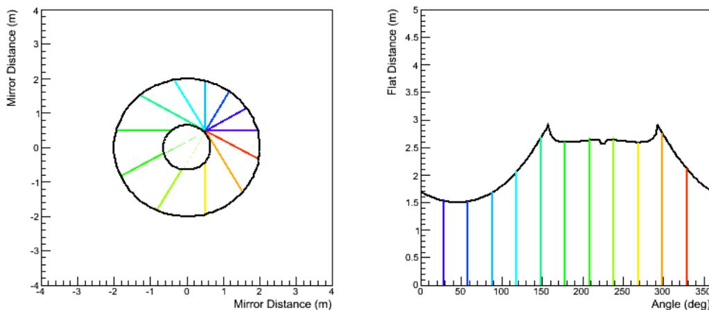
Figure 3.38: Variation in distance traversed across both mirrors of the dual mirror telescope with azimuthal angle, shown in the case of an on-axis muon (offset from the mirror centre, left). Right: The effect of including the distance traversed by the light across the secondary mirror is to reduce the depth of the dip induced by the hole of the primary mirror. Only the primary mirror is shown on the left.
