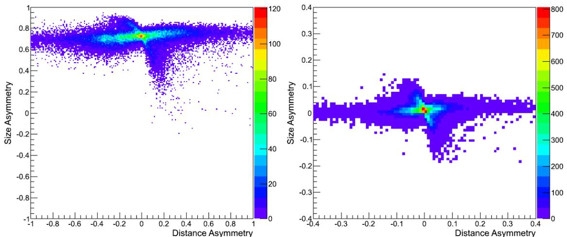
Figure 4.6: Monte Carlo size distance histogram between two H.E.S.S. telescopes (CT5 and CT1) of  $600 \text{ m}^2$  and a  $100 \text{ m}^2$  mirror area respectively. Left: the distribution has clearly been shifted from that in figure 4.2.2. Right: the image size in CT5 has been rescaled using an expected size ratio from simulations. This rescaling was performed using the logarithm of the image sizes, such that the distribution appears squashed, as well as shifted back to be centred on zero.
