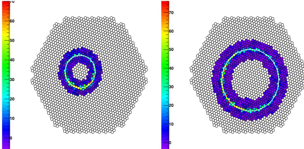
Figure 3.35: An example simulated muon event in an MST (left) and an LST (right). Although the cameras are differently shaped to the H.E.S.S. cameras, this does not affect formation or parameterisation of the ring images. The centres of the muon rings are offset from the camera centres, corresponding to muons inclined to the telescope axis (see figure 3.1).
