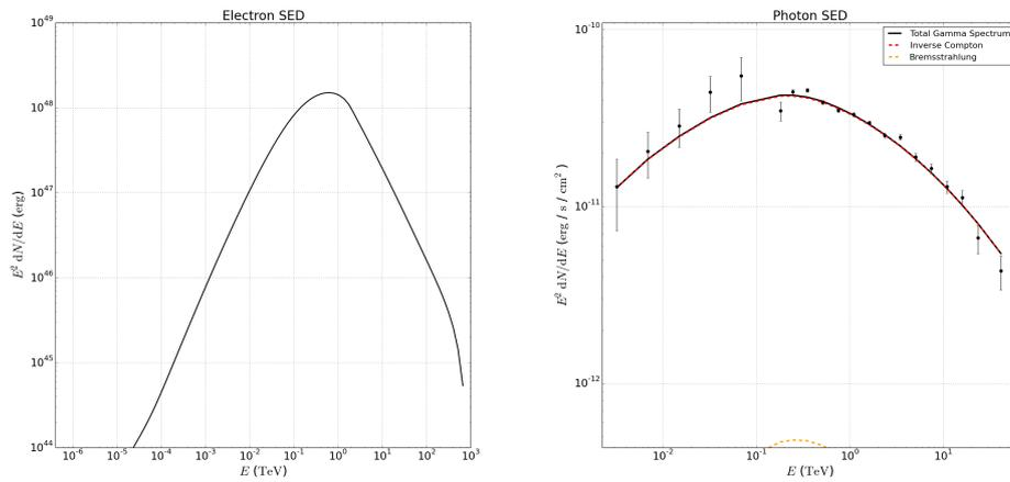
Figure 7.15: The evolved particle spectrum and resulting  $\gamma$ -ray spectrum from the free expansion model 1. The  $\gamma$ -ray spectrum is dominated by Inverse Compton emission, with a small Bremsstrahlung contribution. The parameters of the initial particle spectrum are listed in table 7.11. Systematic errors have been used for the Fermi-LAT points from Grondin et al [111], whereas the H.E.S.S. points from the dataset A analysis of chapter 6 are shown with statistical errors only.
