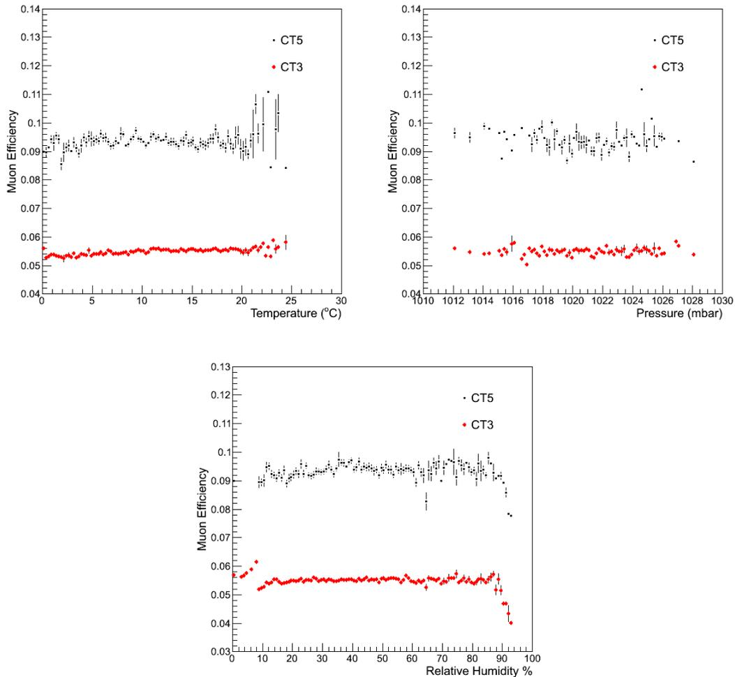
Figure 3.28: Top: Variation of muon efficiency with atmospheric parameters - no significant dependence of the muon efficiency on temperature (left) or atmospheric pressure (right) is seen. Bottom: the muon efficiency can be seen to drop when the relative humidity rises above  $\gtrsim 80\%$ .
