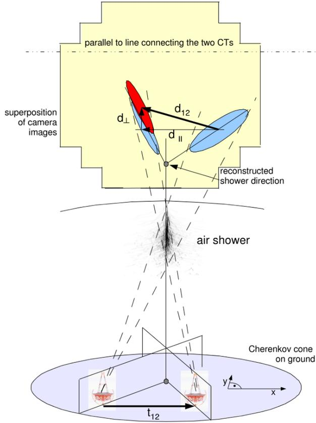
Figure A.3: Geometry of shower image comparison for pointing calibration, taken from [39]. The parallel ( $d_{||}$ ) and orthogonal ( $d_{\perp}$ ) offsets in the centres of gravity may indicate a pointing miscalibration.
