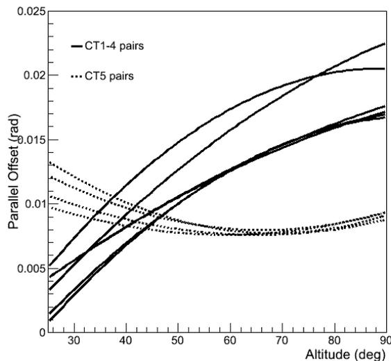
Figure A.5: Parallel pointing offset between telescopes without standard pointing corrections applied. Offsets in H.E.S.S. I pairwise comparisons tend to increase with increasing altitude, whilst pairs involving CT5 tend to decrease and flatten.
