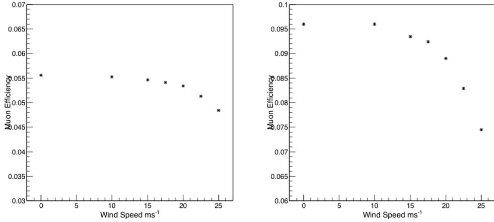
Figure 3.27: Muon Efficiency in CT1 (left) and CT5 as a function of wind speed (equivalent to the level of aerosols in the atmosphere). Results are from MC with the same input efficiency at all wind speeds (88% for CT5). Note that the wind speed rarely exceeds  $6\text{-}7\text{ms}^{-1}$  under normal data taking conditions, whilst the aerosol content is monitored by the Cherenkov Transparency Coefficient [38].
