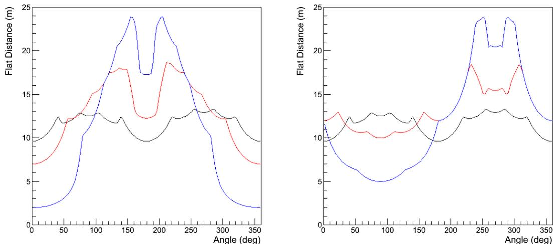
Figure 3.10: Variation in the distance  $D(\rho, \phi)$  across the CT5 reflector dish with azimuth angle, shown (left) for fixed vertical position at 0 m and horizontal displacements of 0 (black), 5 (red) and 10 m (blue), and (right) for fixed horizontal position at 0 m and vertical displacements of 0 (black), 5 (red) and 10 m (blue). The effect of the corners and mirror edges is clearly noticeable in the profile shape as a function of azimuth angle.
