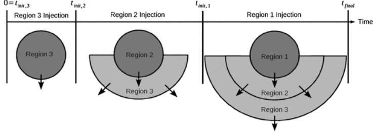
Figure 7.12: Figure taken from [109], illustrating their multi-zone approach. Each zone is injected at the same central location, yet separated in time, with the same size, zone shape and injection spectrum. The particles then diffuse away and into neighbouring zones (arrows) cooling in the process (light grey).
