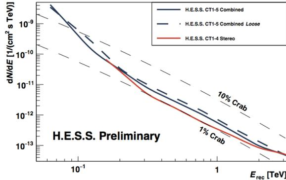
Figure 2.14: Differential sensitivity of H.E.S.S. II using a combined analysis (mono and stereo events), for observations at  $\sim 12^\circ - 22^\circ$  zenith angle. The performance is significantly better than that of CT1-4 only at low energies. Figure taken from [56].
