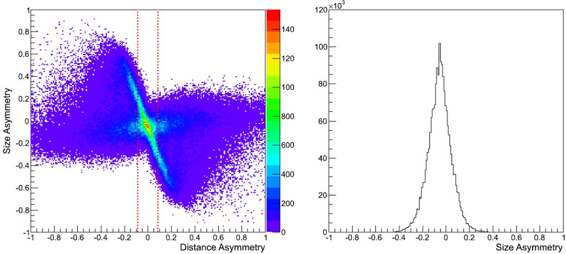
Figure 4.1: Monte Carlo histogram of image size asymmetry against distance asymmetry (left) features a horizontal and anti-linear component. Cutting on the absolute value of the distance asymmetry,  $|a_d|$  (as shown by dotted lines) leaves a symmetric distribution of size asymmetries (right), the mean of which is a measure of the response efficiency asymmetry between two telescopes.
