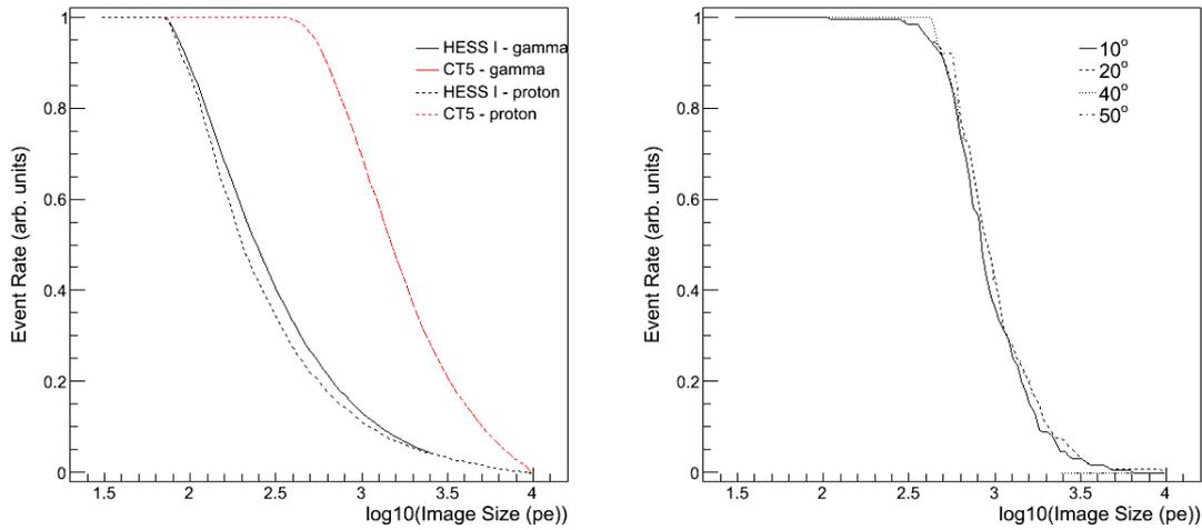
Figure A.1: Cosmic ray rate (in arbitrary units) variation with image size as determined from Monte Carlo. Left: The shape of the curve remains similar between  $\gamma$ -ray and proton Monte Carlo, with almost no discernible change for CT5 with respect to CT1-4. Right: There is no considerable change in the shape of the curve with zenith angle (the curves having been normalised to a maximum of 1).
