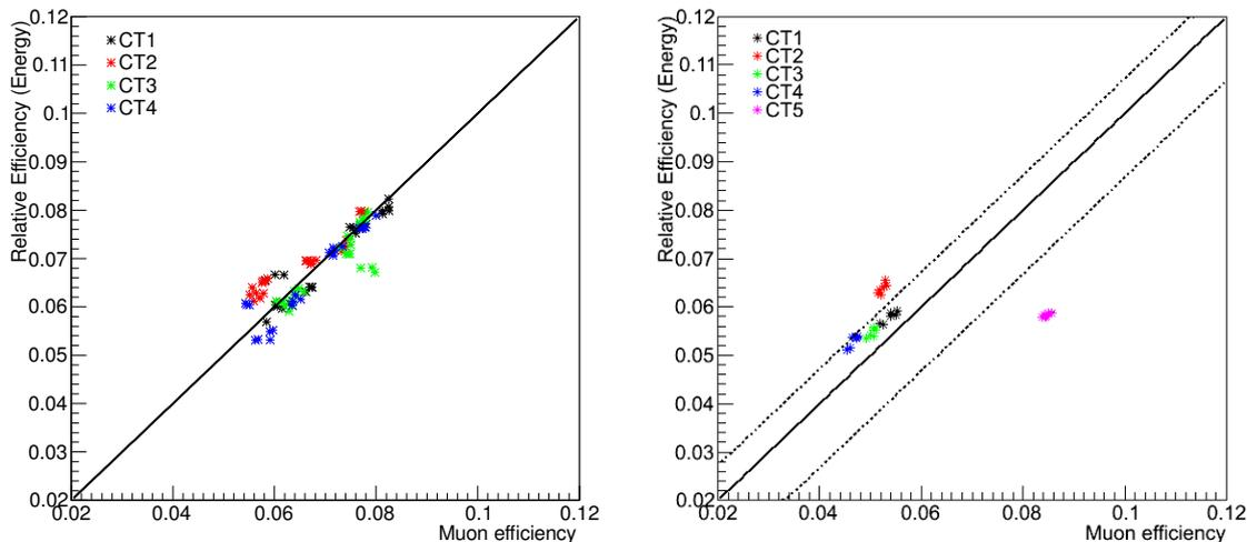
Figure 5.6: Optical Efficiency recovered using the cross calibration with reconstructed energy and the muon calibration approaches from Crab Nebula data taken with H.E.S.S. during its first (left) and second (right) phases of operation. No muon correction was applied to the reconstructed energies. The expected level of deviation due to the MC reference optical efficiencies not being the same for all telescopes in phase 2 is indicated by the dashed lines, for CT4 (above) and CT5 (below).
