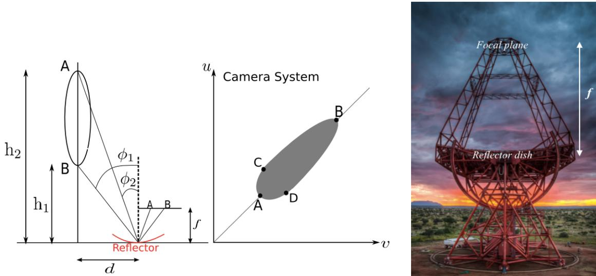
Figure 2.5: Left: schematic demonstrating the imaging geometry of IACTs, reflecting the Cherenkov light from an extensive air shower onto the camera. Right: Photo of the fifth H.E.S.S. telescope, showing the large reflector dish and the camera, onto which the light is focused. Figures taken from [28] and [29].
