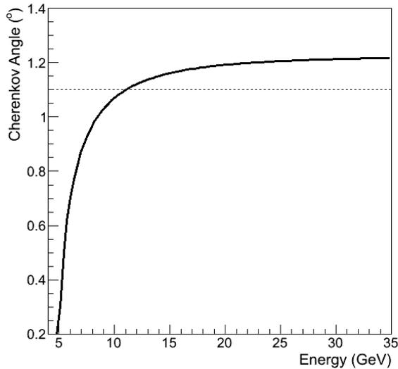
Figure 3.4: Muon ring radius (opening angle of the Cherenkov cone) as a function of energy. Above  $\sim 15 - 20$  GeV, the Cherenkov angle  $\theta_c$  approaches a constant value of  $\sim 1.21^\circ$ . The lower bound on the ring radius used in selection of muon events for calibration in CT5 is marked by a dashed line.
