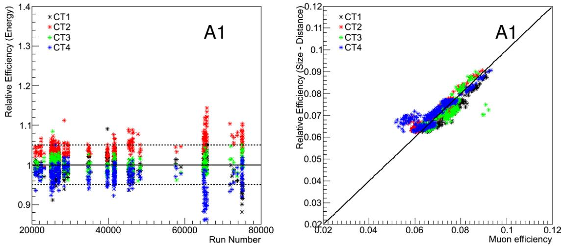
Figure 6.7: Results of the cross calibration on dataset A1. Left: the relative efficiencies obtained via the reconstructed energy approach lie generally within the acceptable tolerance level, except for a time period during which CT4 was significantly degraded with respect to the other telescopes. Right: correlation of the image size based relative efficiencies with the muon efficiency values. The few large outliers correspond to the time period of considerably degraded CT4.
