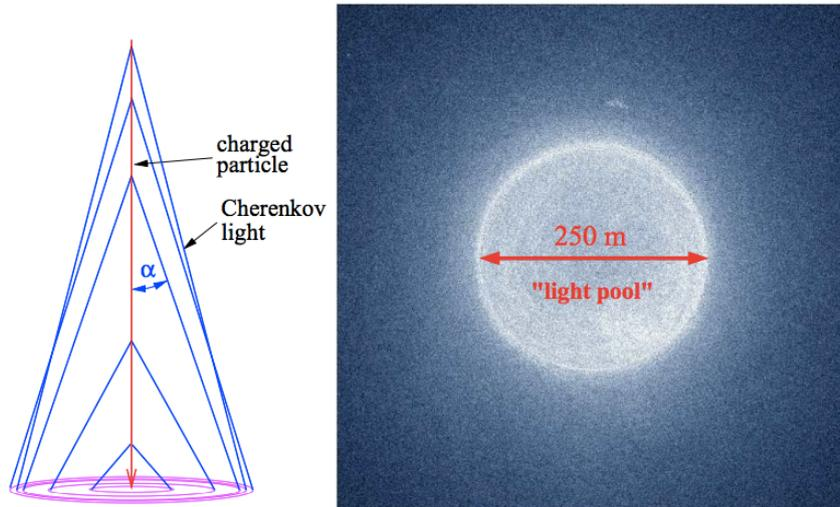
Figure 2.4: Changes in the refractive index with height lead to changes in the Cherenkov emission angle, labelled  $\alpha$  here. This leads to a light pool of approximately 250 m diameter (seen at an observation level of 1800 m) with higher emission levels near the edge. Figure taken from [22].
