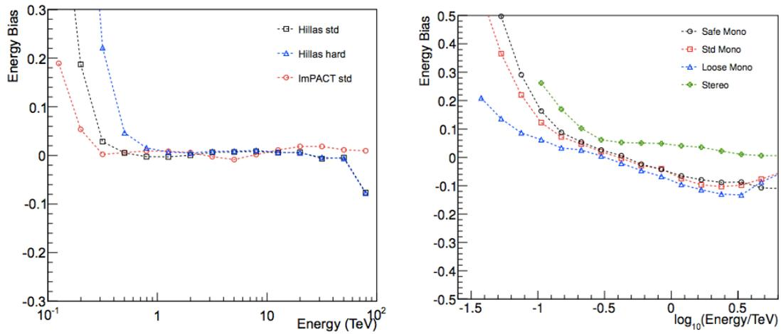
Figure 2.12: Energy bias of H.E.S.S. as a function of energy. Left: likelihood based analyses show improved performance over Hillas based analyses. Right: The energy threshold is considerably lowered by CT5. Figures taken from [47] and [54].
