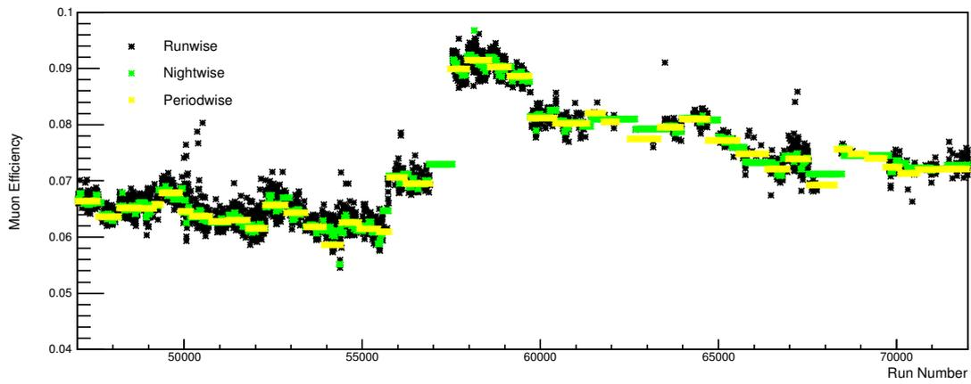
Figure 3.32: Evolution of muon efficiency (CT3) shown for run-wise, night-wise and period-wise averaged values. Statistical variation and anomalous values (due to short runs or weather conditions) are clearly reduced by night-wise averaging, whilst period-wise is a more crude approximation.
