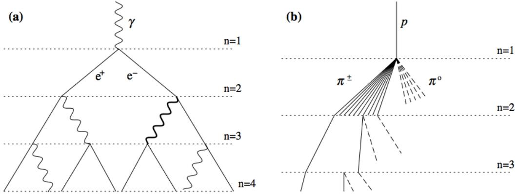
Figure 2.1: Schematic showing the development of an electromagnetic (a) and a hadronic (b) shower cascade under the Heitler model. Figure taken from [19].
