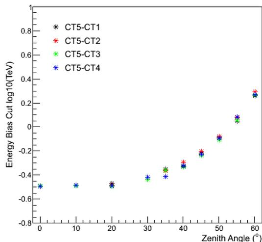
Figure 4.12: Above zenith angles of  $\sim 30^\circ$ , the energy bias cut shifts towards higher energies with increasing zenith angle. This is a consequence of the increasing energy threshold (see also figure 2.13 of chapter 2).
