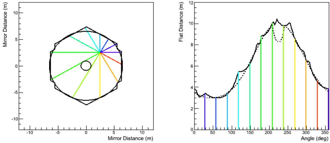
Figure 3.8: Variation of the distance to the mirror edge with azimuth angle for a given impact position, shown for the H.E.S.S. I telescopes under a circular approximation and using interpolation between a set of points. A circle is a good approximation to the mirror shape, and deviations are only minor. An example muon with an impact position offset from the mirror centre is chosen to illustrate the asymmetrical effect on the 1D profile.
