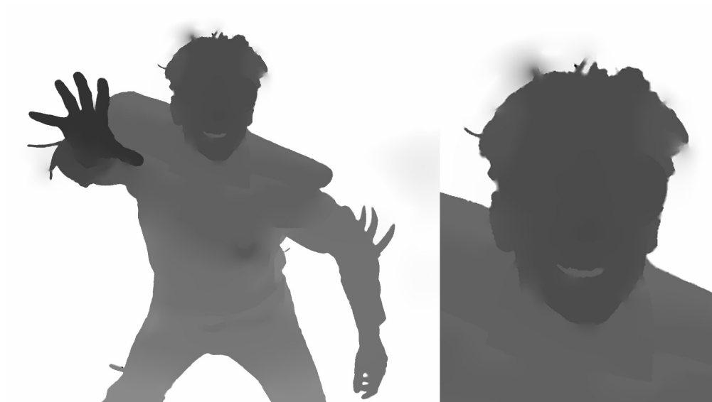
Figure 4.6: Depth maps results for scene 2. We obtain detailed results using user scribbles. Color bleeding can be seen at a few depth boundaries.
