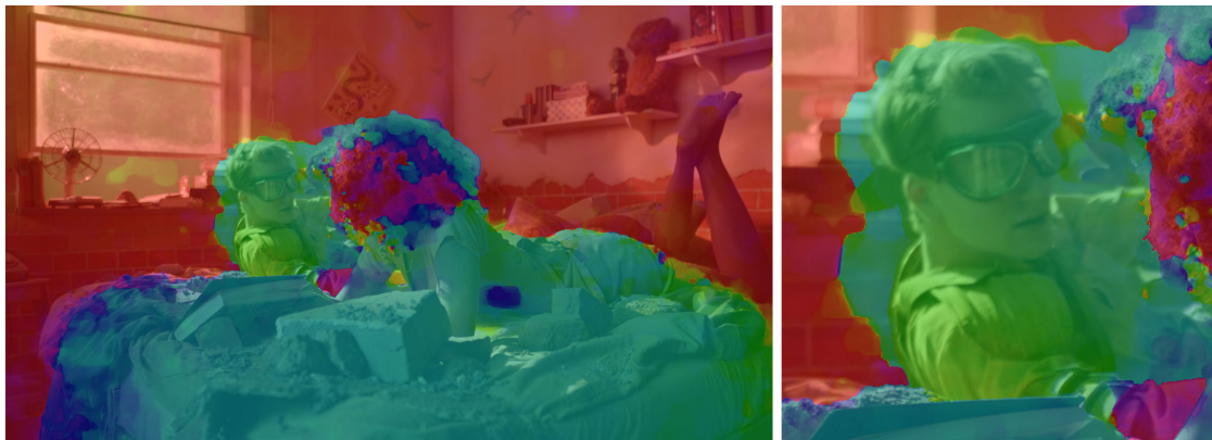
Figure 3.4: This figure shows a state-of-the-art optical flow result ([83]). Optical flow especially performs poorly at depth discontinuities. The colors in this figure represent the measured flow direction.
