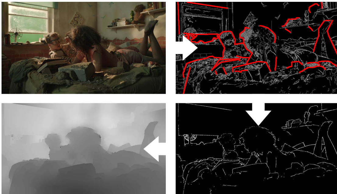
Figure 2.1: Depth discontinuities are labelled, learned by a random forest and afterwards predicted for several subsequent frames. We use those discontinuity edges as interpolation regularization. Thus, depth maps can be interpolated from sparse depth information. As result, our depth maps are smooth with sharp edges only at discontinuities.
