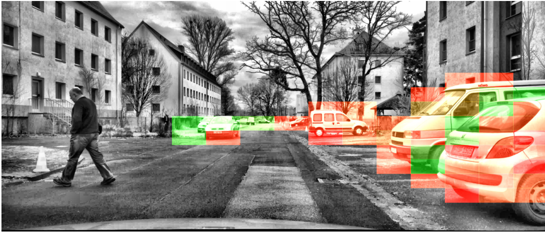
Figure 11.5: To determine boundaries between objects, we asked whether a box contains more than one vehicle. The green boxes on the lower right corner clearly divide both vehicles.
