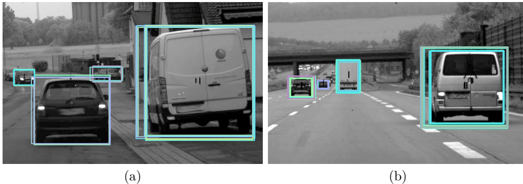
Figure 10.21: We tested propagation workflows on bounding box projects to test this approach on a more favourable setting. Our instructions again turned out to be vague. Some of the participants included side mirrors into their annotations, some did not. If one relies on algorithms such as majority votes, such ambiguities have to be avoided to achieve optimal results.
