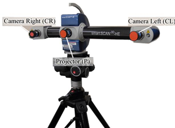
Figure 3.3: The structured-light 3D scanner– *Breuckmann smartSCAN HE*.
