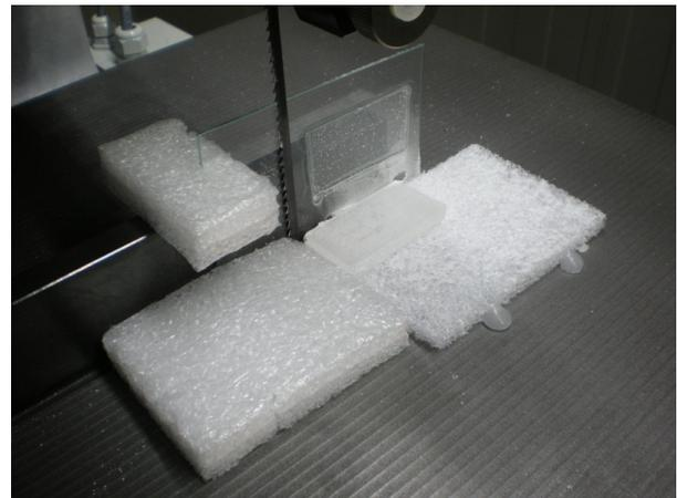
Start the saw and push the slide continuously with the help of styrofoam pieces or thick brushes **slowly** towards the back and slightly towards the metal boundary. A fixed piece of styrofoam can help preventing the break of the cut off thick section. **Observe and practice the sawing on some waste ice first!**
