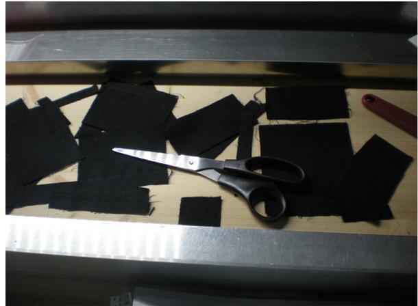
For the LASM recording a black background is needed which is provided by pieces of black cloth. Find or prepare a piece that fits the length of the sample, it should be just as long or a tiny bit longer. Align the sample on top of the cloth parallel to the stage border and with top arrow pointing to the back.
