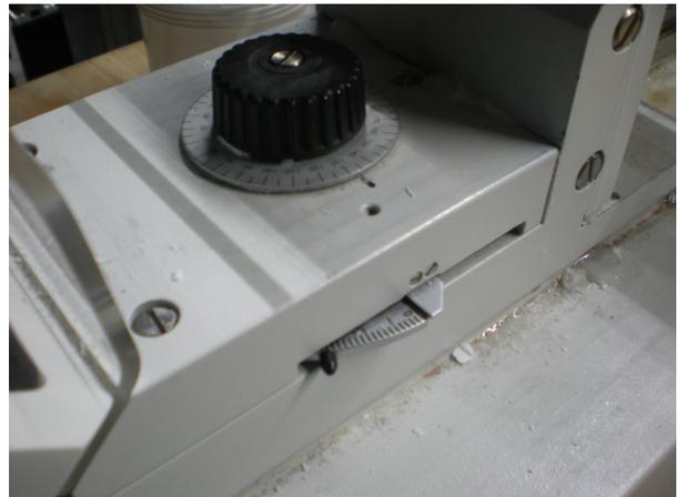
Before you start with microtoming **make sure the wheel scale on the side of the sledge is set to zero** – otherwise the stage will be raised automatically each time the sledge reaches the front! One turn of the dial corresponds to  $250\ \mu\text{m}$ .
