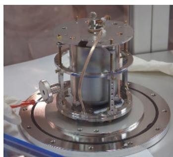
(e) semi-coaxial detector in jig prepared for transport
