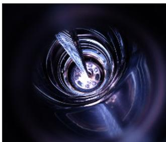
(f) view through lock into cryostat on top PMT plate
