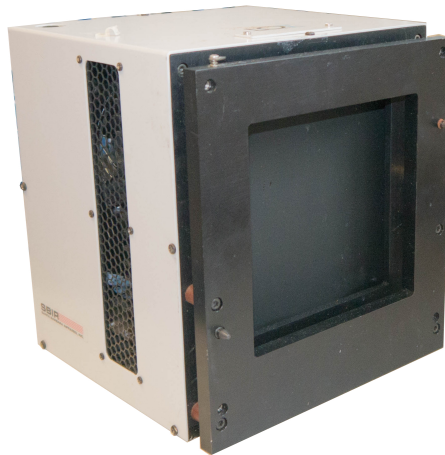
Figure 4.13.: Photo of the black body calibration unit used to calibrate the IR camera. The inner black surface at the front is the area used for the calibration.
