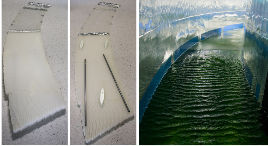
Figure 4.3.: Pictures of the wave absorber used in the Aeolotron. The left picture shows the wave absorber from the top, the middle picture shows the support structures on the bottom side, that are needed to make it more stiff and to maintain it from sinking to deep into the water. The right picture shows the wave absorber installed in the Aeolotron's water channel. Pictures taken from Kropp [64].
