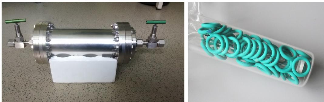
**Figure 4.10.:** (Left) Picture of the O-ring emanation source vessel as it was integrated in the interface gas system. (Right) Sample of the same type of viton O-rings (Novotek) prepared for radon emanation measurements using proportional counters.
