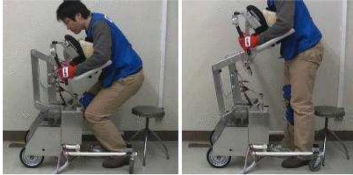
Figure 1.8: Prototype of the Chugo device providing STS support to a subject [26].
