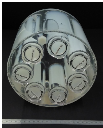
Figure 3.3: Image of the phantom with different agarose concentrations. The smaller tubes are filled with agarose concentration from 1% to 7% and have a diameter of 43 mm. They are surrounded by pure 0.9% NaCl solution in a cylinder of 190 mm diameter.
