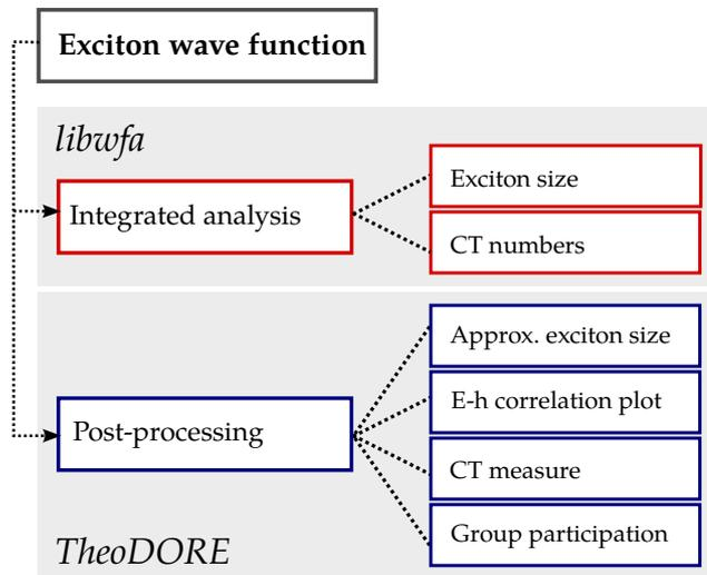
Figure 4.1: Wave function analysis software used in this chapter: the libwfa library and the TheoDORE program package.
