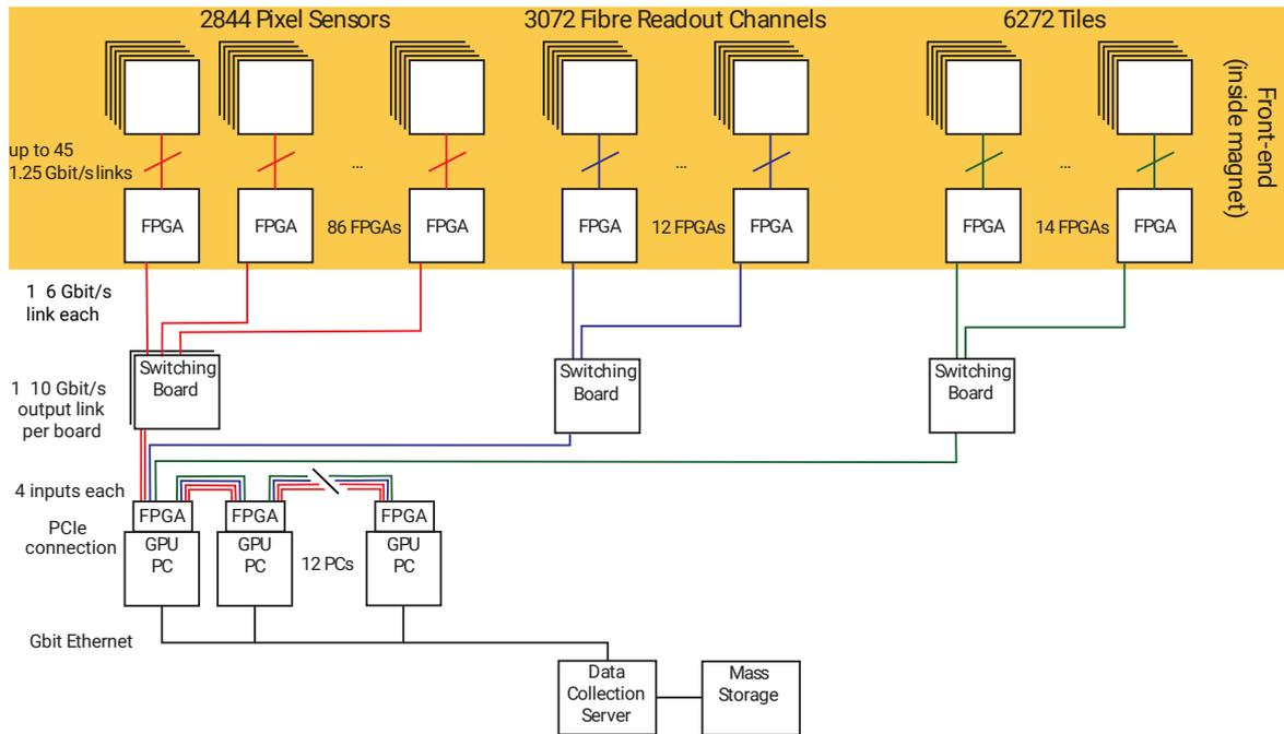
**Figure 2.16:** Schematic of the DAQ system [53].
