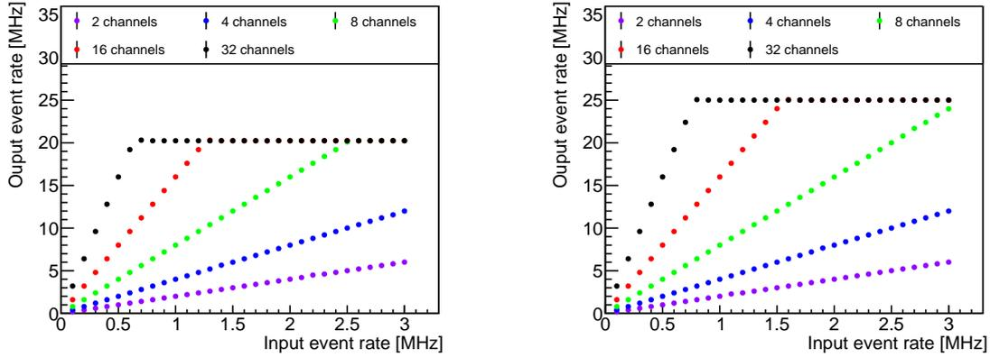
**Figure 6.13:** Output Event rate as a function of the input event rate. The test pulse is injected into 2, 4, 8, 16, 32 channels respectively. Left: standard event length configuration, where the hit event data has 48 bit. Right: short event length configuration, where the hit event data has 27 bit.
