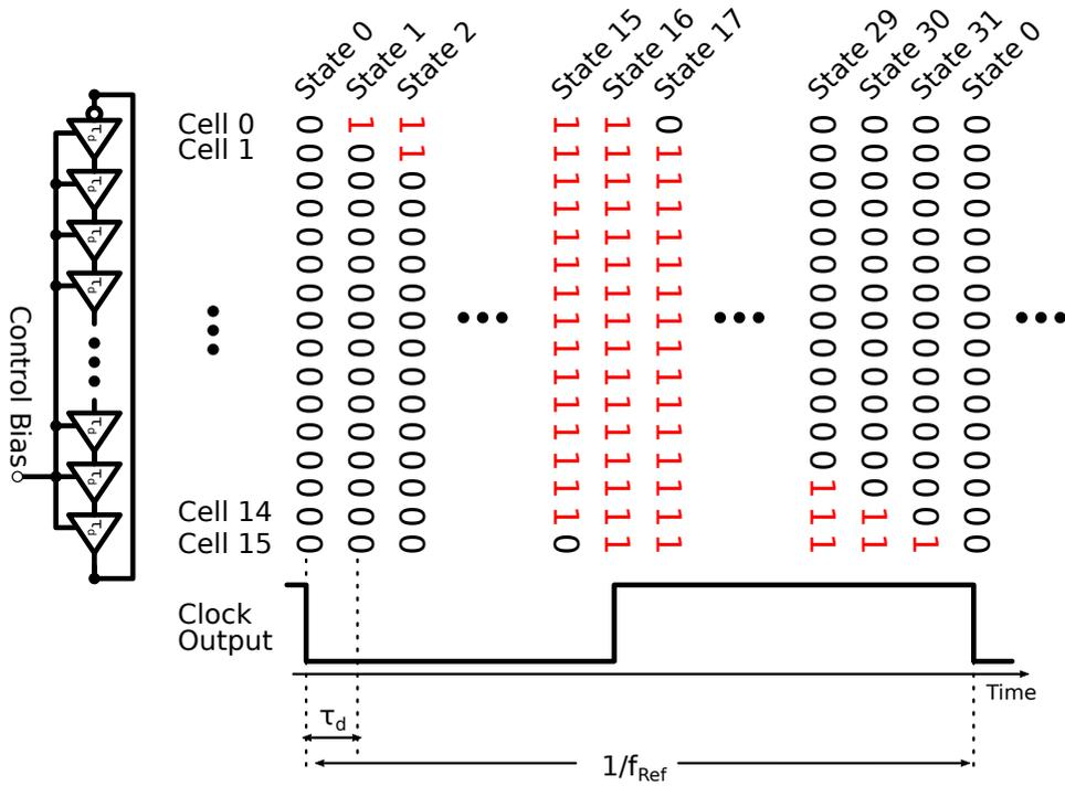
Figure 5.9: Working principle of the VCO cell.
