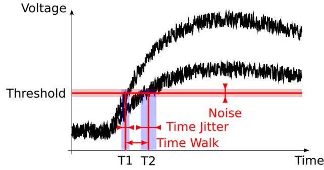
**Figure 3.11:** Timing errors with leading edge discrimination.
