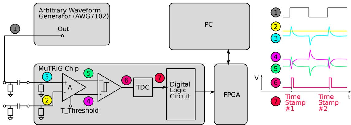
Figure 6.7: Full chain jitter measurement setup.
