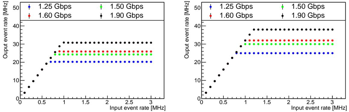
**Figure 6.14:** Event rate measurement result for different serial data link bit rate with the standard (left) and the short (right) event configurations.
