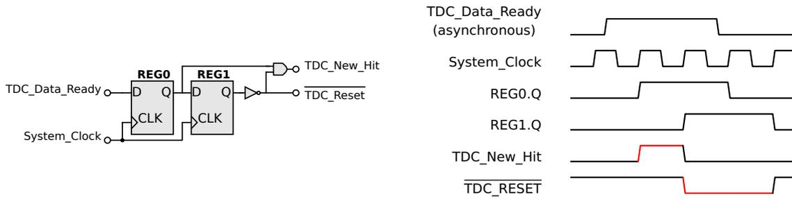
**Figure 5.12:** Schematic and the timing diagram of the circuit for generating the TDC\_New\_Hit and TDC\_Reset signals. The red pulses indicates the assertion of the signals.
