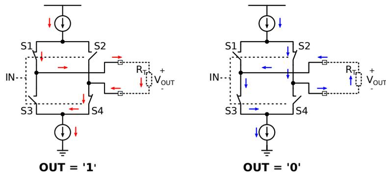
Figure 5.21: Working principle of the LVDS driver.
