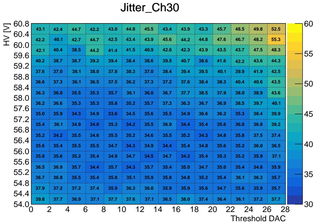
Figure 6.20: Timing resolution of channel 30 at all the tested configurations.
