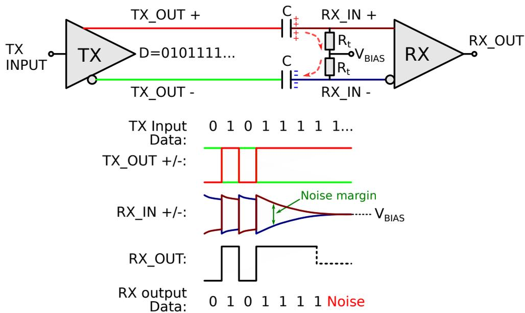
**Figure 5.18:** An example of DC unbalanced data over the AC-coupled LVDS link. The red arrows indicate the current due to the flow of charge stored on the right conductor plane of capacitances  $C$  after the signal transition. Essentially the voltages of these two nodes will result in the same potential as  $V_{BIAS}$ . The effect is exaggerated by using a small  $RC$  time constant.
