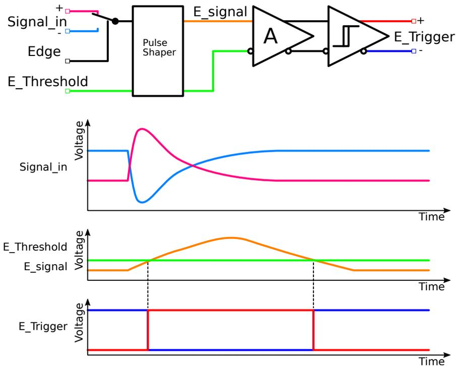
Figure 5.5: Diagram of a MuTRiG energy branch.
