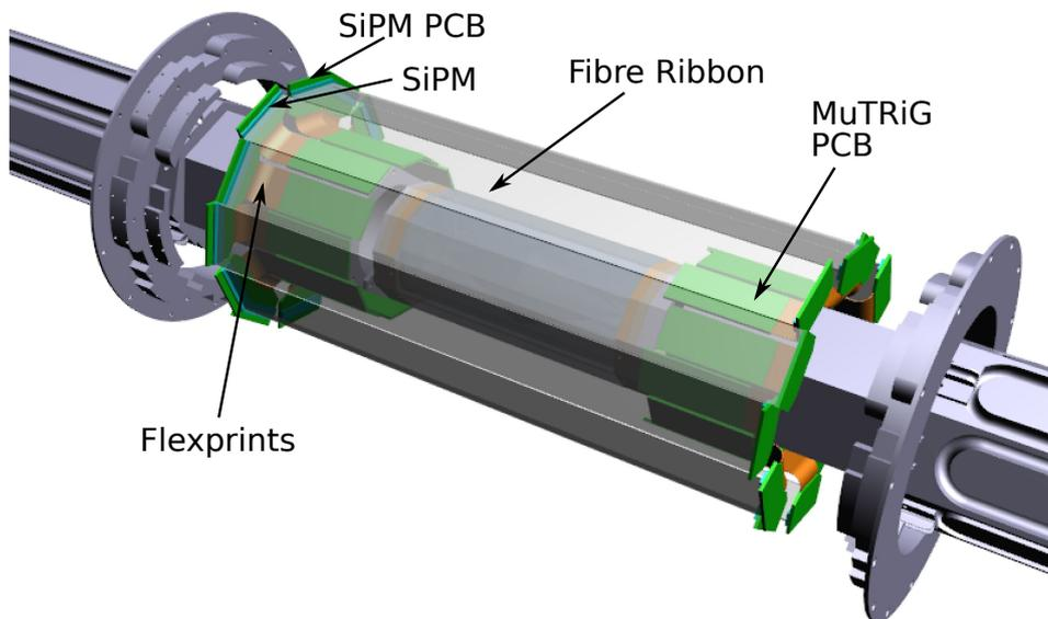
**Figure 2.13:** CAD drawing of the Mu3e fibre detector. Modified from [7].
