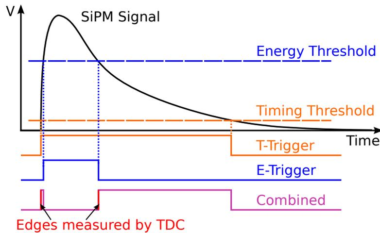
Figure 5.1: Trigger principle of the MuTRiG channel.
