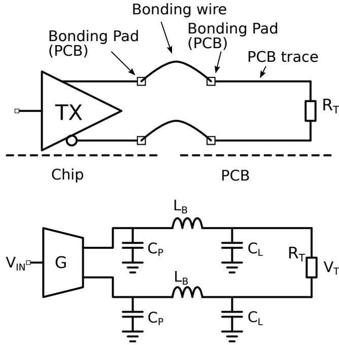
Figure 5.24: Distributed load model of the LVDS driver.
