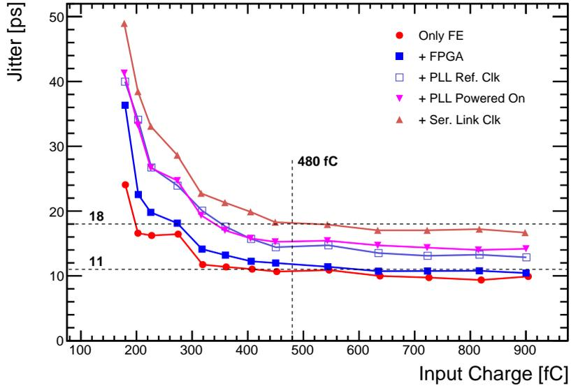
Figure 6.6: Front-end jitter measurement results.
