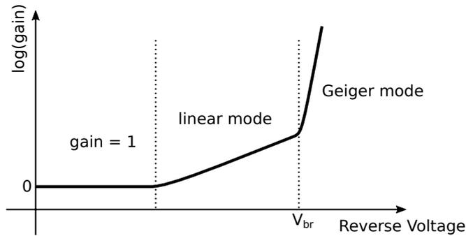
**Figure 3.4:** Gain of the APD in different reverse bias voltage.
