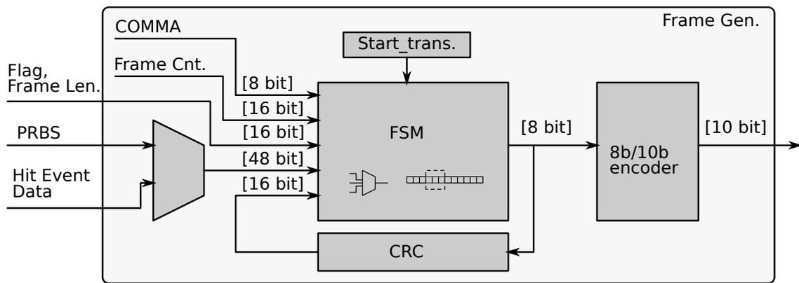
**Figure 5.16:** Block diagram of the frame generator unit.
