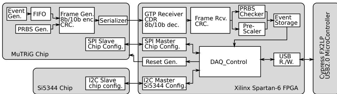
**Figure 6.4:** Logical Block of the DAQ firmware on FPGA. Related units in the MuTRiG and Si5344 chip is also shown.
