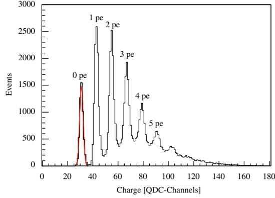
Figure 3.9: Single Photon Spectrum of a SiPM [63].
