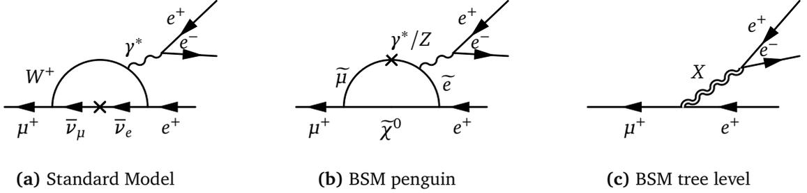
**Figure 2.1:** Feynman diagram for the lepton violation decay  $\mu \rightarrow eee$ . **(a)** The  $\mu \rightarrow eee$  decay via neutrino mixing in the Standard Model. **(b)** The  $\mu \rightarrow eee$  decay via penguin loop diagram involving new heavy particles in the super-symmetric models. **(c)** The  $\mu \rightarrow eee$  decay at tree level involving new particles in the models beyond Standard Model.
