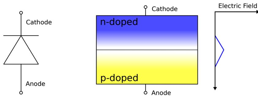
**Figure 3.1:** Circuit symbol, schematic structure and electric field distribution of a p-n junction.
