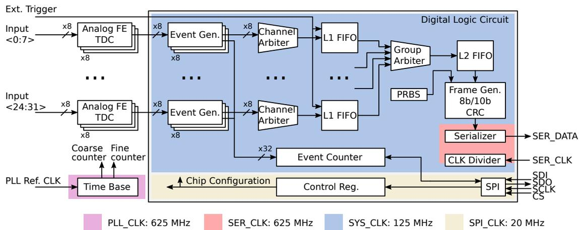
Figure 5.11: Block Diagram of the MuTRiG Chip.
