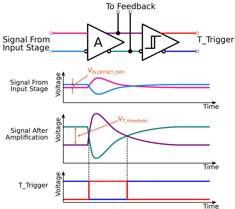
Figure 5.4: Diagram of a MuTRIG timing branch.
