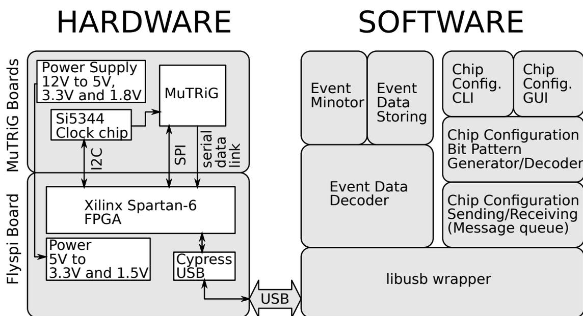
**Figure 6.3:** Overview of the MuTRiG characterization DAQ system.
