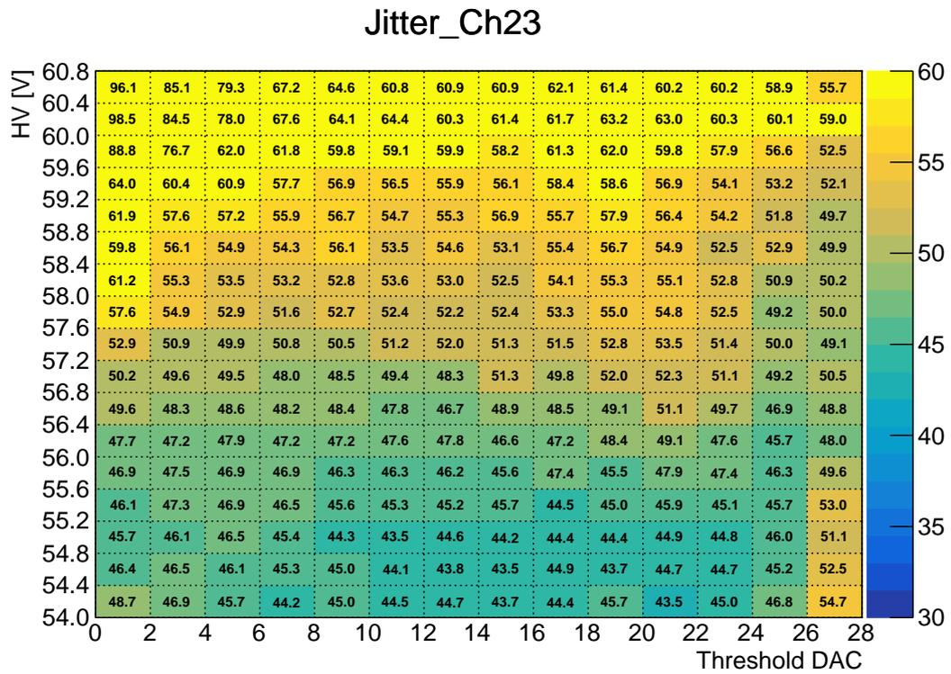
Figure 6.22: Timing resolution of channel 23 at all the test configuration.
