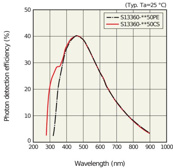
**Figure 3.10:** PDE vs. wavelength characteristic of the Hamamatsu S13360 series MPPC with 50  $\mu\text{m}$  pixel pitch [64].
