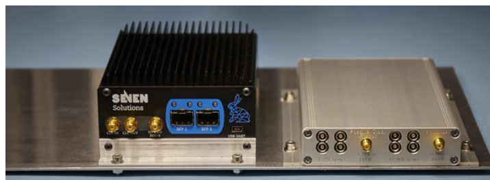
Figure 3.14: Picture of the WR LENO and the fanout (credit: Felix Werner).
