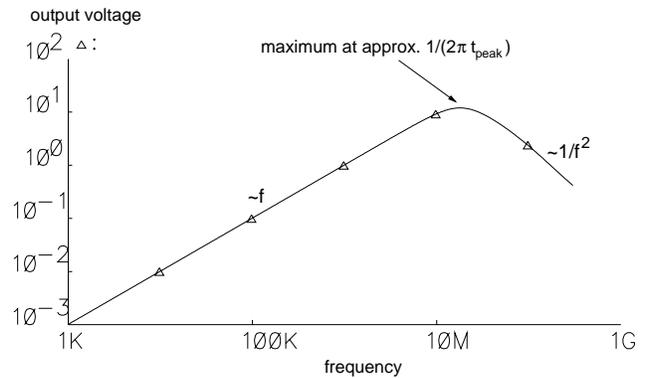
Figure 5: Frequency response of the pulse shaping stage
