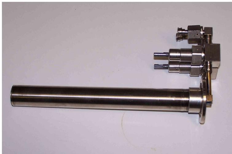
**Figure 6.2 :** *Sample container. At the top the VCR fittings and the valves can be seen. At the right, the flange by which the sample container can be attached to the sampling dewar is visible.*
