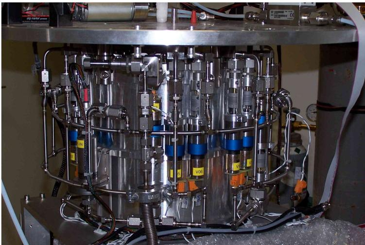
**Figure 6.6 :** *Balloon sampler. One can see the inlet and outlet manifolds with attached stubs and bellows. Further, the motors and couplings to the valves of the sample containers can be seen.*
