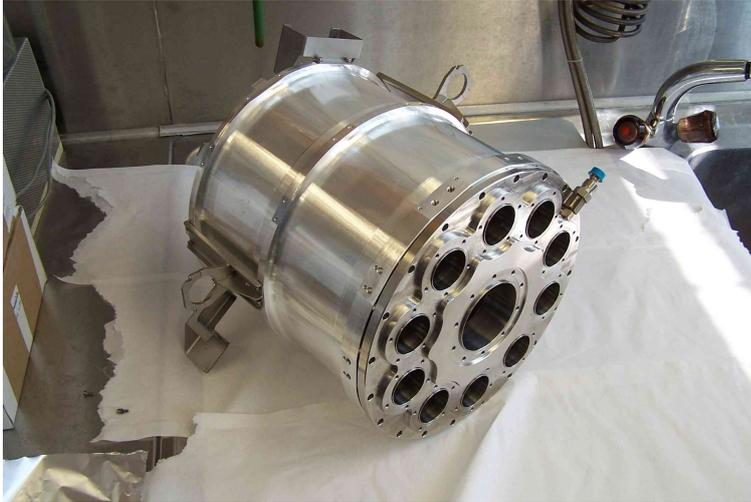
**Figure 6.3 :** *Main dewar with no sample containers attached.*
