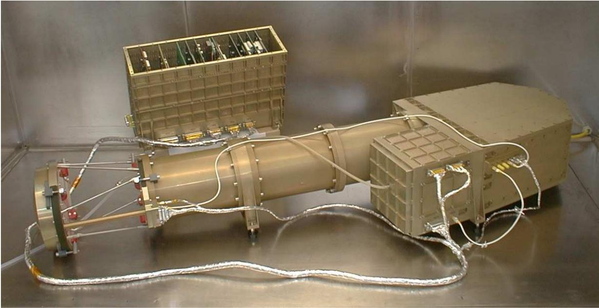
Figure 1.4: Cometary and Interstellar Dust Analyzer (CIDA). Time-of-flight mass spectrometer with high mass resolutions ( $m/\Delta m \geq 150$ )
