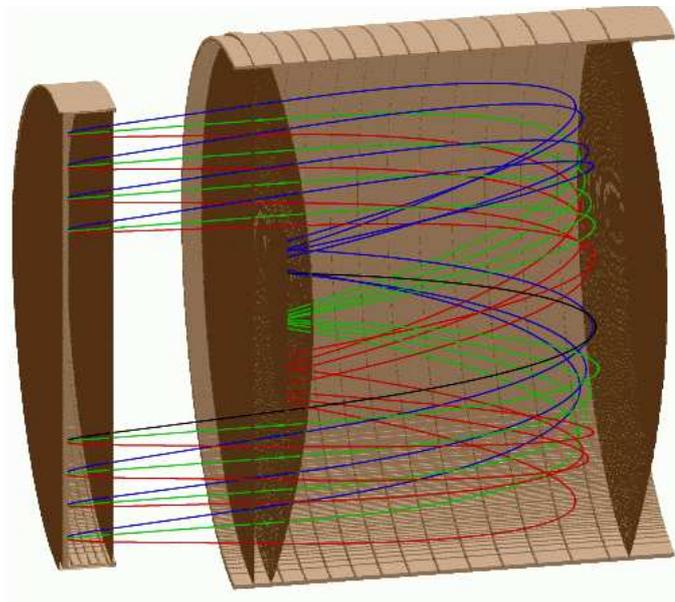
Figure 1.5: Large-Area Mass Analyzer (LAMA). Left: Impact target and acceleration grid. Right: Reflectron with two parabolic grids and potential rings at the side wall. In between the two units, a field-free region allows the integration of the trajectory sensor module. The colored lines represent ion trajectories for different initial conditions.
