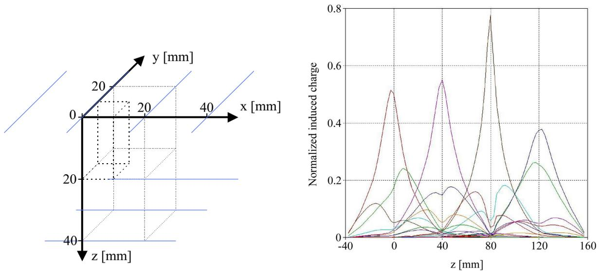
Figure 2.3: EM simulation of the detector signals for a typical trajectory. Left: Choice of the coordinate system. The sensor planes are located at  $z = 0, 40$  mm,  $80$  mm and  $120$  mm ( $80$  mm and  $120$  mm not shown). Right: Transient signals of a typical particle trajectory. Amplitudes are plotted as fractions of the particle charge.
