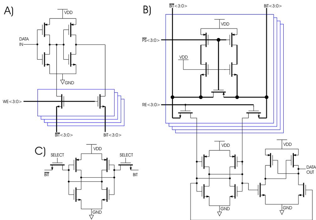
Figure 3.18: Pipeline components. The circuit parts highlighted with blue boxes are implemented fourfold in parallel. A) Input amplifier. B) Output amplifier. C) Memory cell.
