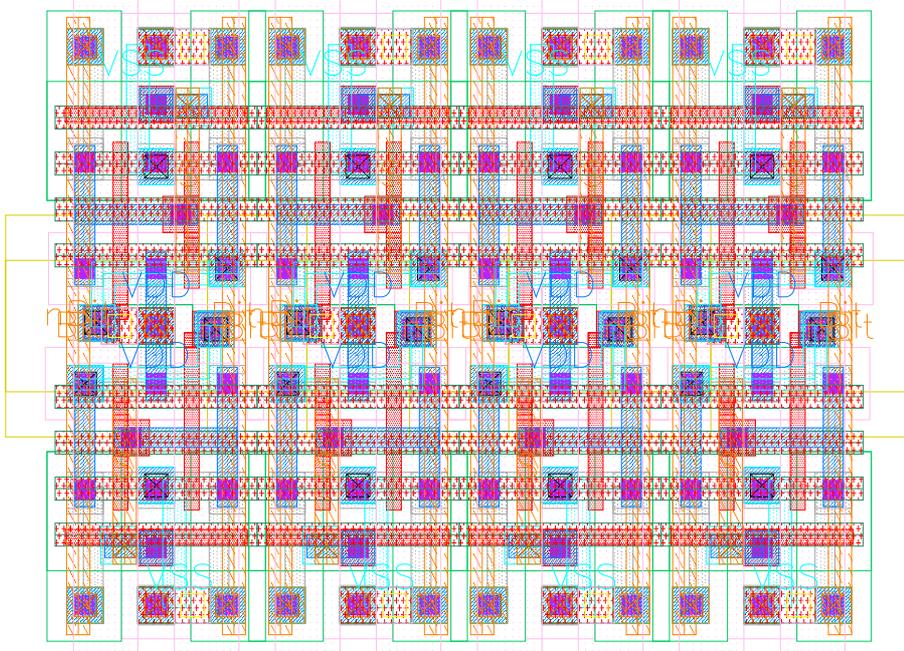
Figure 3.17: Layout of a 8 bit memory cell array unit. Four select lines (red crossed horizontal bars) have to be implemented per memory row to achieve the sub-column architecture.
