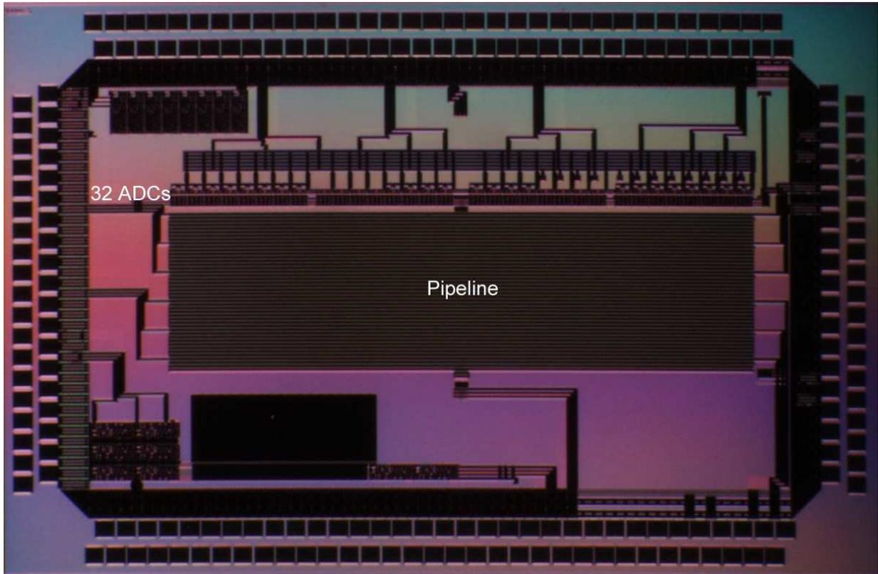
Figure 2.7: DUNE 1.0 chip photograph. Front-end amplifier unit (bottom left) and 32-channel transient recorder (center) with 10 bit resolution. Chip size: 5 mm  $\times$  3.3 mm. The two units can be powered and operated independently.
