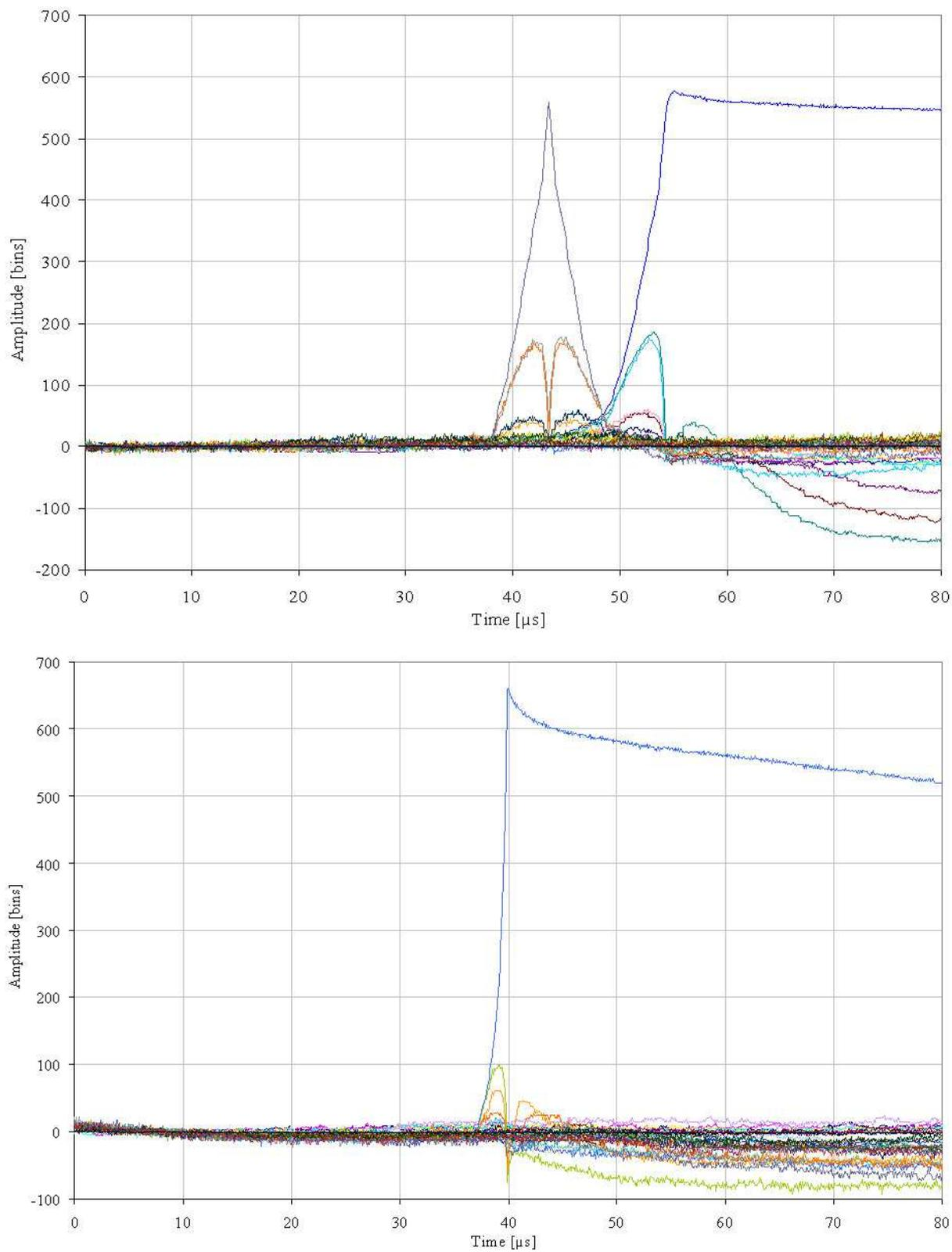
Figure 4.14: Wire Impacts. Top: Impact on second sensor plane. The first plane shows the signal shape typical for trajectories close to a wire. Bottom: Impact on the first plane.
