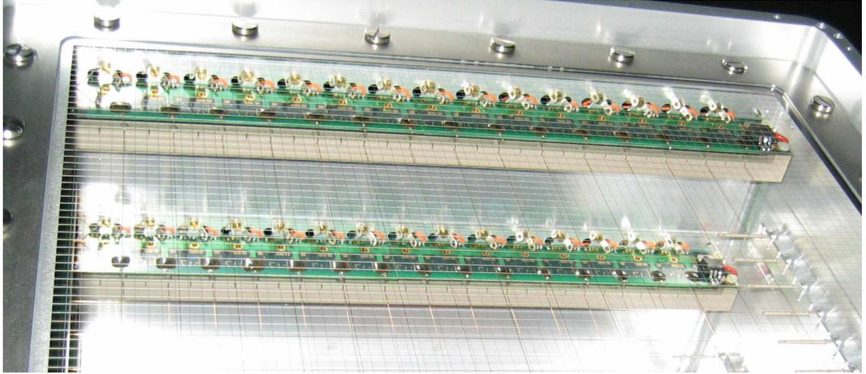
Figure 4.2: Detector inside. 30 front-end ASICs are bonded onto two detector boards and covered with glob top for protection. Ground connections between shield and boards are provided all 20 mm.
