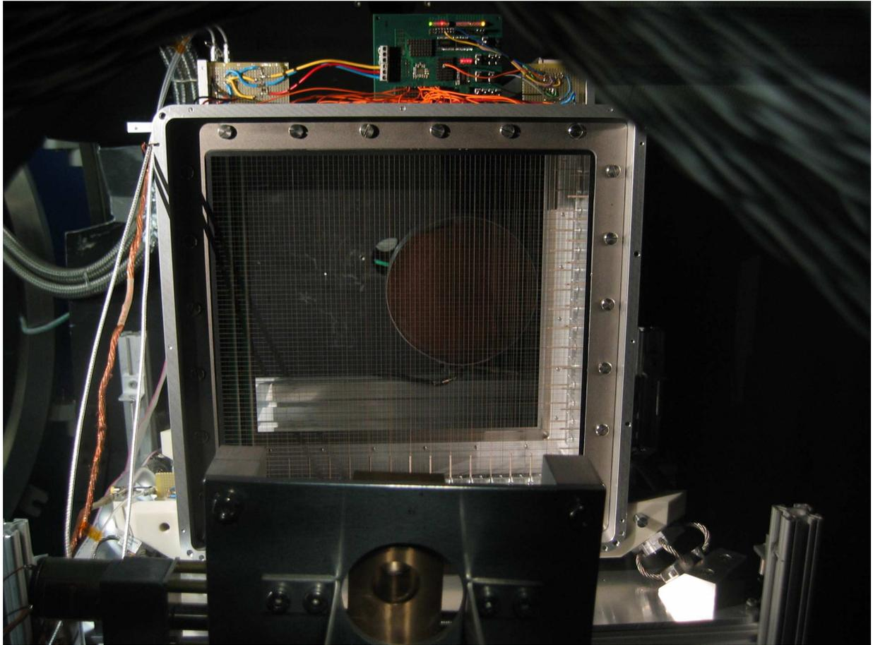
Figure 4.12: Dust accelerator setup. The detector is equipped with 31 microchips (30 front-end amplifiers and one transient recorder). In order to achieve a precise beam focus, the dust beam is sent through a slit aperture (front). The trajectory sensor is triggered by an impact target at the backside of the detector (round copper plate).
