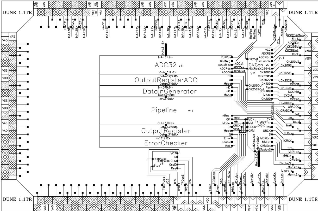
Figure 3.8: DUNE 1.1TR top-level schematic and pad assignment. The 32 analog inputs  $InA< 31 : 0 >$  are routed to the 32 ADCs (ADC32). The 320 bit wide data stream is then stored in the pipeline. The output register is controlled by the trigger logic and serializes the parallel data stream on readout.
