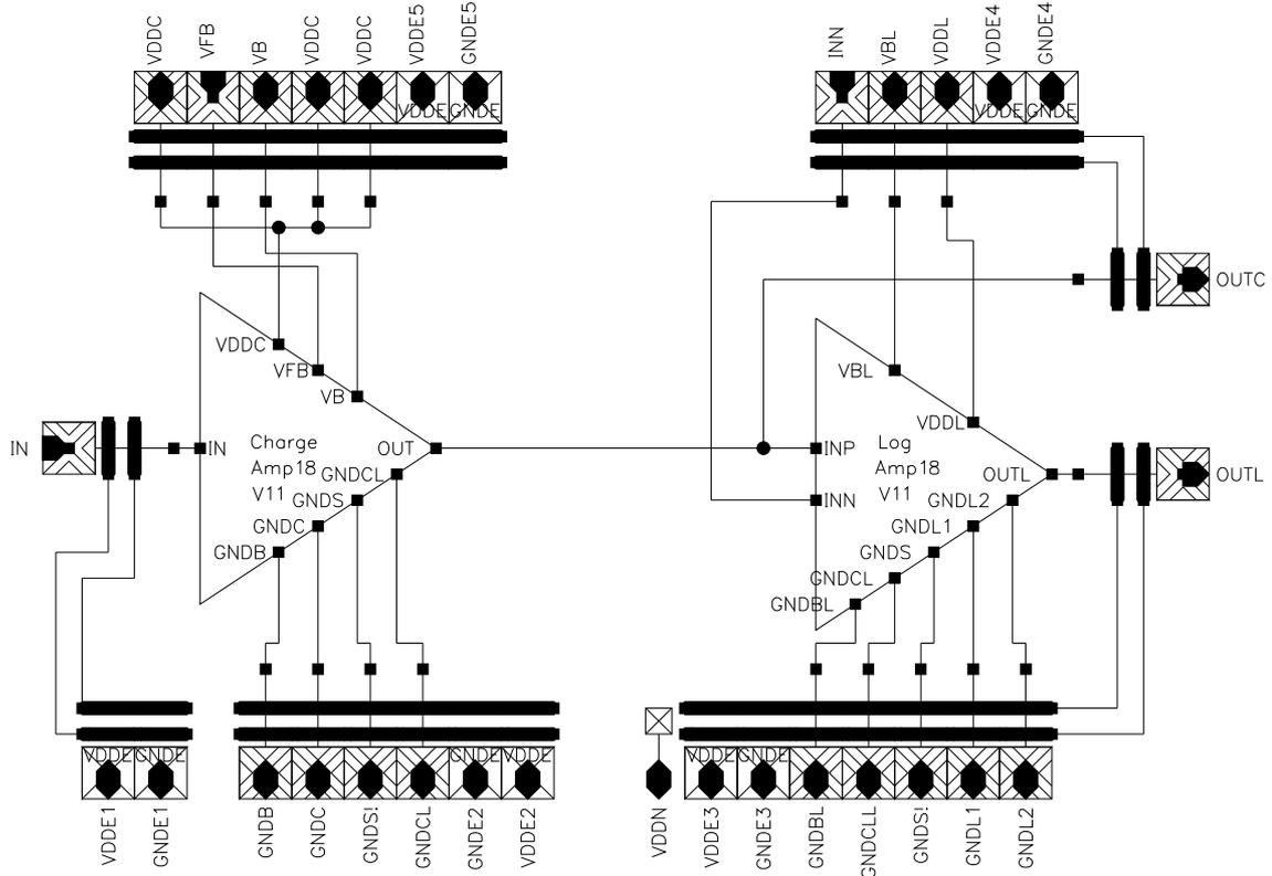
Figure 3.3: DUNE 1.1FE top-level schematic and pad assignment. The noninverting input (INP) of the logarithmic amplifier is connected to the charge sensitive amplifier, while the inverting input (INN) is provided by an external feedback circuit.
