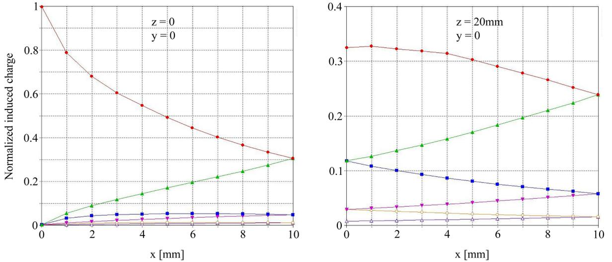
Figure 2.4: Distance function of induced charge signals for characteristic particle locations. Left: Particle position in the first sensor plane ( $z = 0$ ). Amplitudes are plotted as functions of  $x$ , the distance to the closest wire. Right: Particle position between first and second sensor plane ( $z = 20$  mm).
