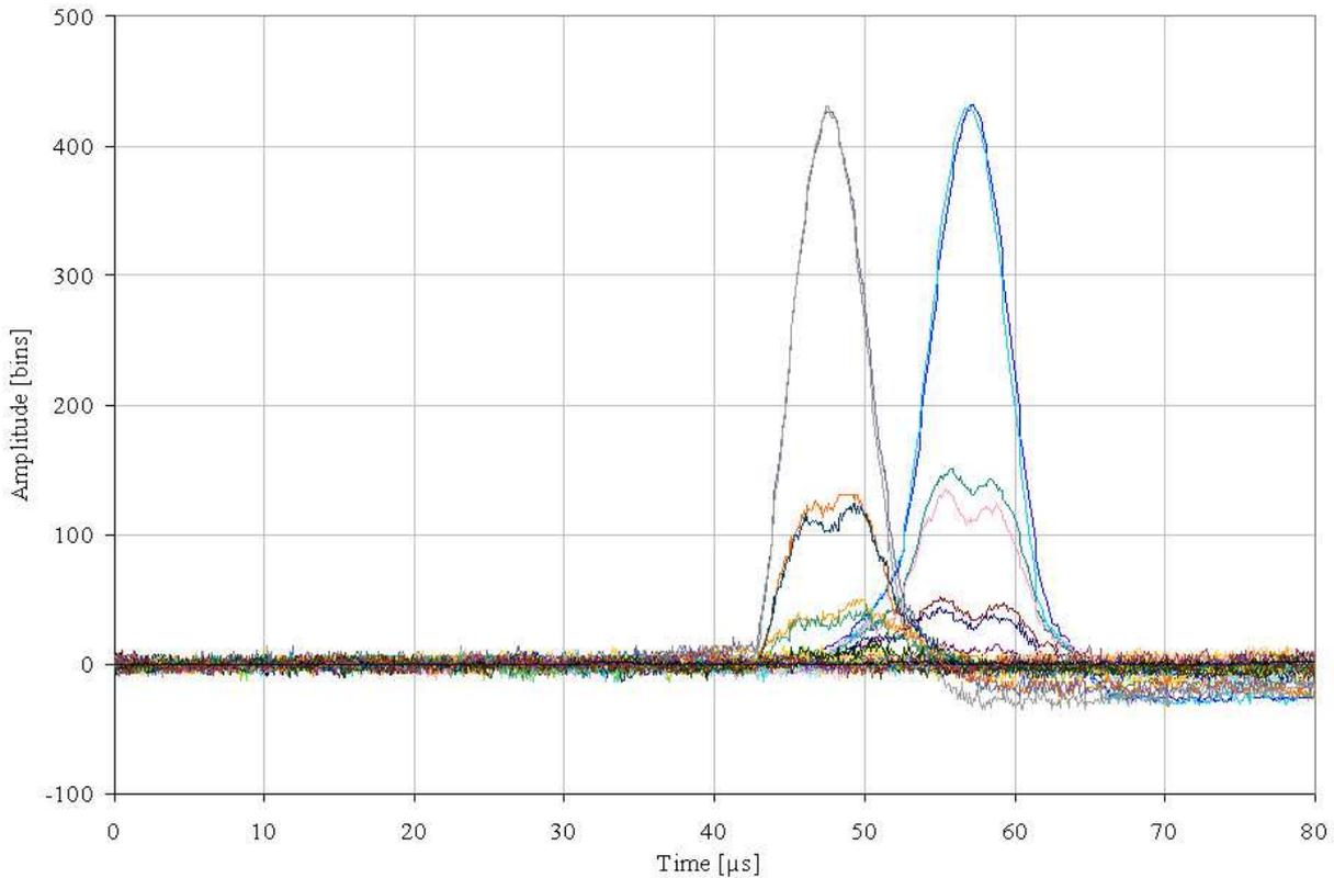
Figure 4.13: Typical charge signals of a dust particle ( $Q = 2.2$  fC,  $v = 8$  km/s).
