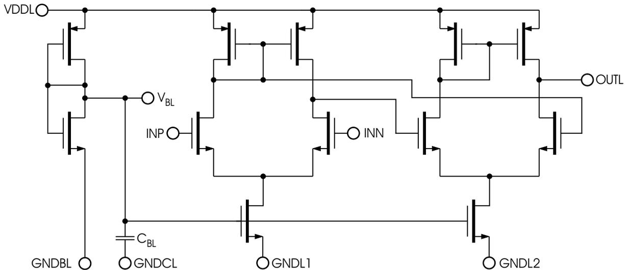
Figure 3.5: Logarithmic amplifier. Series of two differential amplifiers with on-chip biasing. The charge sensitive amplifier is connected to INP. External access to the inverting input (INN) enables the implementation of a feedback circuit for control of the operating point and stabilization of the baseline.
