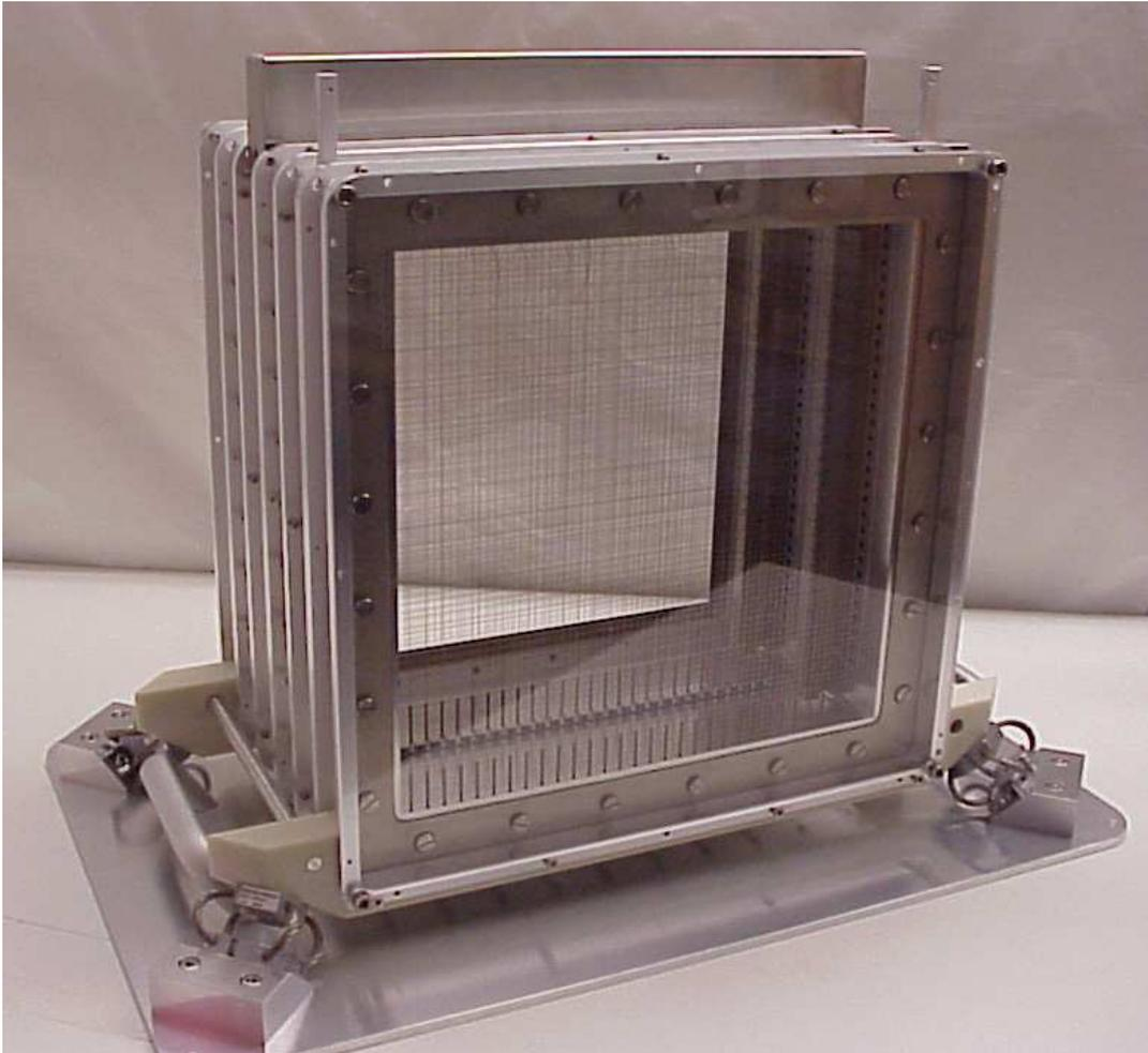
Figure 2.1: DUNE trajectory sensor. The detector consists of six stacked frames. The outer frames are shielding grids, the inner four are equipped with sensor wires. Wires of adjacent sensor planes have a perpendicular orientation with respect to each other. The spacing of the frames is 40 mm.
