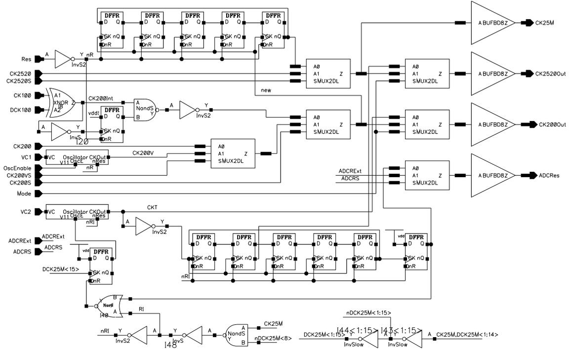
Figure 3.22: Schematic of the clock generator. Synchronized clock signals for the ADCs and the memory are produced by a voltage controlled oscillator (VCO). Optionally, the clocks can be provided externally.
