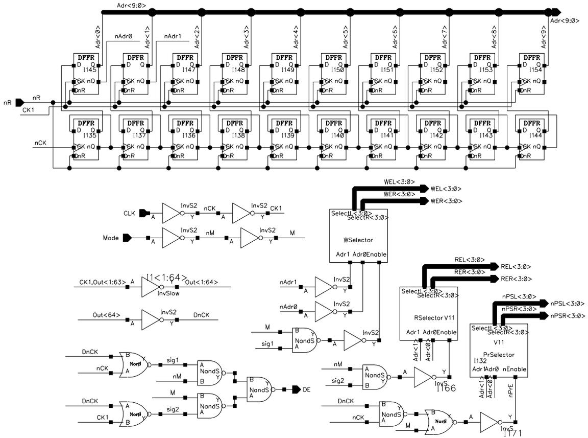
Figure 3.20: Pipeline Controller schematic. A 10 bit counter with output register generates a synchronous address signal. The two LSBs of the address (nAdr0 and nAdr1) are decoded internally to provide the sub-column information. The decoder enable signal (DE), the read and write enable signals (REL, RER, WEL, WER) and the precharge select signal (nPSL, nPSR) are produced by this unit.
