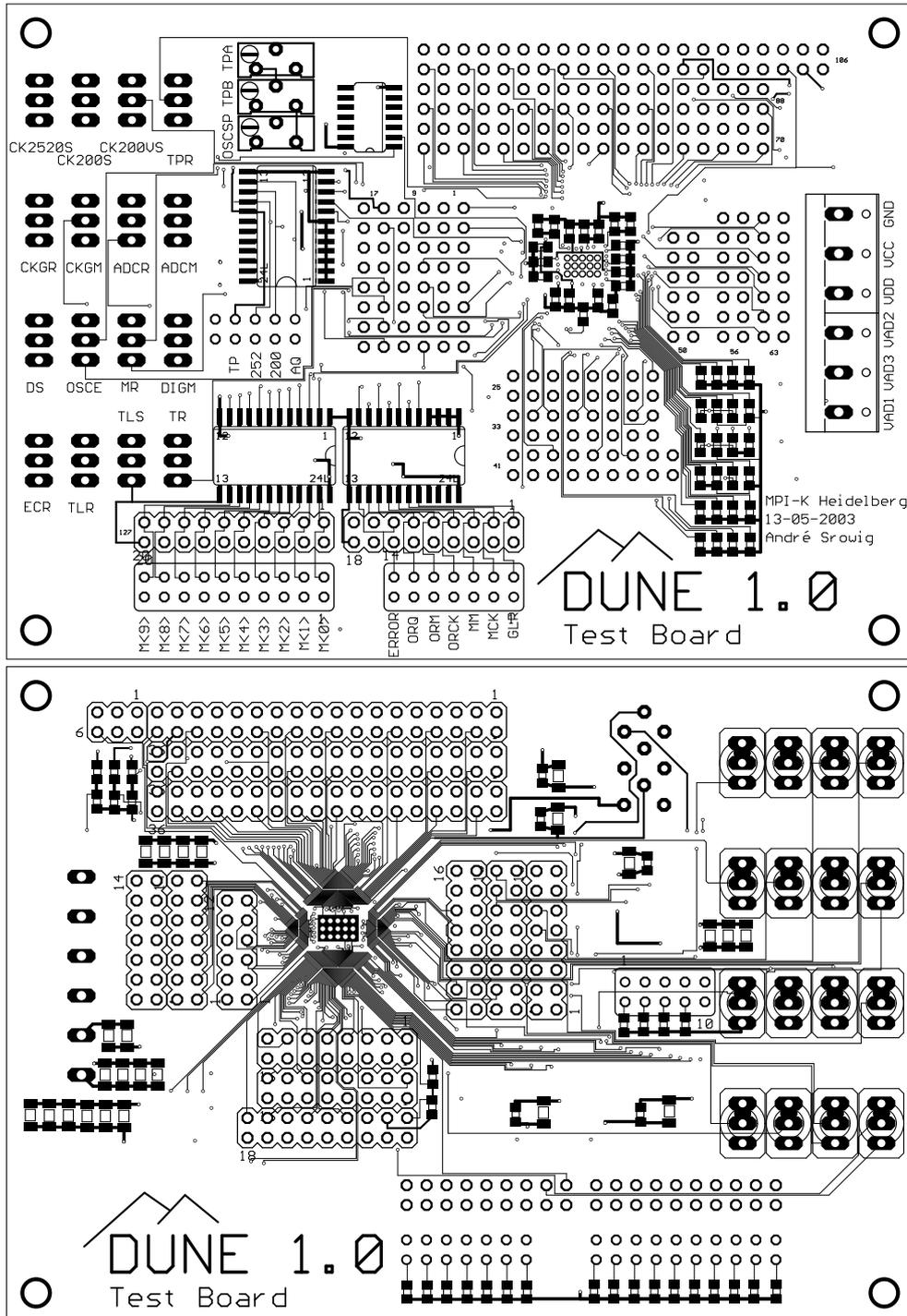
Figure 4.3: DUNE 1.0 test board with chip-on-board technology. The bond wire pitch is  $60\ \mu\text{m}$ . 16 switches and 21 LEDs enable simple control and testing of the circuit. Since the pad layout of DUNE 1.1TR and DUNE 1.0 are identical, the test board could be utilized for the detector assembly.
