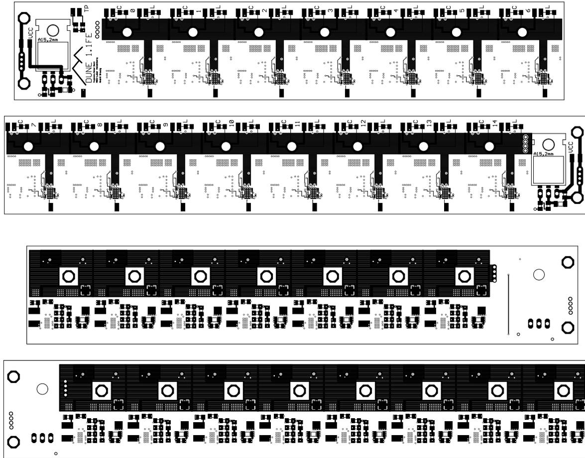
Figure 4.1: DUNE 1.1 detector board. The printed circuit board is a four-layer design with shielded output lines. Chip-on-board technology is applied. Filter components are placed on the backside of the board.
