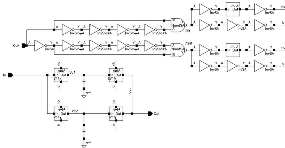
Figure 3.15: Schematic of the sample & hold unit. Interleaved sampling structure with non-overlapping differential clock generator. While one capacitance is charged to the input voltage, the other provides its potential to the comparator. The transmission gates are charge injection compensated.
