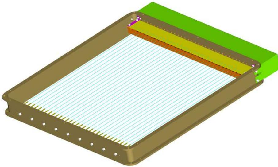
Figure 2.2: Sensor plane. Active area is  $300\text{ mm} \times 300\text{ mm}$ . Up to 31 wires can be mounted with a spacing of  $10\text{ mm}$ . The nominal configuration consists of 16 wires ( $20\text{ mm}$  spacing). Mounts have been provided for the circuit boards carrying the readout electronics.
