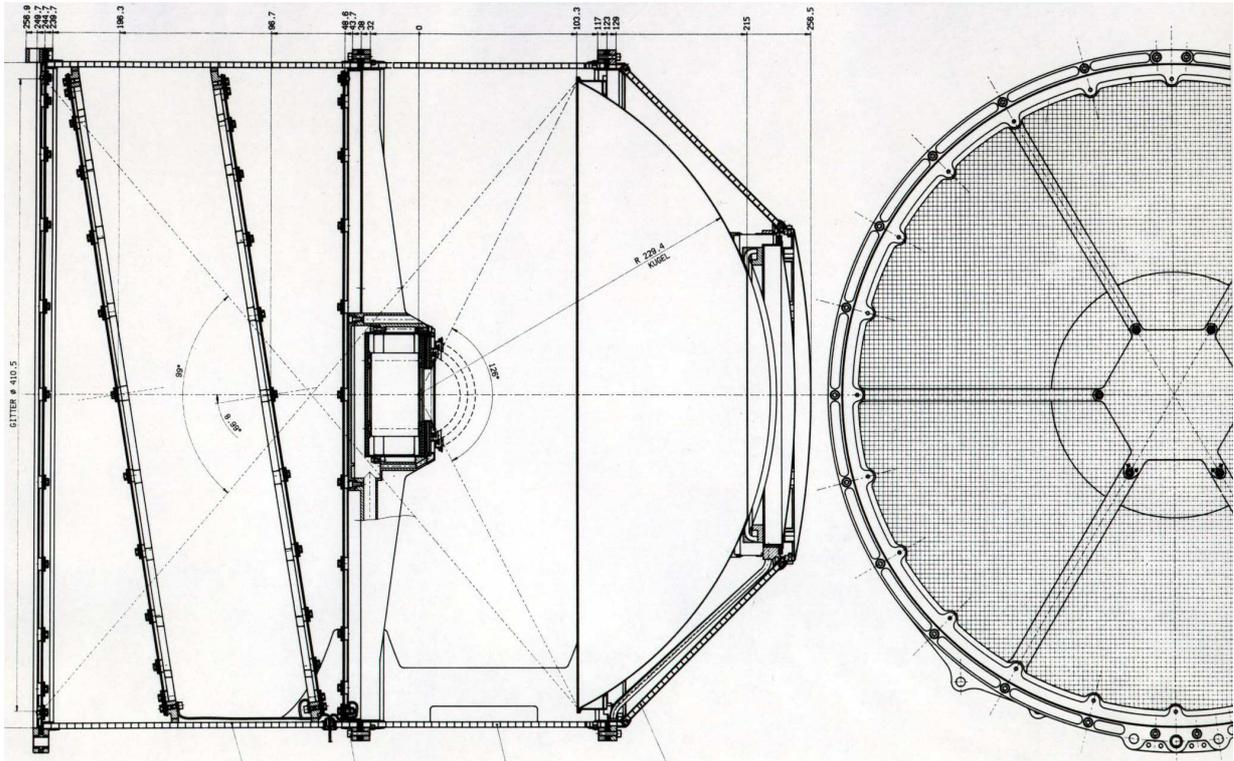
Figure 1.3: Cassini Cosmic Dust Analyzer (CDA). The charge sensor consists of two shielding grids and two tilted sensor grids. Both sensor electrodes are connected to one charge sensitive amplifier. From the signal shape of a particle measurement a rough estimate of the trajectory can be gained.
