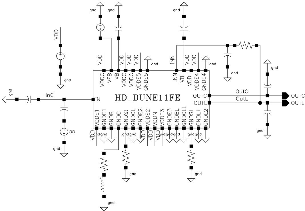
Figure 3.6: Simulation environment and external setup. The current source of the folded cascode is connected to ground via a  $100 \mu\text{H}$  inductance (GNDC) in order to reduce flicker noise of the cascode current source. Its series resistance of  $5 \Omega$  has been considered in the optimization. The low-pass feedback from OUTL to INN forms the baseline stabilization circuit.
