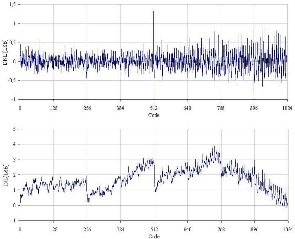
Figure 4.8: DNL and INL of the ADC with activated range controller. Input voltage range is 0 .. 1.4 Volts. The INL is dominated by mismatch of the R-2R DAC resistors determining the MSBs.
