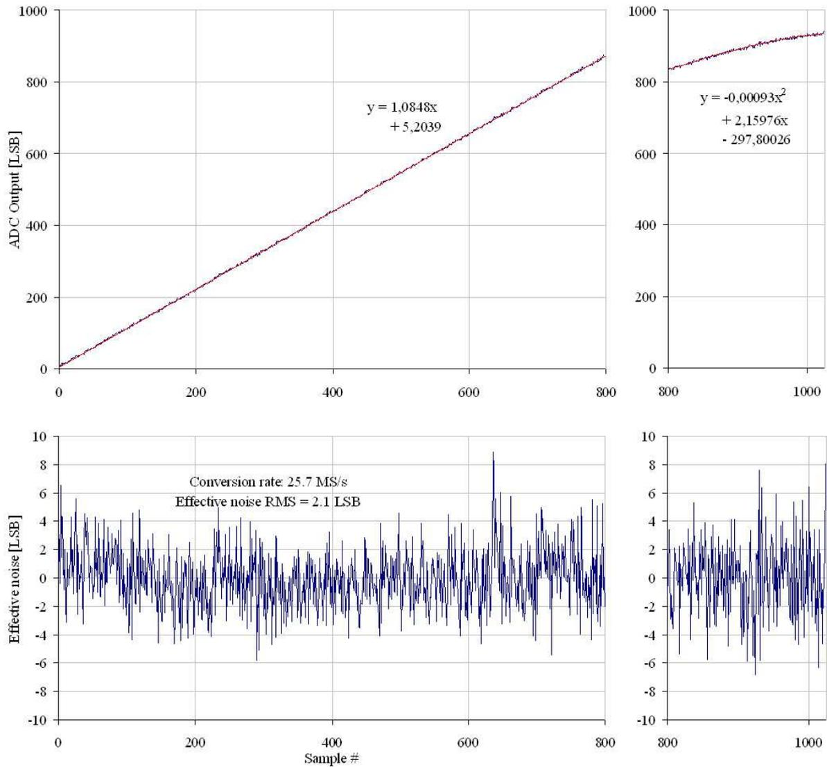
Figure 4.6: ADC linearity and effective noise. Left: Linear fit to a typical channel. Right: Quadratic fit to the worst case channel at the upper rail.
