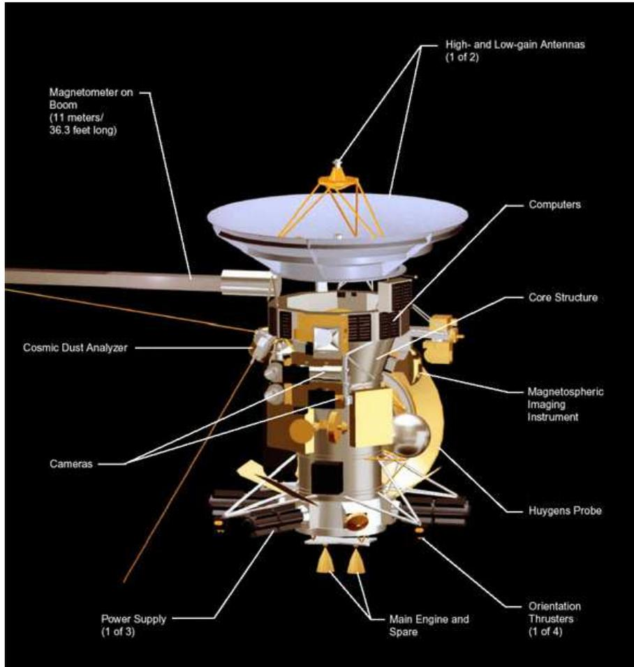
Figure 1.2: Cassini spacecraft. Launched from Kennedy Space Center on October 15, 1997, the Cassini-Huygens spacecraft reached the Saturnian region in July 2004. The mission is composed of two elements: The Cassini orbiter that will orbit Saturn and its moons for four years, and the Huygens probe that will dive into the atmosphere of Titan and land on its surface.
