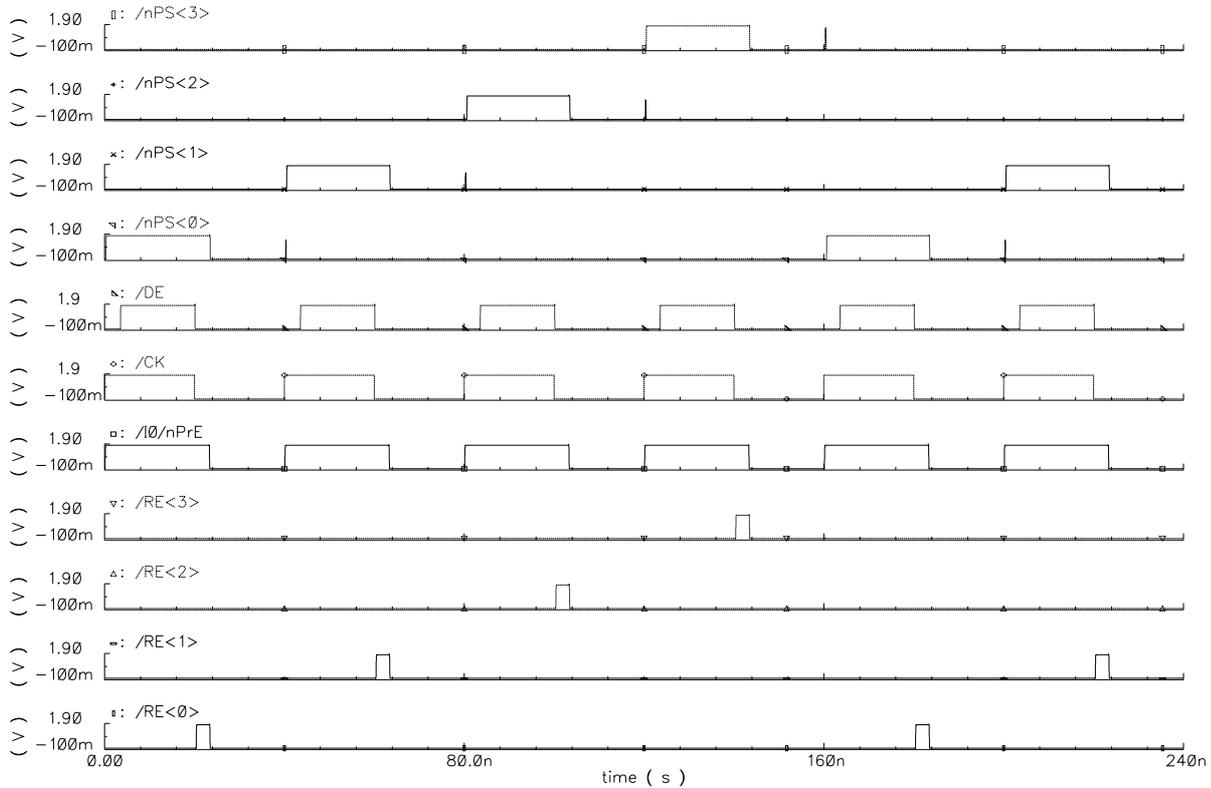
Figure 3.21: Simulation of the pipeline controller in read operation. From top to bottom: Precharge select signals ( $nPS<3:0>$ ; active low), decoder enable signal (DE), memory clock (CK), precharge enable ( $nPrE$ ; internal signal that is propagated to one of the sub-channels by the precharge selector), read enable ( $RE<3:0>$ )
