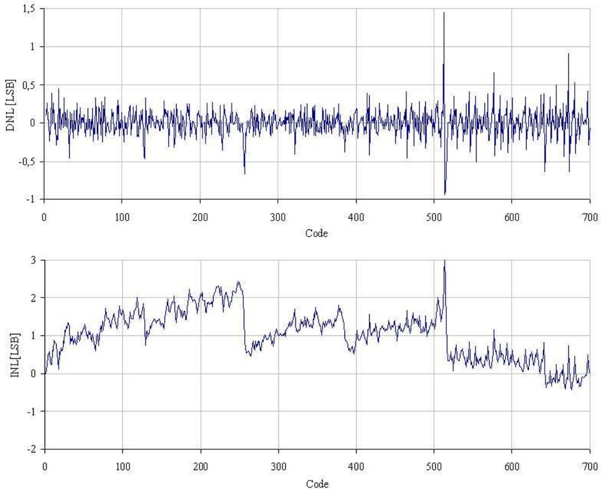
Figure 4.7: DNL and INL of the ADC in the DUNE operating range.
