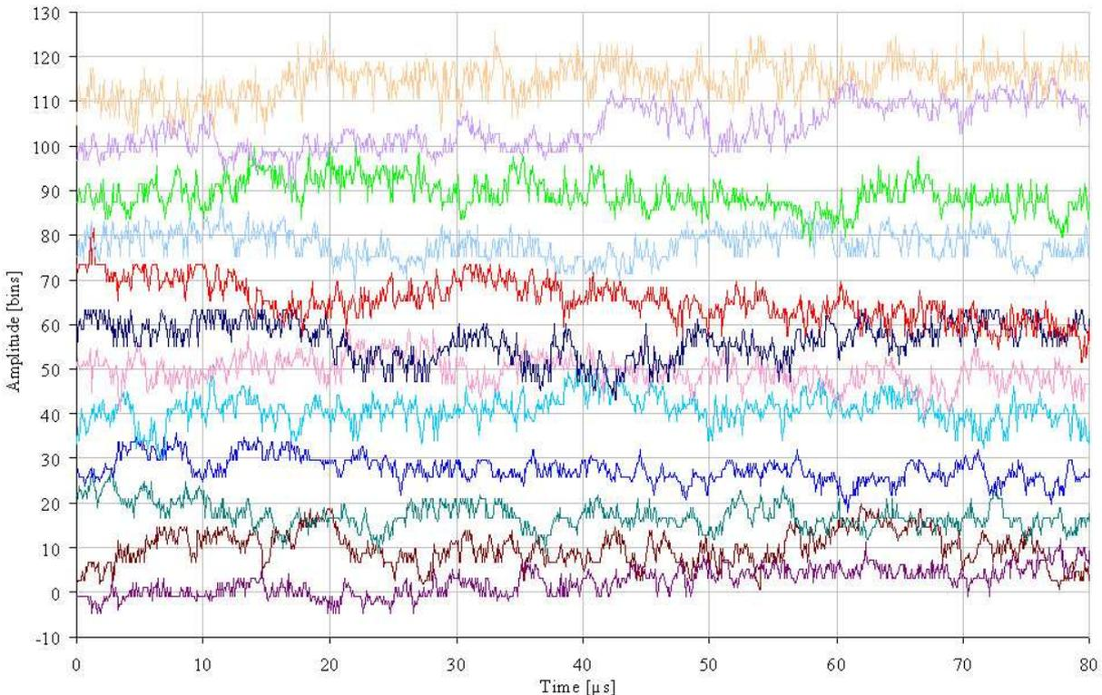
Figure 4.15: Total noise of the DUNE 1.1 readout chain on channels 5 .. 16. The RMS values range from 2.9 LSB to 4.9 LSB. The average RMS value is 3.7 LSB.
