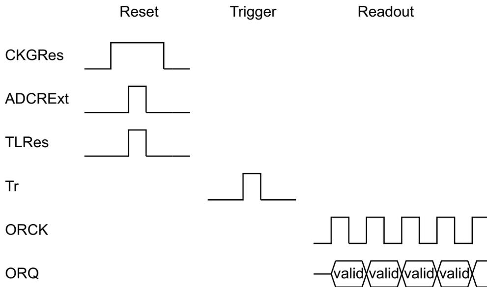
Figure 4.4: DUNE 1.1 control sequences. After reset, the system is in recording mode. A trigger signal stops the recording, so data can be read out.  $2^{19}$  clock pulses have to be sent to the output register (ORCK), in order to read out the complete memory.
