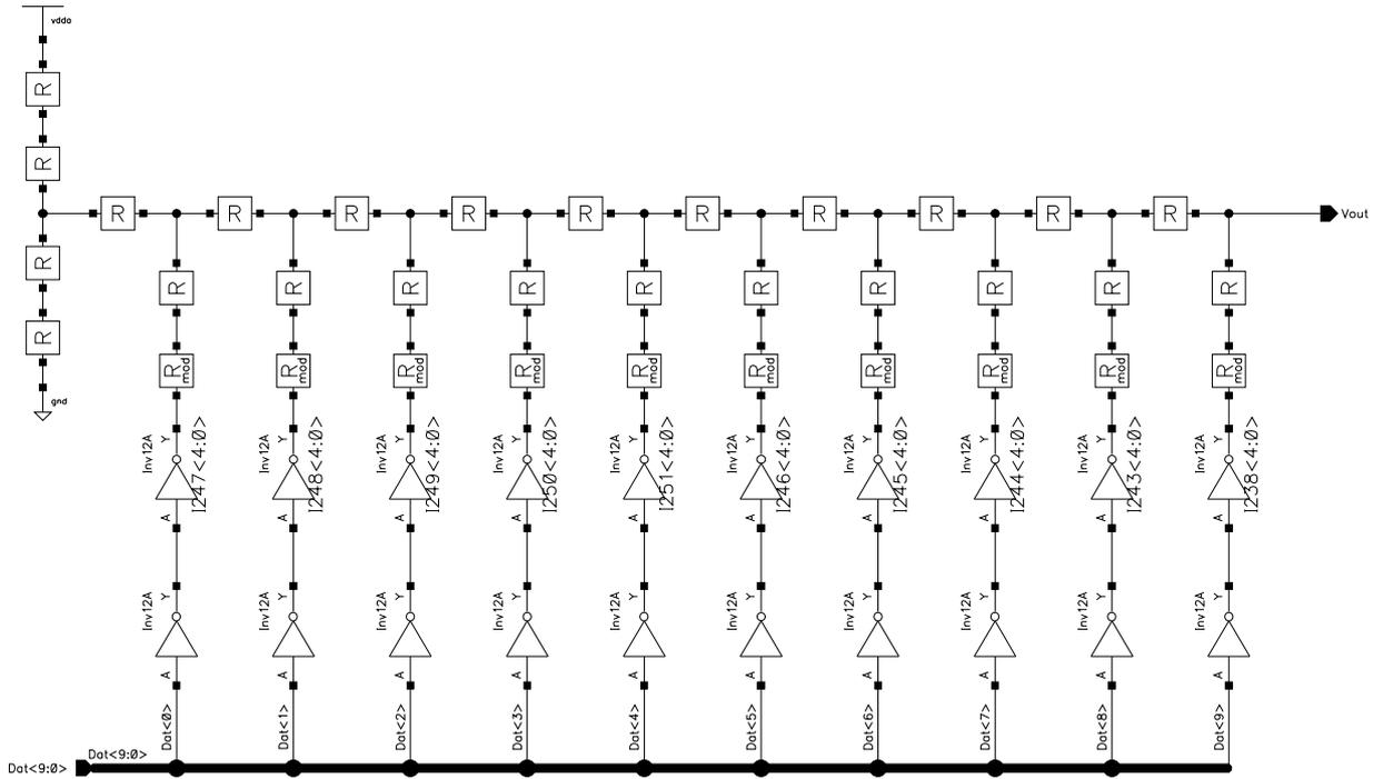
Figure 3.13: DAC schematic. The R-2R resistor ladder is driven by inverters. The resistors directly connected to the drivers are slightly smaller than  $R$  in order to account for the driving impedance of the inverters.
