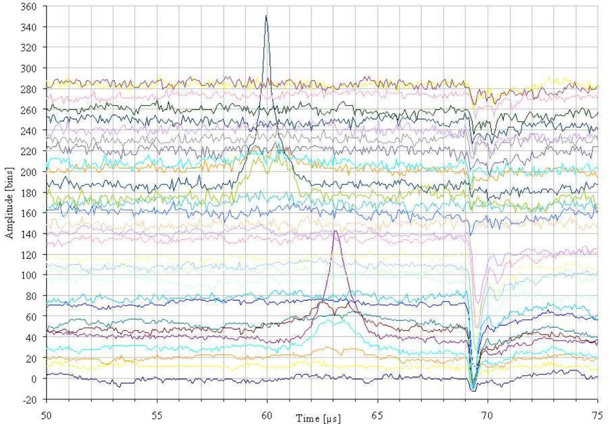
Figure 4.16: Small particle. The speed of this dust grain was 27 km/s, and it carried a charge of only 0.9 fC. The signal-to-noise ratio of the dominant signal is 45. On impact, fast ejectors of opposite polarity were repelled and produced additional signals, mainly on the second sensor plane.
