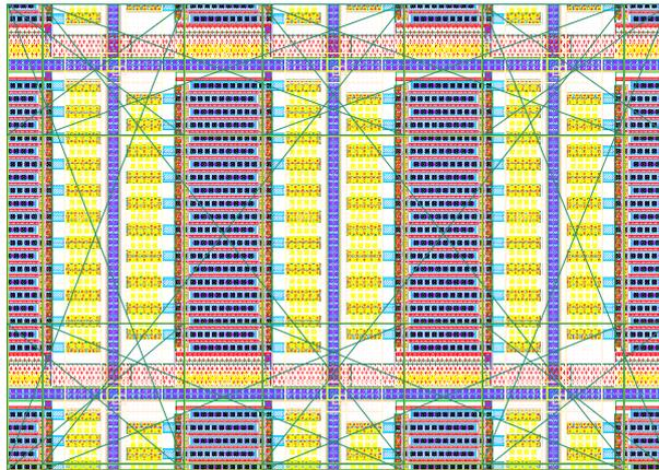
Figure 3.1: Low noise RF transistor array. Multi-finger layout assures a small gate resistance. Guard rings keep the substrate ground stable.
