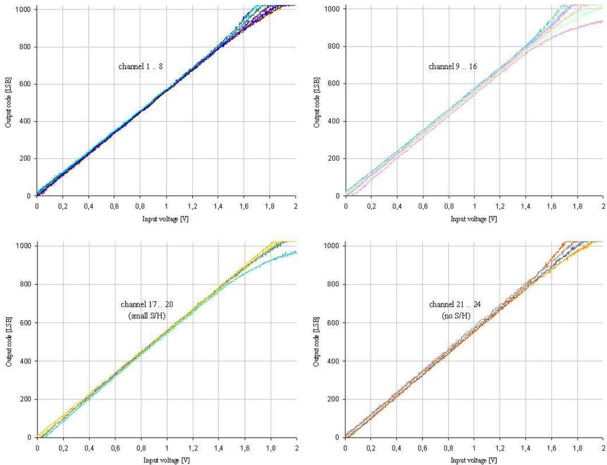
Figure 4.5: ADC rail-to-rail sweep at 25.7 MS/s conversion rate. 1024 samples per channel are recorded.
