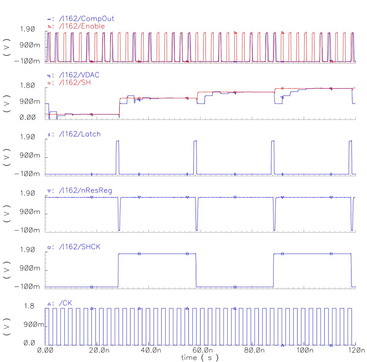
Figure 3.11: Simulation of the ADC. From top to bottom: comparator output and enable signal steering the SAR register, sample & hold voltage and approximating DAC reference voltage, output latch signal, register reset signal, sample & hold clock, ADC clock.
