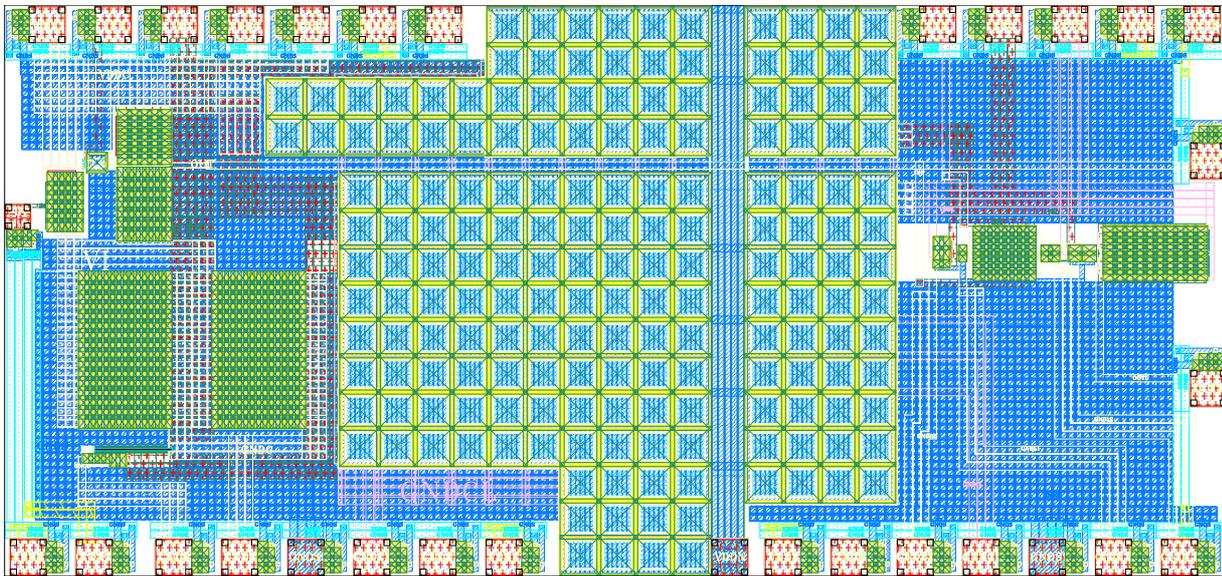
Figure 3.2: Layout of DUNE 1.1FE. The die size is  $3.3 \text{ mm} \times 1.6 \text{ mm}$ . Left: Charge sensitive amplifier. Center: Decoupling capacitances, Right: Logarithmic amplifier.
