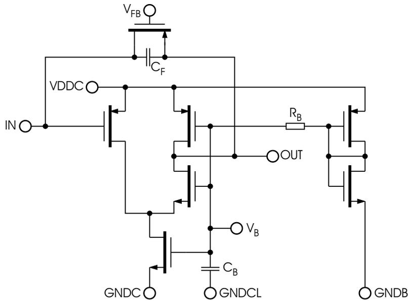
Figure 3.4: Charge sensitive amplifier. Folded cascode amplifier with capacitive feedback and on-chip biasing.
