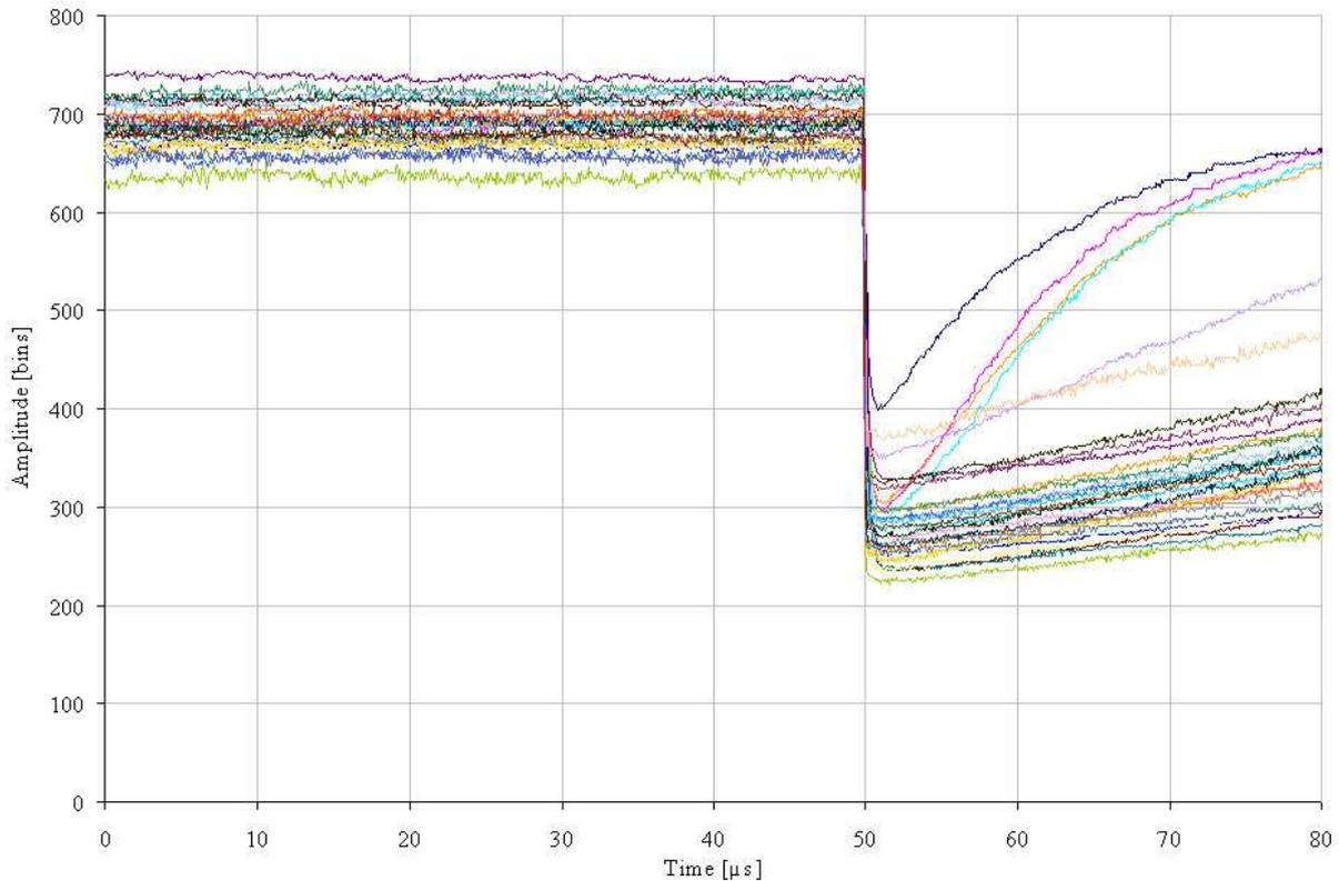
Figure 4.9: Test pulse transient signal. Channels 1 .. 4 (dark blue, red, yellow and light blue curve) are filtered stronger than the other at the low band edge. Hence, their baselines recover faster.
