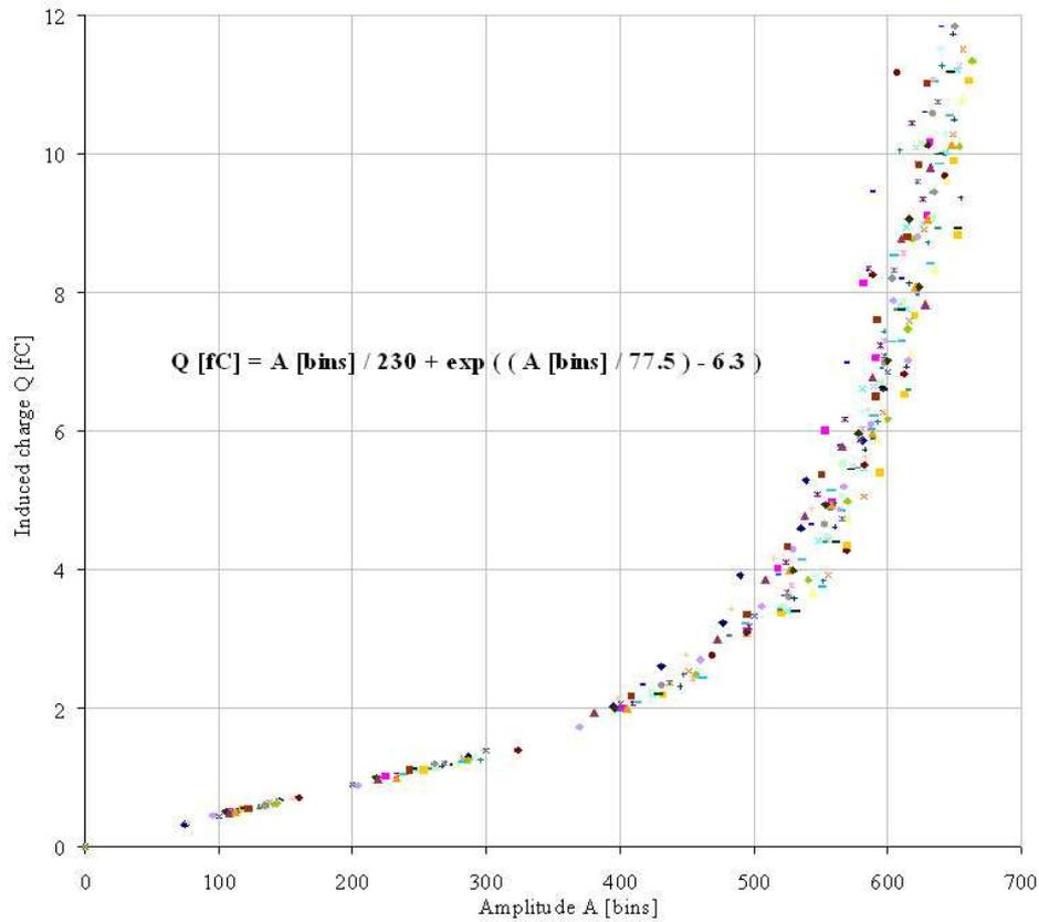
Figure 4.10: Logarithmic amplification. The conversion gain in the linear range is 230 bins/fC.
