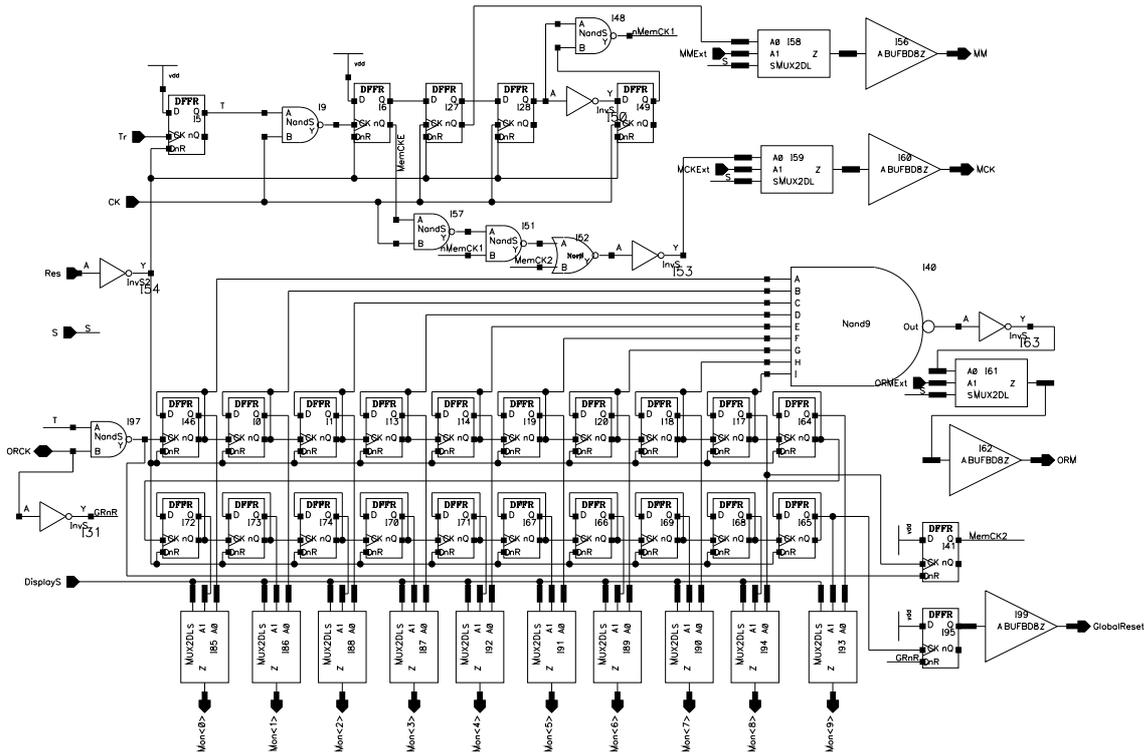
Figure 3.23: Schematic of the trigger logic. This unit controls the read and write operation of the transient recorder. During readout, it gates the 25 MHz memory clock (CK) and reacts on the external output register clock (ORCK). A 20 bit counter keeps track of the number of bits readout. Its state can be displayed via the status bits  $\text{Mon}\langle 9 : 0 \rangle$ .
