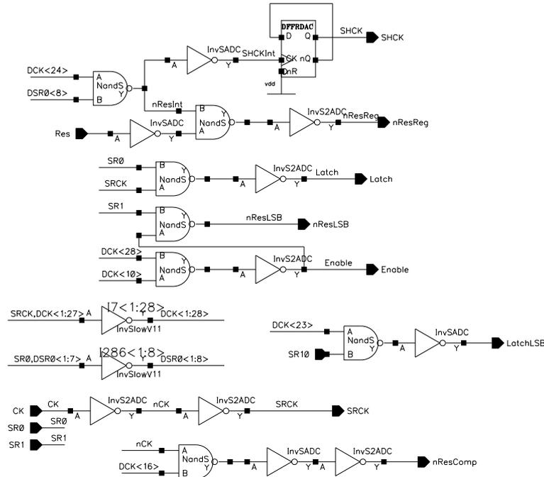
Figure 3.14: ADC controller schematic. From the 250 MHz ADC clock (CK) the S/H clock (SHCK), internal reset signals (nResReg, nResLSB and nResComp) and output latch signals (Latch, LatchLSB) are generated. The last two stages of the ADC shift register are connected to the controller (SR0, SR1). They indicate the last two cycles of the conversion and provide timing information for latching and reset.
