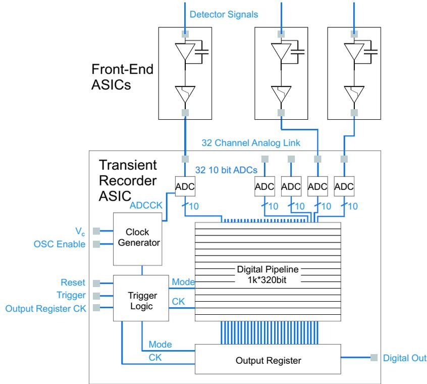
Figure 2.5: DUNE readout electronics block diagram. Individual front-end ASICs are connected to a 32 channel transient recorder ASIC. The analog signals are converted by ADCs at a conversion rate of 25 MS/s. The digital data is stored in a pipeline for 40  $\mu$ s and can be read out on a trigger event.
