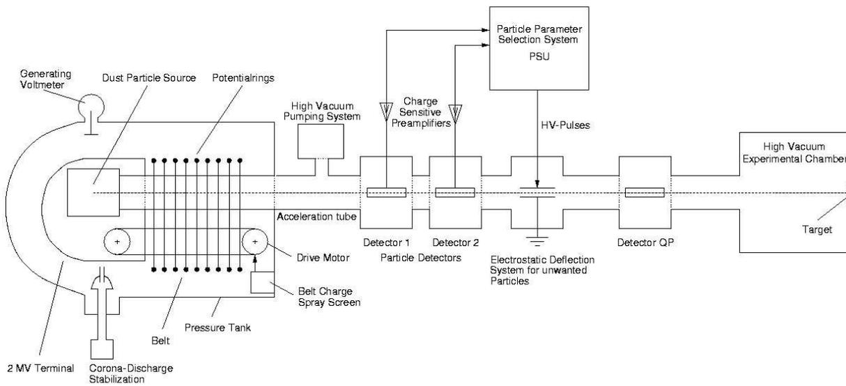
Figure 4.11: Dust accelerator with particle selection unit (PSU) and experimental chamber.
