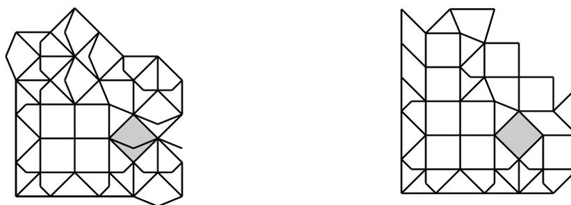
Figure 3.18. On the left: part of the the plane projection of a muqarnas vault in a shrine at Bisṭām (see Section 5.2.2). On the right: the plane projection of a muqarnas vault in a niche at the Friday Mosque in Natanz (see Section 5.2.1).
