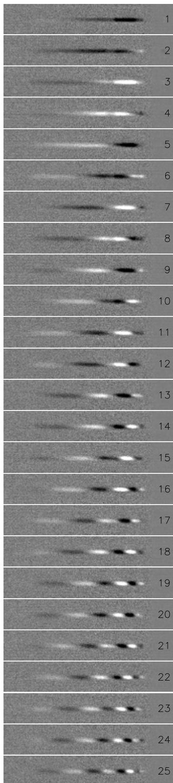
**Figure 3.3:** Fringe pattern on the detector during one fringe scan of HD 120404 at  $t = 17$  s (see figure 3.2). The interferometric signal is dispersed in horizontal direction. The scan consists of 25 individual steps of the piezo, *i.e.* it is different from the normal scan length of 40 steps. For increasing optical delay (here in total by  $52 \mu\text{m}$ ), more and more fringes appear in wavelength direction.
