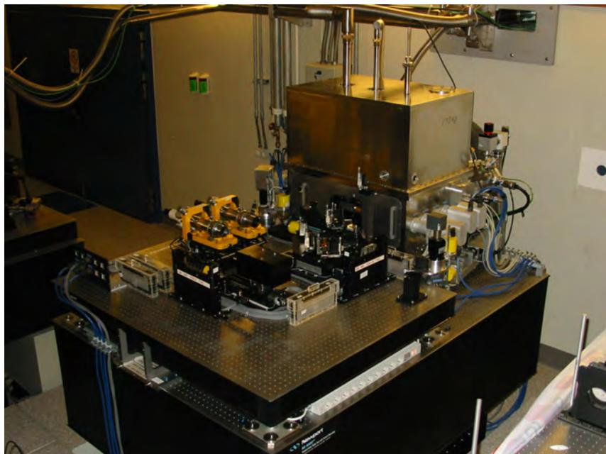
**Figure 2.9:** MIDI in the interferometric laboratory. Only the warm optical bench with the MIDI internal delay lines can be seen. The rest of the instrument is located inside the dewar at the far end of the optical table. (Image courtesy of ESO)
