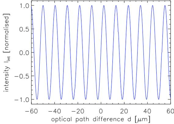
**Figure 2.2:** Intensity variation of the interferometric signal  $I_{\text{int}}$  with change of optical path difference  $d$  for a monochromatic source with a wavelength of  $\lambda = 10.5 \mu\text{m}$ . For  $d = 0.5\lambda, 1.5\lambda, \dots$  positive interference occurs, while for  $d = 0, \lambda, 2\lambda, \dots$  there is negative interference.
