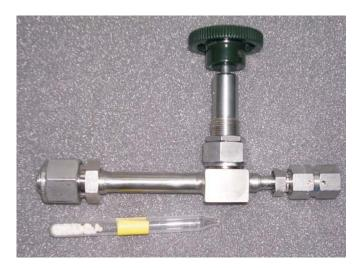
**Figure 3.25:** System for extraction of microwave treated glass vials. The vial can be inserted totally in the cracker system. Thus, contamination by leaking atmospheric air, as it is present in the case of an o-ring connection, can be prevented. The hand valve is used for moving of a plunger, which cracks the capillary and releases the gases from the vial. Below the cracker an opened sample is displayed.
