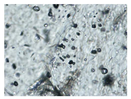
Figure 2.5: This section of a sample from the stalagmite H12 from Oman. The dark irregular shaped inclusions are assumed to be only air-filled. The light-reflecting, round or ellipsoidal inclusions are water-filled.
