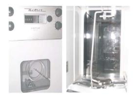
Figure 3.7: High precision balance (Mettler Toledo) with a precision of 2  $\mu$ g. The sample is put on the small roundish dish inside a chamber which is protected from air motion by sliding windows.
