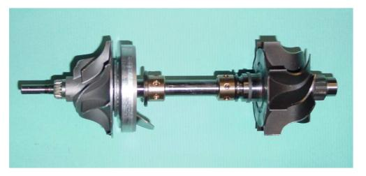
**Figure 1.1:** The rotor of a turbocharger consists of the shaft, the compressor (left) and the turbine wheel (right). The small brass rings are floating rings and mark the position of the bearings.
