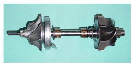
**Figure 6.2:** The rotor of a turbocharger used in the experiments at TCRDL. It consists of the shaft, the compressor (left) and the turbine wheel (right). The bearing positions are indicated here by the two floating rings (golden color). The experiments were done for plain journal bearings without floating rings.
