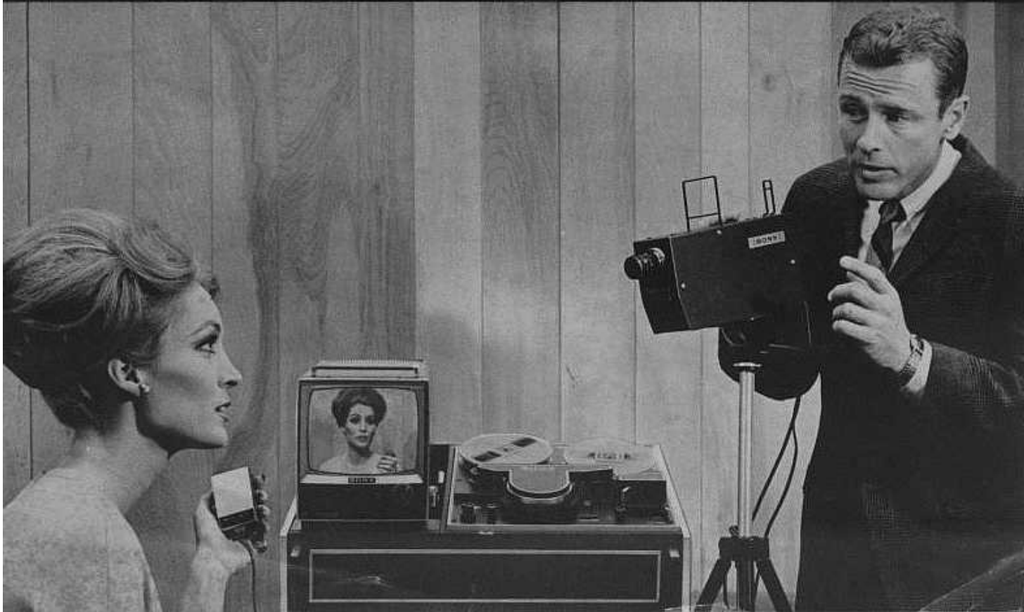
Sony VCK 2000, since 1965. A woman with microphone and a man with the video camera mounted on a tripod. Behind it: Recorder with magnetic tape and monitor. Photo: Sony.
