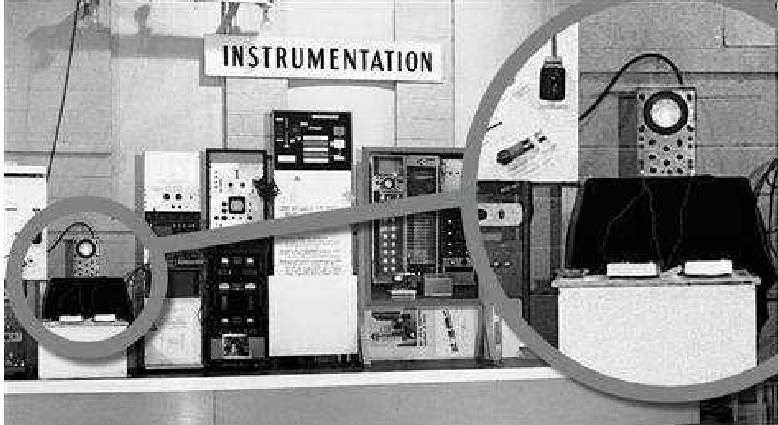
Higinbotham, William: Tennis for Two, 1958, Systron Donner Analog Computer, Germanium transistors, oscillograph (diameter: 5 inches), 2 boxes with turning knobs and press keys. Exhibited at the visitor's day of the Instrumentation Division at the Brookhaven National Laboratory, U.S. Department of Energy, Upton/Long Island ("Tennis for Two" is presented enlarged in the wider circle. Image source: Brookhaven National Laboratory).
